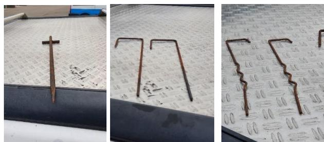
Figure 2: T-peg hering (left) and pins (middle and right) that were used for the installation of the temporary protection.
