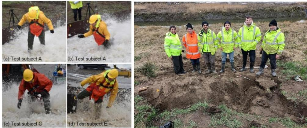
Figure 3. Left: Students of TU Delft volunteering as subjects in overtopping experiment in which overtopping discharges that a human can withstand were measured. Right: Johannes Idsinga, student of TU Delft participating in a concrete grout excavation activity in the living lab to collect data for his minor thesis.
