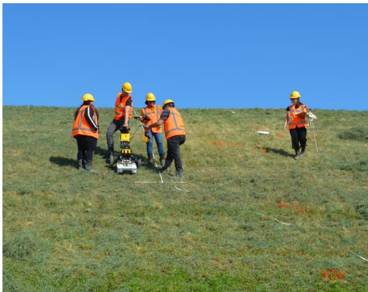
Figure 4: Hoang Dung Nguyens, PhD student of Lille University, performing a GPR scan in the living lab with the support of students from HZ and TU Delft.
