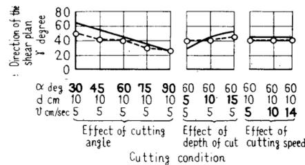
As it can be observed the shear angle varies with the cutting angle, the table below summarizes the cutting conditions observed withing this experiment, moreover in chapter 4 an analysis has been conducted underlying the dependency of the strengthening factor to the shear angle.
