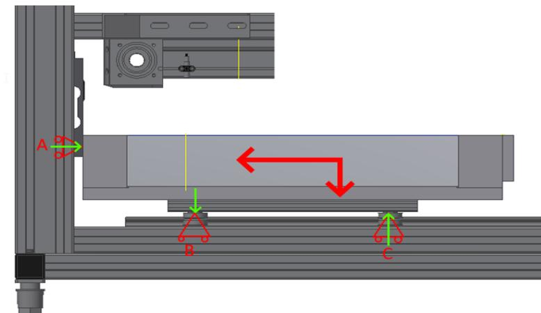
To counteract this problem two solutions have been thought, the first consist in purchasing a multi-axis load cell that would measure both the vertical and horizontal forces, this solution is however not feasible from an economic point of view. For this reason a second concept have been thought, the horizontal and vertical forces are going to be measured in different moments, this is allowed by replacing the load cells with two dummy aluminum blocks.
