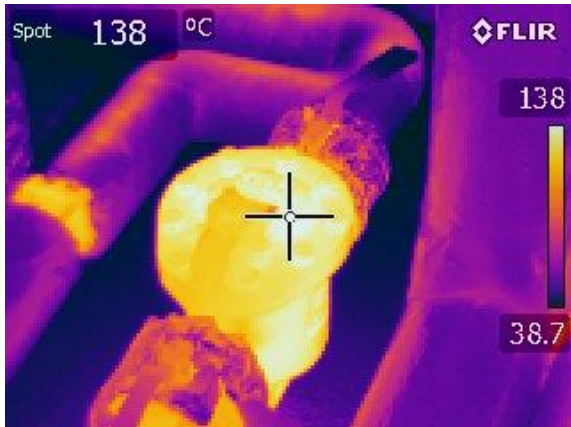
Figure 19: Temperature of the steam trap
