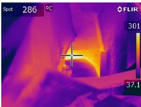
Figure 21: Hotspot near turbocharger
