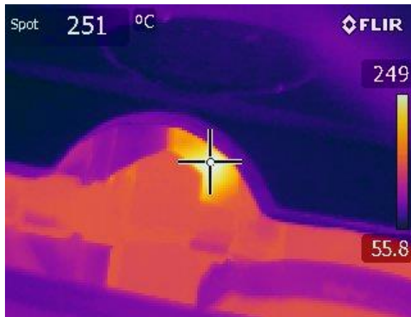
Figure 25: Hotspot between cylinders
