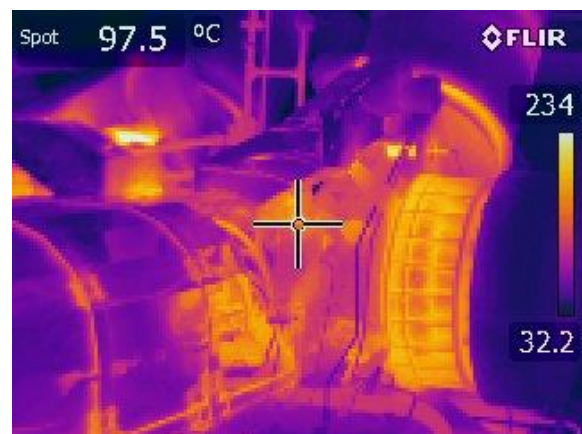
Figure 22: Hotspot near turbochargers
