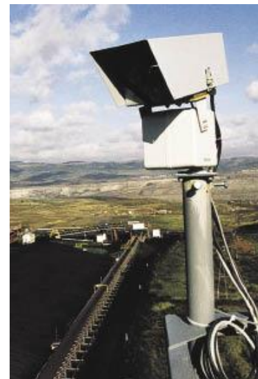
Figure 10: Thermal imaging camera mounted on the steel mast (FLIR, 2015)
