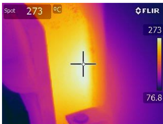
Figure 23: Hotspot near the hatch cover
