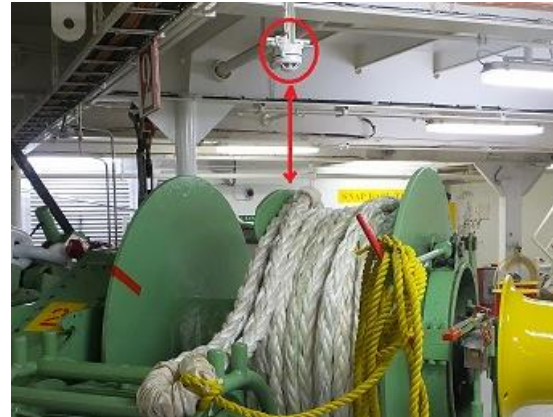
Figure 28: Position of the heat detectors to the mooring winches
