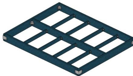
The frame's shape is reinforced by the use of corner plates on the inside and backer plates on the outside. These maintain the rigidity of the frame.
