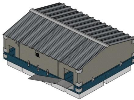
The next step would be to install the access ramp/gangway and the roof. The ramp is braced by triangular support brackets connected to the joist header. The roof sections may be simply nailed to the walls before attaching the ridge cap on the top, which prevents leaking.
