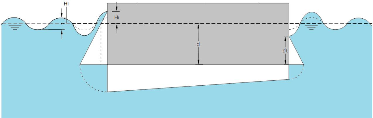
Figure 19: horizontal pressure gradient formed by incident waves
