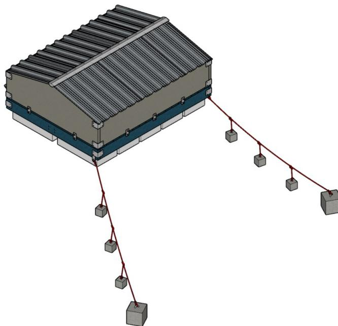
At this point, the structure may be put on the water and floated into position before securing the weighted ropes to the back of the structure such that the openings point downstream.
