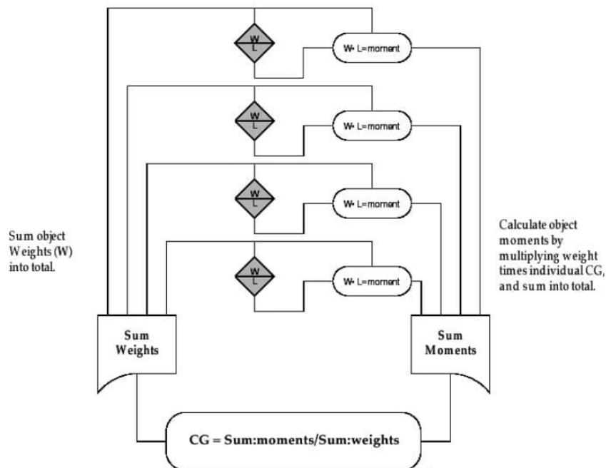
To facilitate the metacentric height calculations, the centres of gravity are determined on a case-by-case basis, in addition to the composite centre of gravity. The different cases are as follows:
