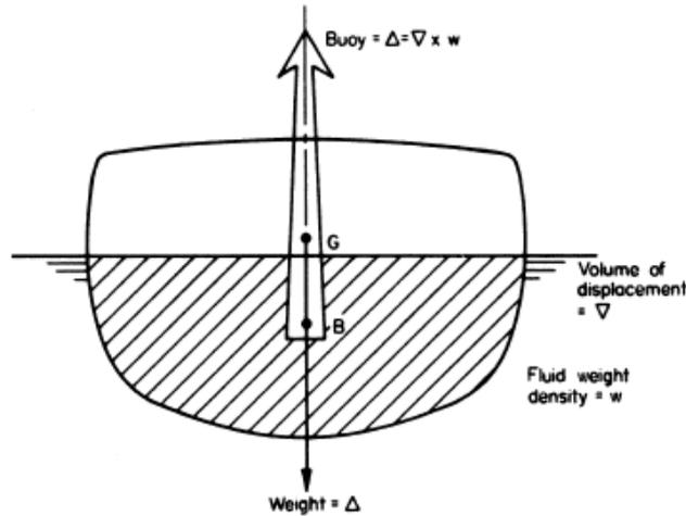
Figure 13: overview of hydrostatic points
