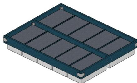
Next, the expanded polystyrene floats will be placed into the equally sized compartments between the bottom joists. Following from this, the entire frame should be lifted and placed on supports to allow the installation of the top joists.
