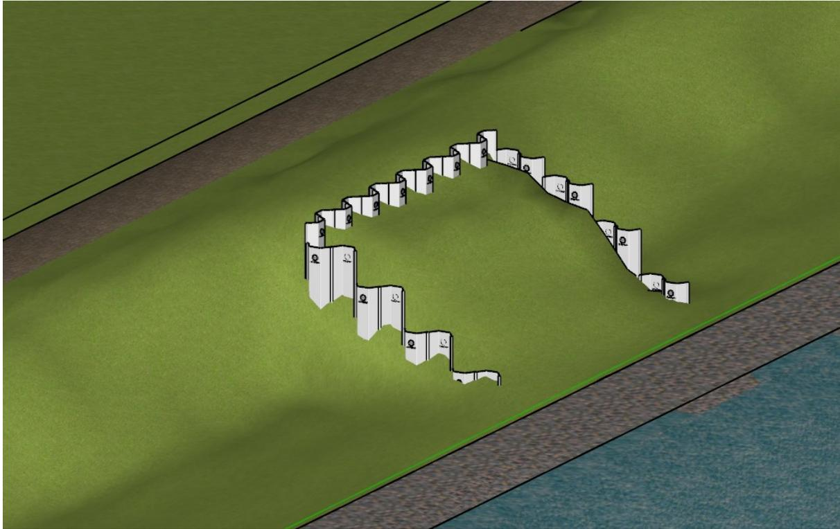
*Figure 10: use of sheet pile compartment placed against dyke*
