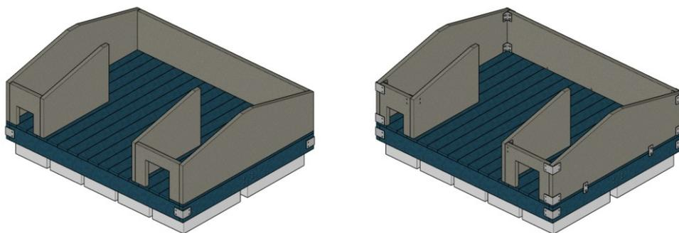
The walls of the superstructure can then be erected and secured in place using the same corner and backer plates as were used for the base platform. The connection between the platform and the walls will be facilitated by overlapping fishplates, two on each of the shorter sides and three on the longer back panel.
