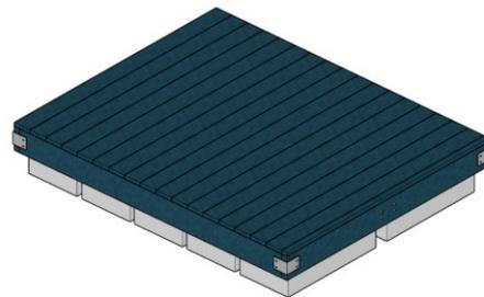
Finally, to complete the construction of the platform, the deck boards will be screwed to the outer joist headers and to the inner top joists. The screw holes should be marked or drilled beforehand to ensure accuracy.
