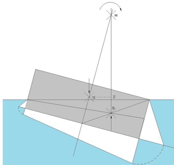
Figure 16: acting moment and pressure differential
