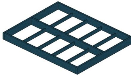
The frame or base is first constructed after ensuring all the boards are of the correct length. The joist headers are the outermost boards and are therefore laid down first, using the equally spaced bottom joists to maintain correct spacing before securing the bolts in place. Lock washers should also be used to keep the bolts and nuts from loosening.
