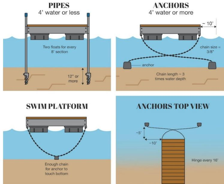
Figure 11: floating dock anchorage systems
