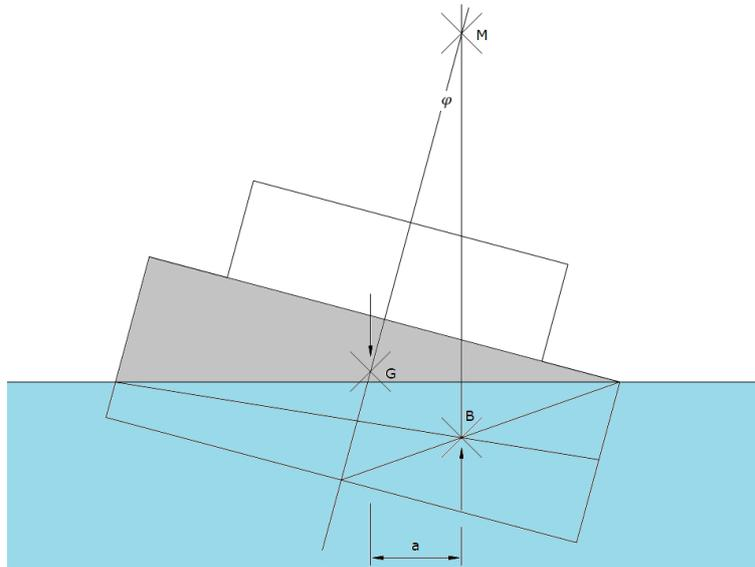
Figure 17: intersection of centreline and buoyant line of action
