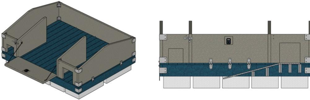
The maintenance wall may then be installed. The hinges and chains are first secured before fastening the panel to these points. The chains limit the rotation of the wall outwards in order to keep the hinges intact. A sliding latch lock is used to hold the wall in place. A point of attention is that the monitoring camera window may be installed prior to this step.
