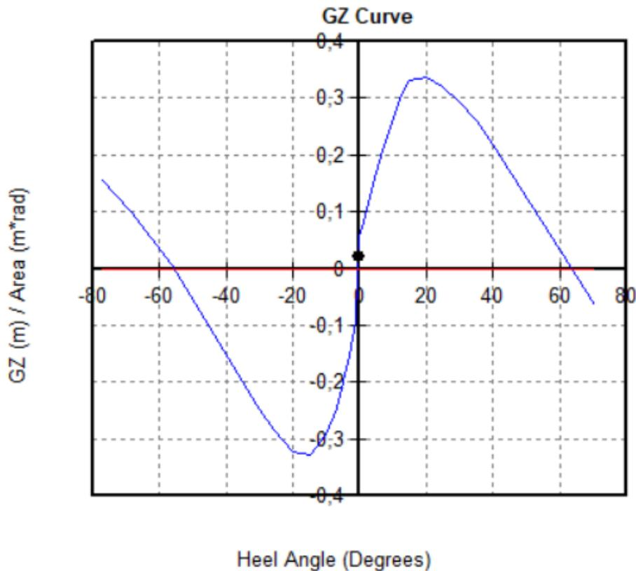
Figure 27: relationship between righting arm and heel angle for finalised floating HVP design
