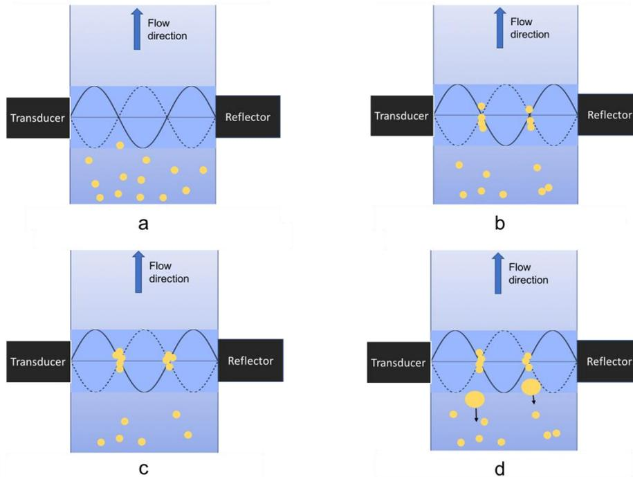
**Figure 1** Diagram illustrating the particle separation process using Ultrasound waves. Yellow circles represent the suspended particles in the fluid. (a) standing wave created by transducer and reflector (b) particles become trapped by acoustic forces at the nodes (c) particles stick together forming agglomerations (d) Agglomerations sediment.
