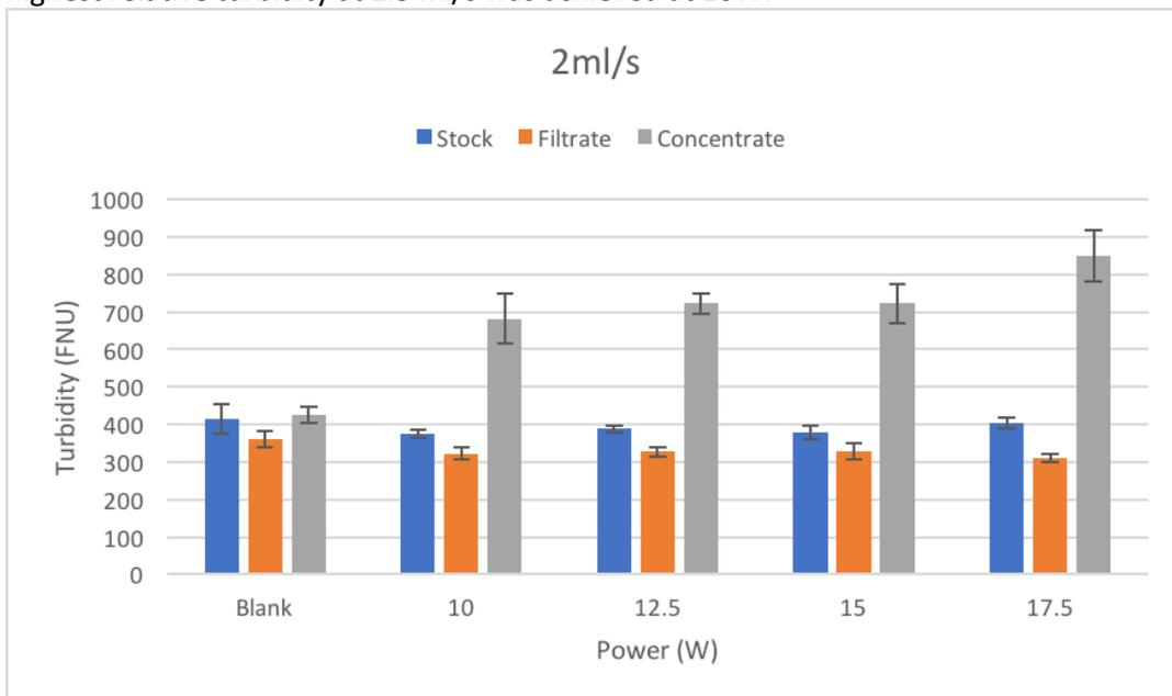
Figure 12 The effect of ultrasound on the turbidity of the filtrate and concentrate compared to that of the stock at varying power outputs at a flow of 2 ml/s.
