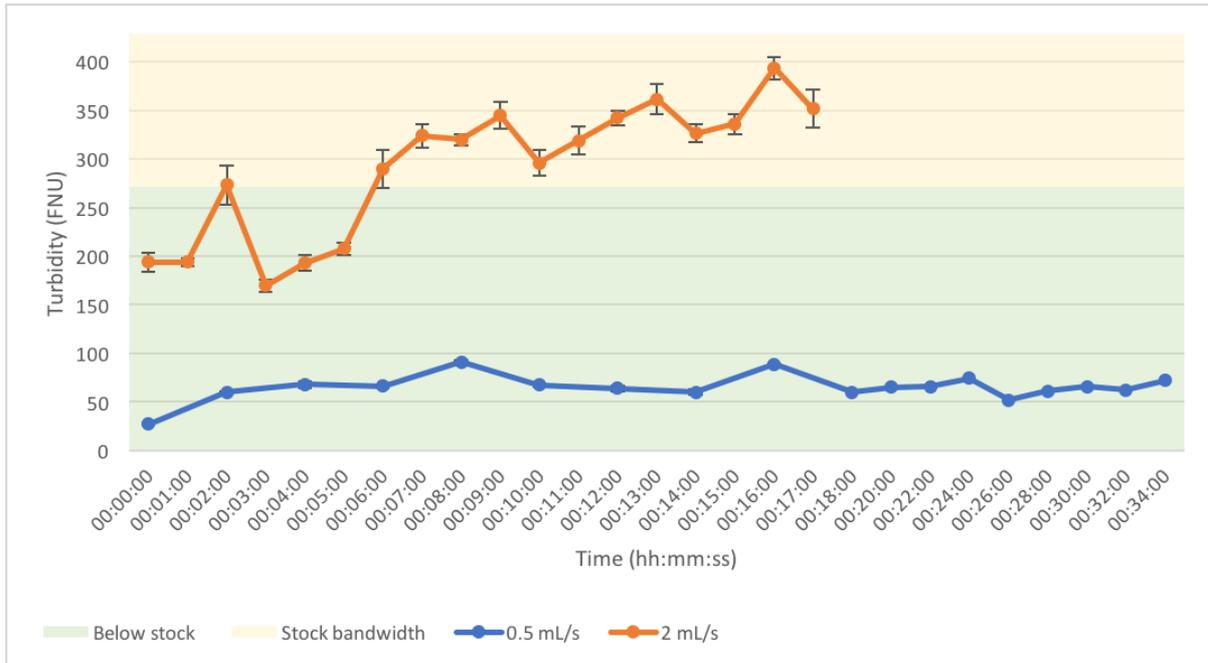
Figure 8 The turbidity of the filtrate through time when ultrasound is off. Turbidity is shown for two flow rates, 0.5 ml/s with 2 minute intervals between measurements and 2 ml/s 1 minute intervals between measurements. The bandwidth of the stock turbidity is shown in orange, and green represents the range of turbidities below that of the stock. Error bars show the Standard error ( $\sigma/\sqrt{n}$ ).
