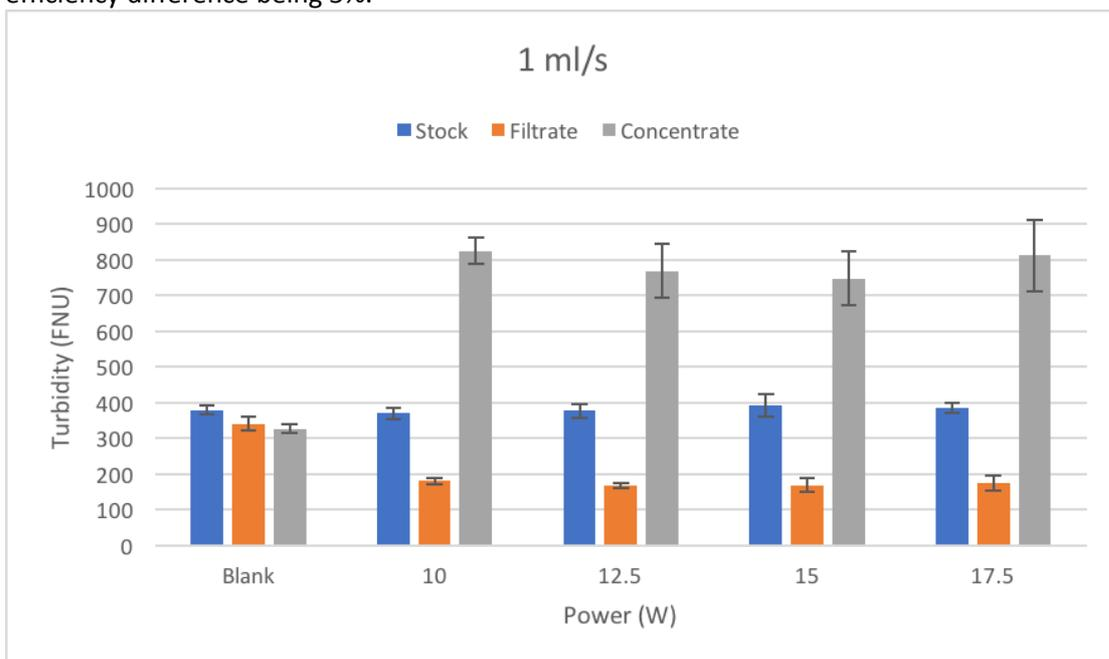
Figure 10 The effect of ultrasound on the turbidity of the filtrate and concentrate compared to that of the stock at varying power outputs at a flow of 1 ml/s.
