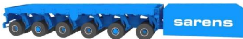
Figure 22 - Example of SPMT (Kamag 2400 ST) (Sarens Equipment data - Transport, 2022)
