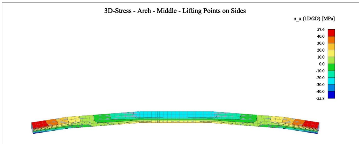
Figure 28 - 3D-Stress in Middle Arch Sections - Lifting points on the sides
