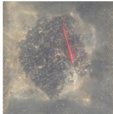
FIGURE 5, EXAMPLE OF A PHOTOGRAPH THAT WAS TAKEN AFTER PLACING THE MUSSELS IN THE CORRESPONDING GABION. THE SCREW WRAPPED IN RED TAPE IS A REFERENCE POINT FOR LATER ANALYSIS.
