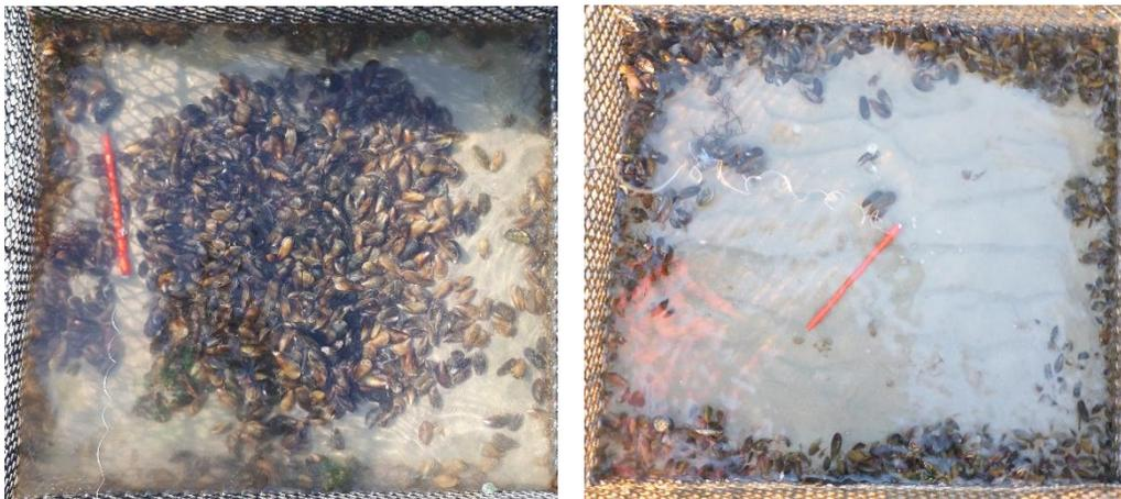
**FIGURE 21, MUSSELS WITHIN THE SAM GABION, THE PICURE LEFT IS AT THE START OF EXPERIMENT FM18 (21-02-2018) THE RIGHT PICTURE IS TAKEN 7 DAYS LATER (28-02-2018) ALMOST ALL THE MUSSELS ARE FORCED TO THE SIDE OF THE GABION.**
