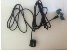
Figure 4. 15 Ultrasonic sensor JSN-SR04T
