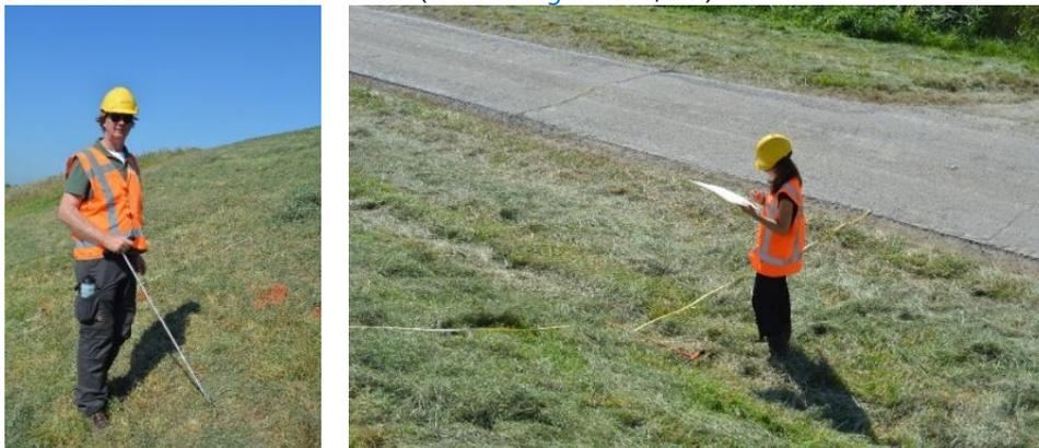
Figure 4.39. Left: Detection of burrows with a probe; Right: Paper mapping of burrows
