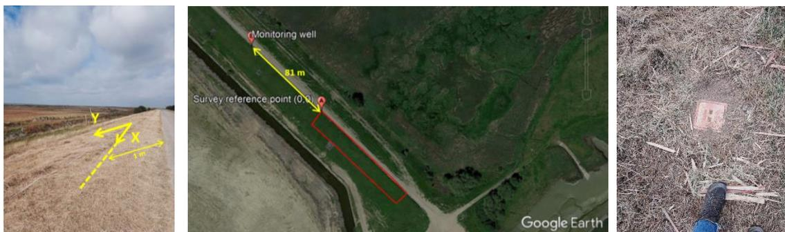
Figure 5.58. Left and middle: Position of reference point in relation to asphalt road and fixed point on the levee. Right: Fixed point 81 m NW of the reference point.
