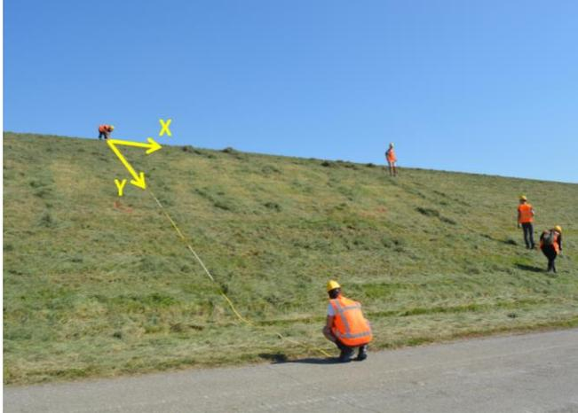
Figure 4.40. X- and Y-axes for recording distance of burrows from reference points.
