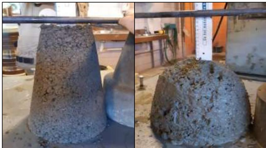
Figure 18. Slump tests of Mix A and Mix B
