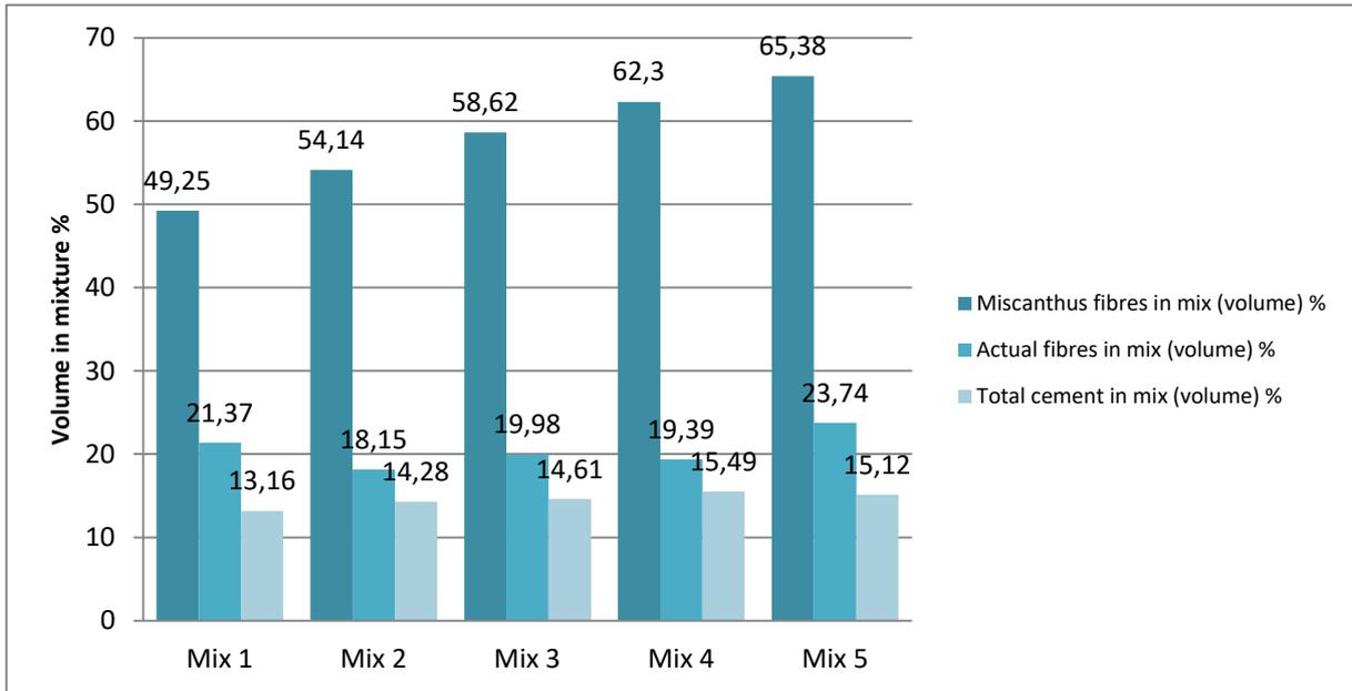
Figure 17. Miscanthus fibre and cement content in bio-concrete mixtures 1 to 5
