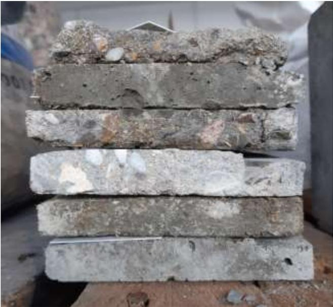
Figure 23. Samples intended for thermal conductivity test
