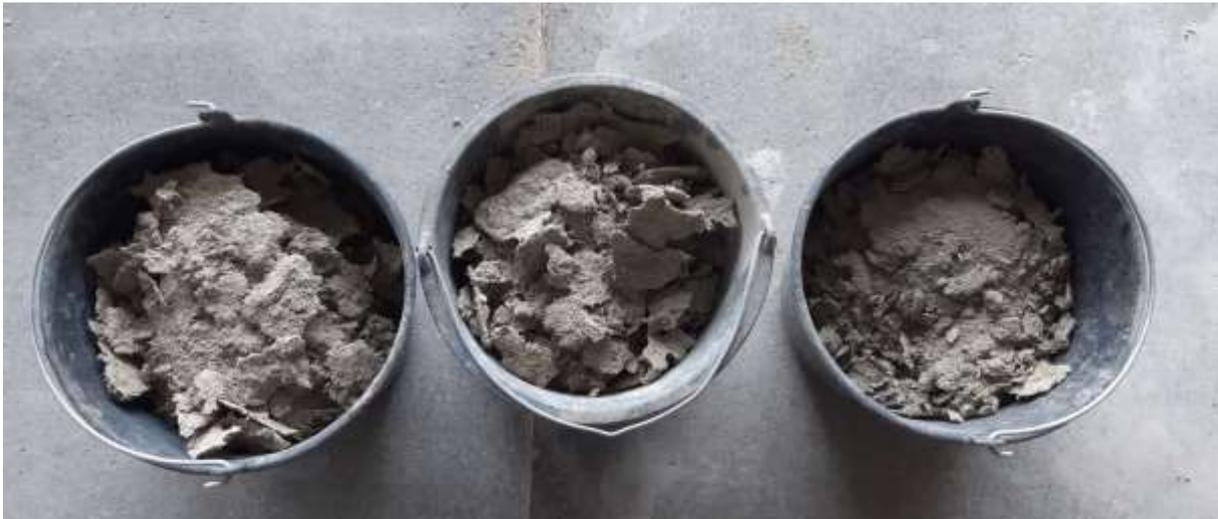
Figure 11. Dried and scraped samples of pre-treated *Miscanthus* fibres, before crushing (preliminary test)
