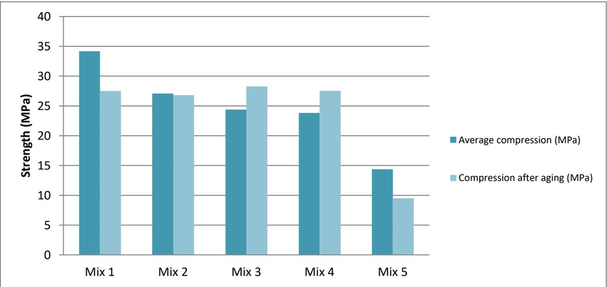
Figure 28. Comparison of compressive strength
