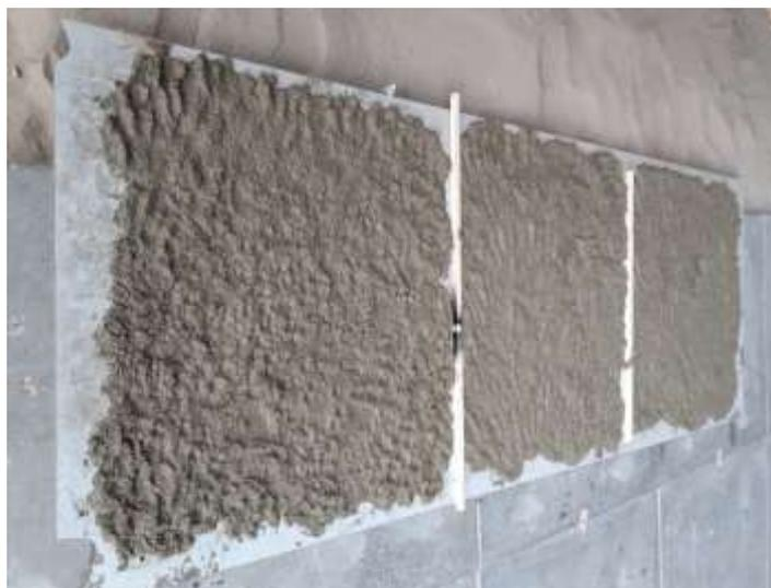
Figure 10. Fresh samples of pre-treated *Miscanthus* fibres (preliminary test)
