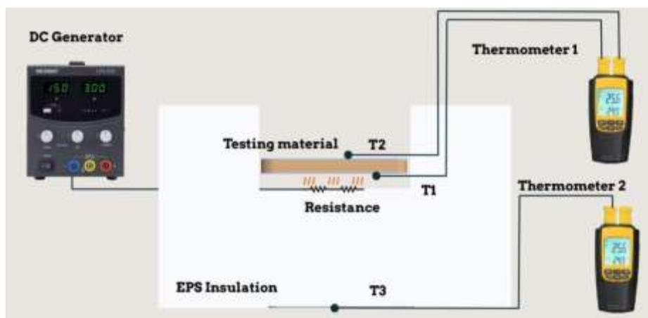
Figure 13. Process Flow Diagram (PFD) of thermal conductivity test at UCR
