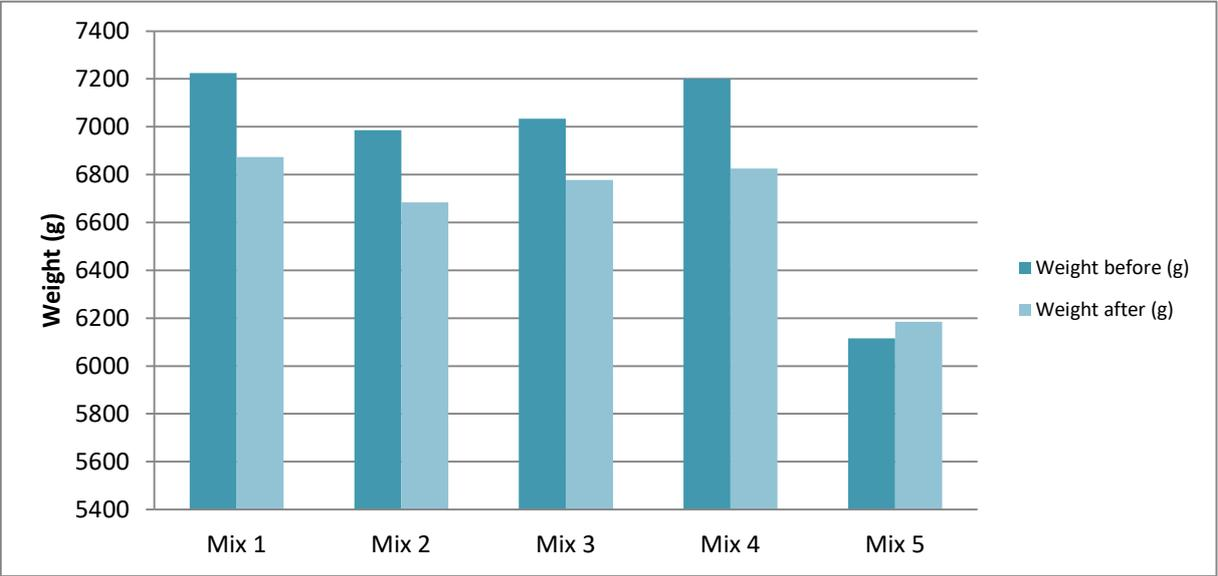
Figure 27. Weight of cubes before and after accelerated weathering/aging process
