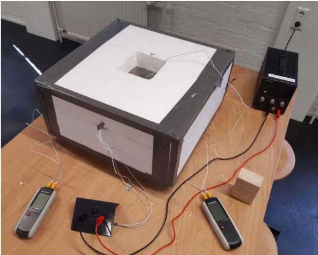
Figure 14. Thermal conductivity testing equipment at UCR laboratory
