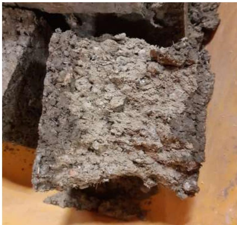
Figure 19. Failed cube Mixture A
