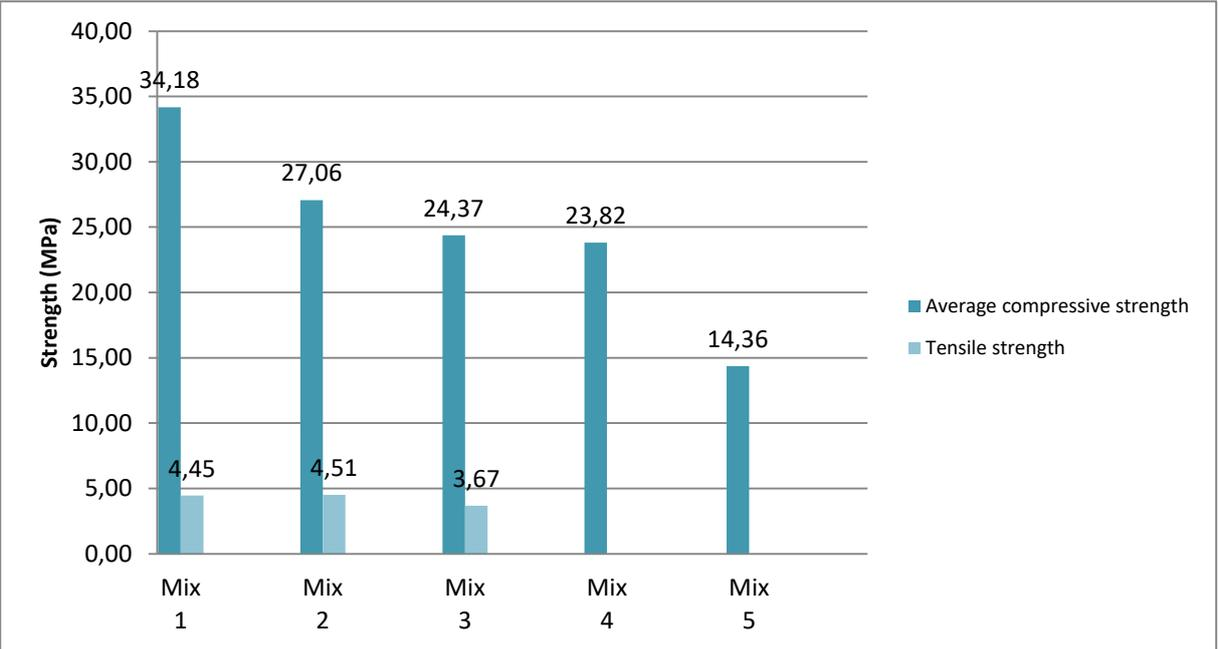
Figure 20. Compressive and tensile strength of bio-concrete mixtures
