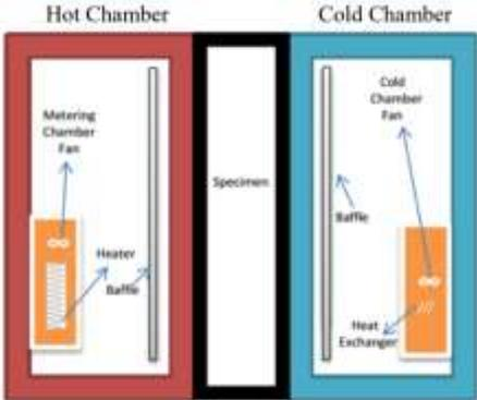
Figure 6. Steady state boxes method (Asadi et al., 2018)
