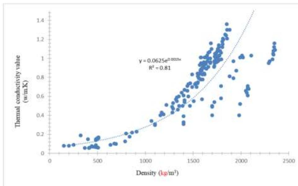
Figure 5. Relation between thermal conductivity and density of materials (Asadi et al., 2018)
