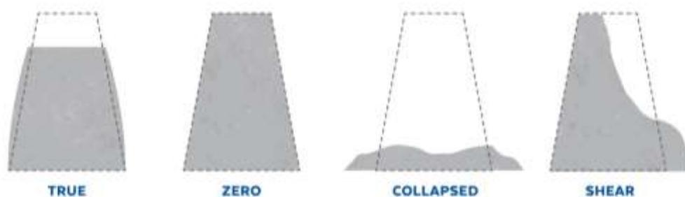
Figure 12. Different types of slump
