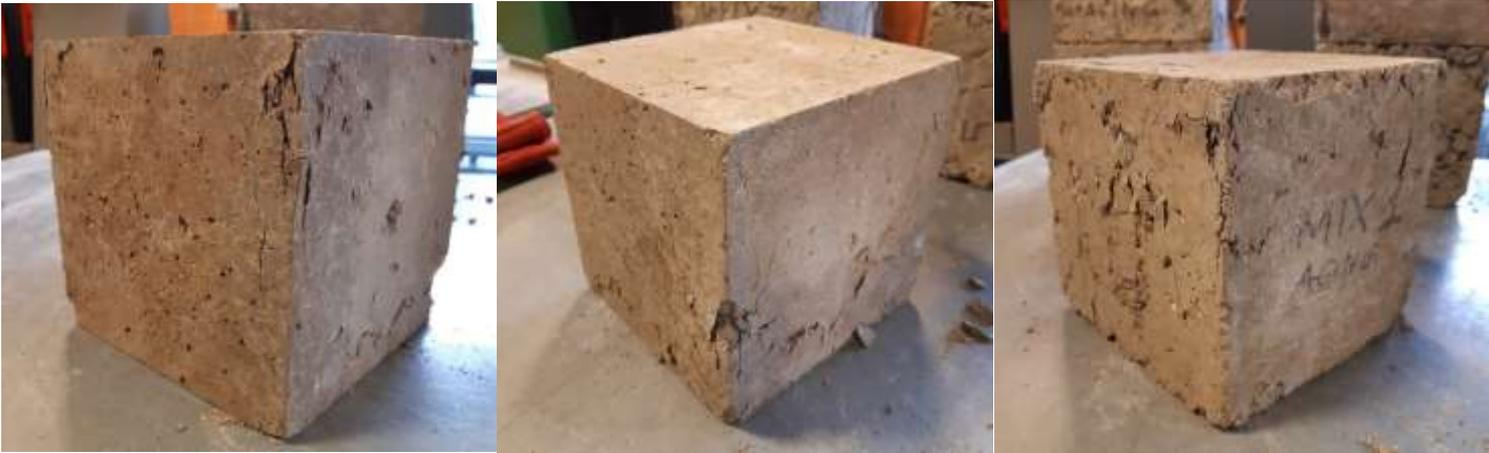
Figure 29. Example of cracks on three different aged cubes after the compressive strength test
