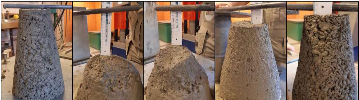
Figure 16. Slump tests (left to right): mix 1, mix 2, mix 3, mix 4 and mix 5
