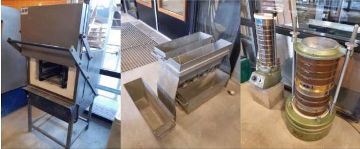
Figure 9. Machines used for sieve analysis at Scalda: oven, quarter sieve, fine sieve (for sand) and coarse sieve (for gravel)
