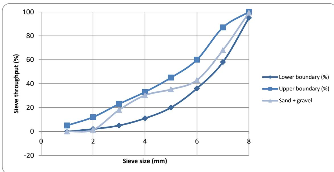
Figure 15. Grain size distribution of sand and gravel delivered by De Hoop
