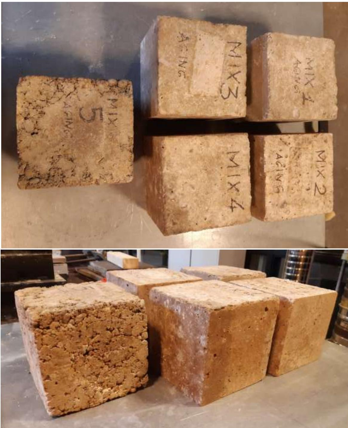
Figure 26. Bio-concrete cubes after accelerated weathering/aging process
