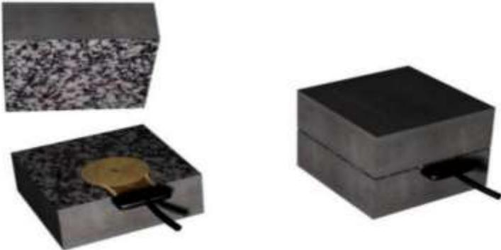
Figure 8. Transient plane source method (Asadi et al., 2018)
