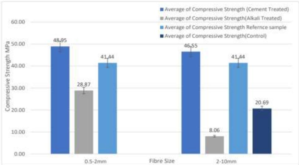
Figure 2. „Compressive strength of tested samples” (Adebisi, 2021)
