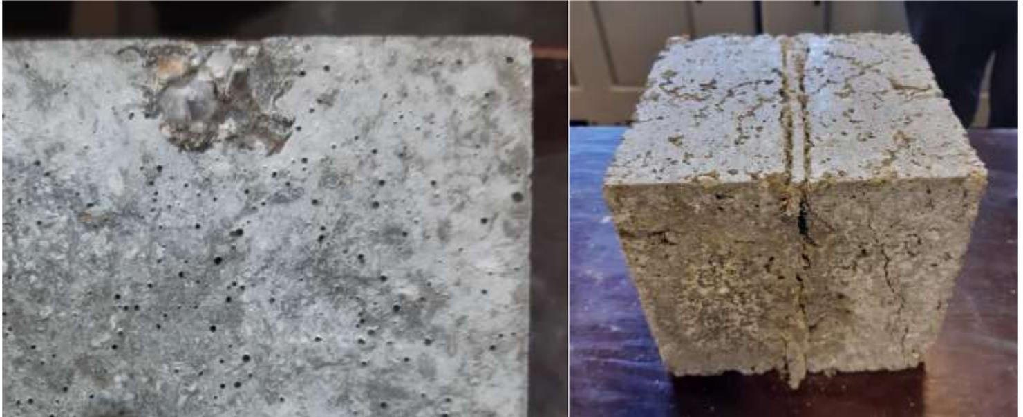
Figure 21. Close-up damage Mix 2 and split tensile tested cube Mix 5
