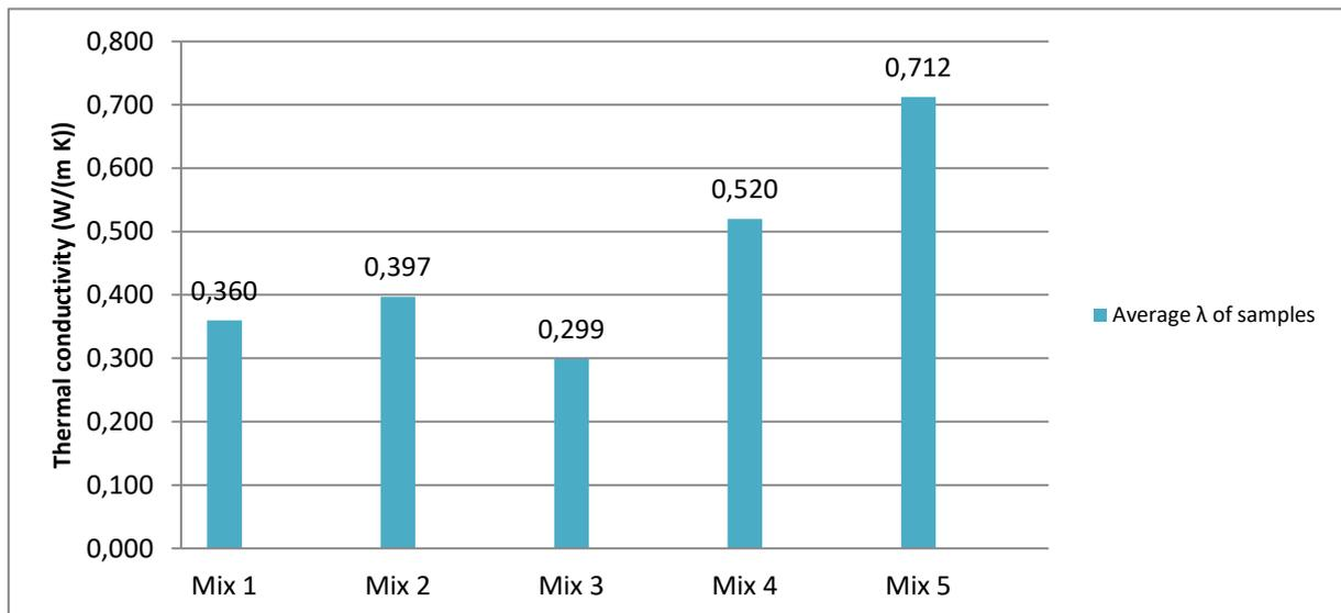
Figure 22. Thermal conductivity test results mix 1 to 5
