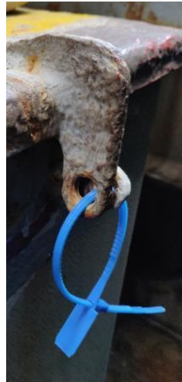
Figure 22 Booby hatch cover sealed
