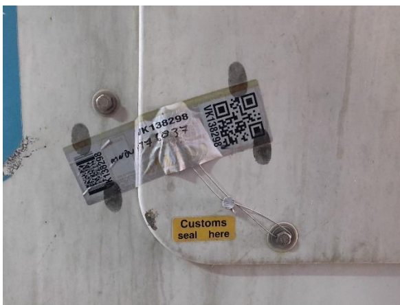
Figure 20 Reefer container motor unit seal
