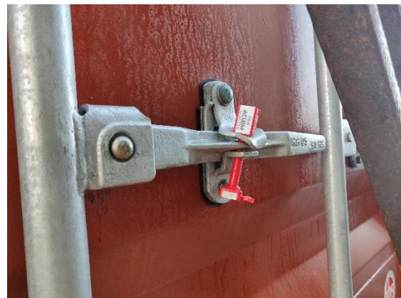
Figure 19 Locking bar on the door
