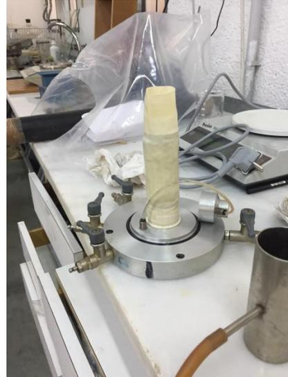
Figure 17 Triaxial Test equipment
