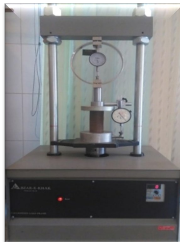
Figure 18 UCS test device in the laboratory
