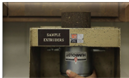
Figure 9 Removal of the compacted sample with an extruder
