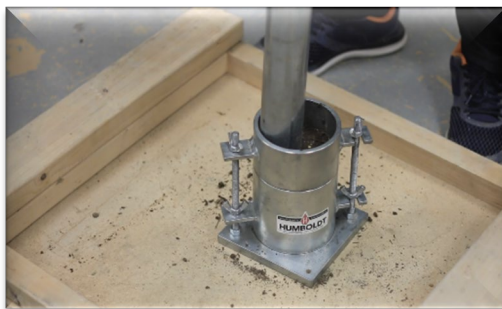
Figure 8 proctor test/ compaction test
