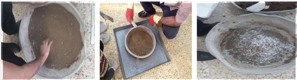
Figure 7 Mixing of fibers with clayey soil
