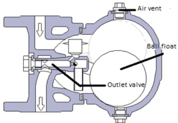
Figure 6 Ball float trap – retrieved from (Condenspot.nl, 2015)
