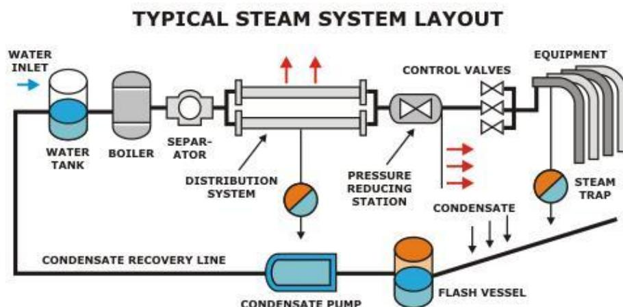
Figure 2 Schematic view of the steam systems principle - retrieved from (Wadeindustrial, 2011)
