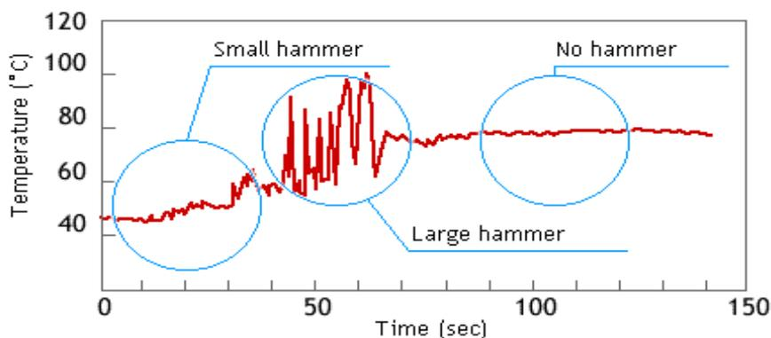
Figure 3 Water hammer at different condensate temperatures - retrieved from (TLV, Steam Theory, waterhammer, 2016)
