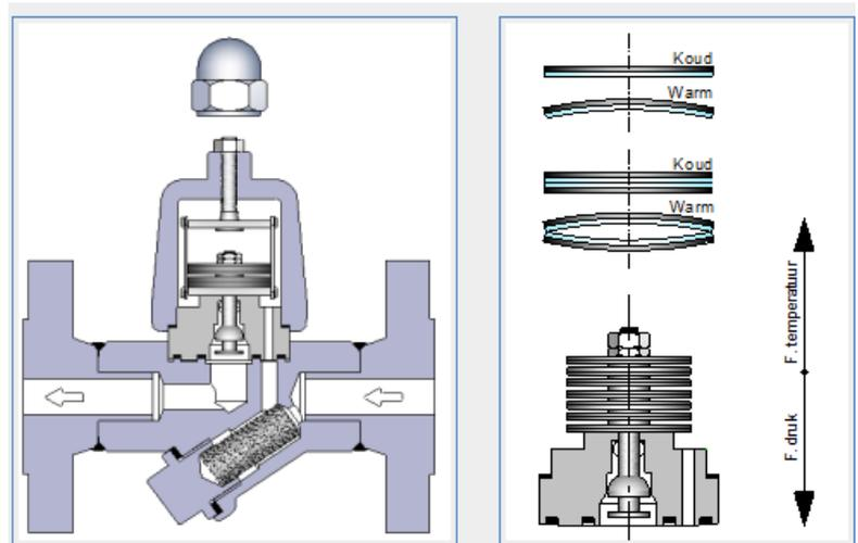
Figure 8 Bimetal steam trap – retrieved from (Condenspot.nl, 2015)
