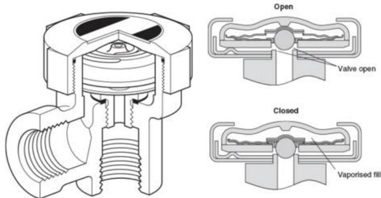
Figure 10 Membrane steam trap - retrieved from (Condenspot.nl, 2015)
