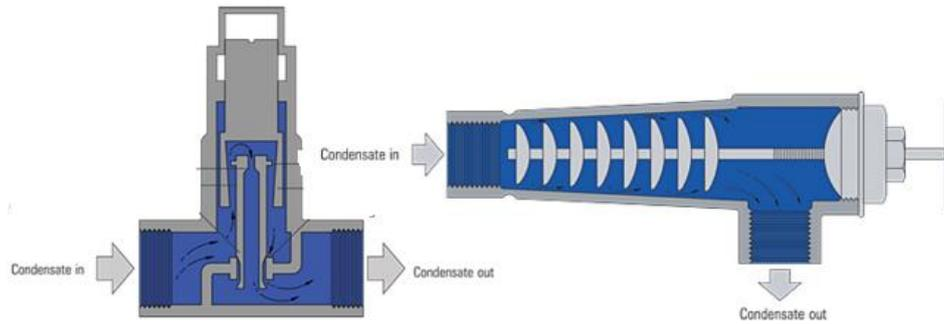
Figure 12 Impulse and labyrinth steam traps - retrieved from *(Thermodynamic Steam traps, Spirax Sanco, 2015)*
