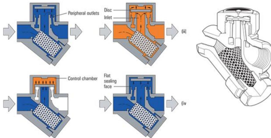
Figure 11 Thermodynamic steam trap - retrieved from (Thermodynamic Steam traps, Spirax Sanco, 2015)
