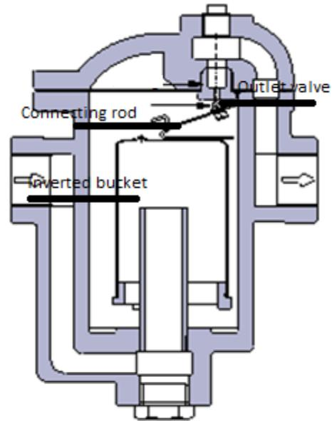
Figure 7 inverted bucket trap - retrieved from (Condenspot.nl, 2015)
