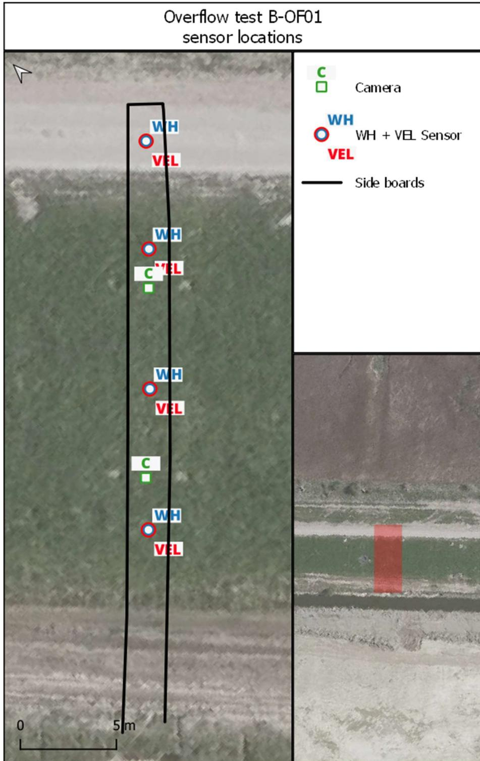
Figure 5 - Sensor locations on B-OF01.
