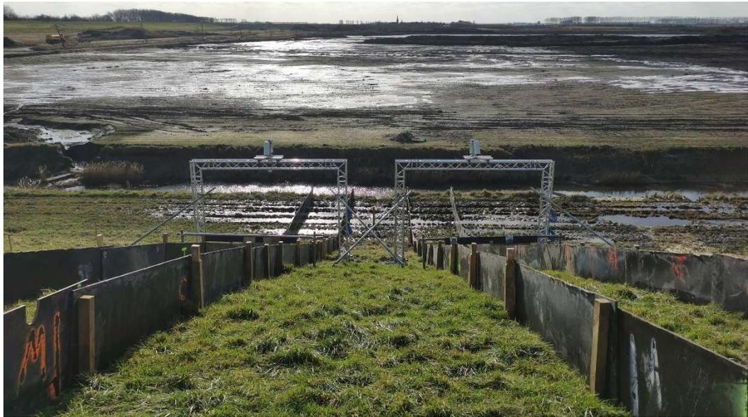
Figure 52 - The two parallel test sections for the Levee Challenge.
