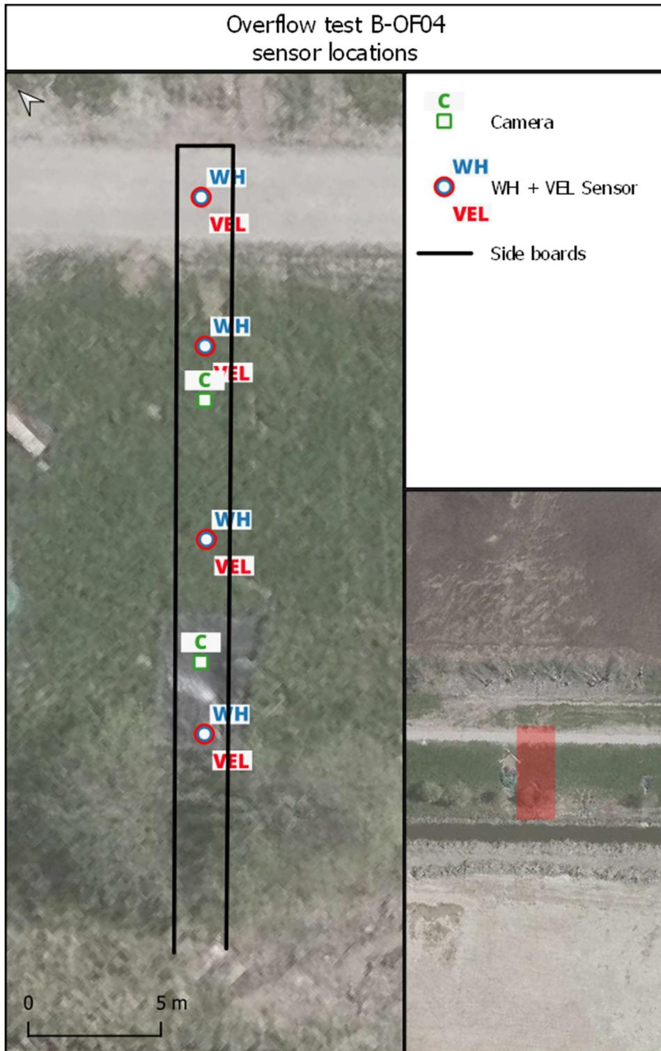
Figure 27 – Approximate sensor locations at B-OF04 (no GPS measurement at this test site).
