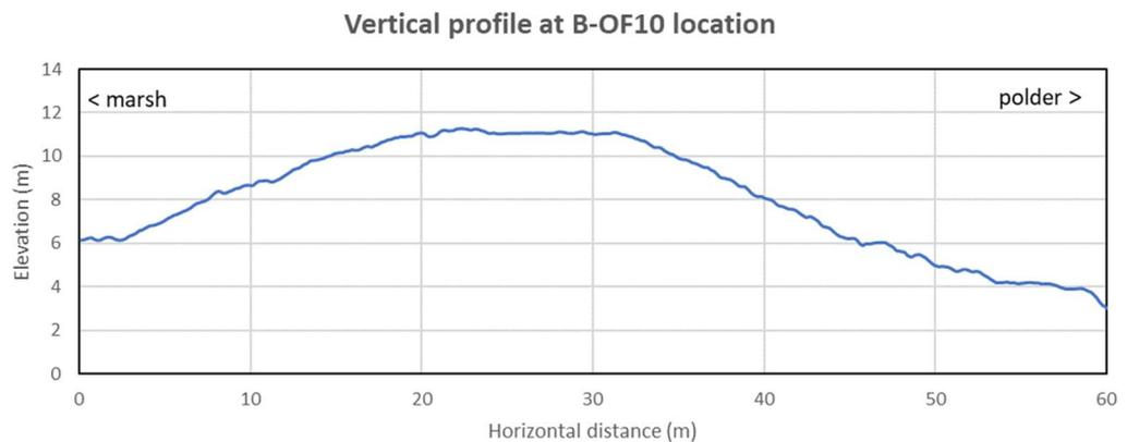
Figure 70 - Vertical profile at the B-OF10 site.
