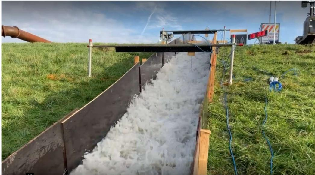
Figure 23 - General view on test section B-OF03. Notice the narrowed section width.
