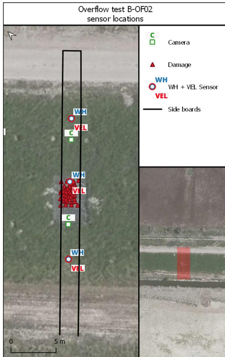
Figure 13 - Location map of overflow test B-OF02.
