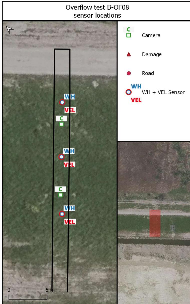
Figure 57 - Positioning of the sensors at the B-OF08 position.
