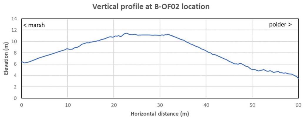
Figure 12 - Vertical profile of the B-OF02 overflow test section.
