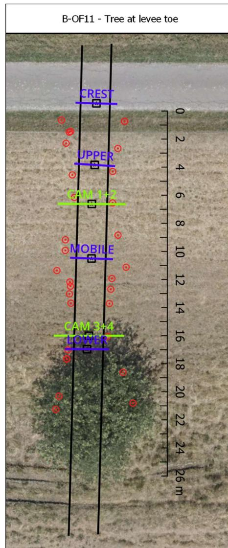
Figure 77 - Sensor locations on B-OF11 test section.
