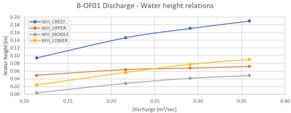
Figure 11 - Discharge - Water height relations for B-OF01 based on block B2.
