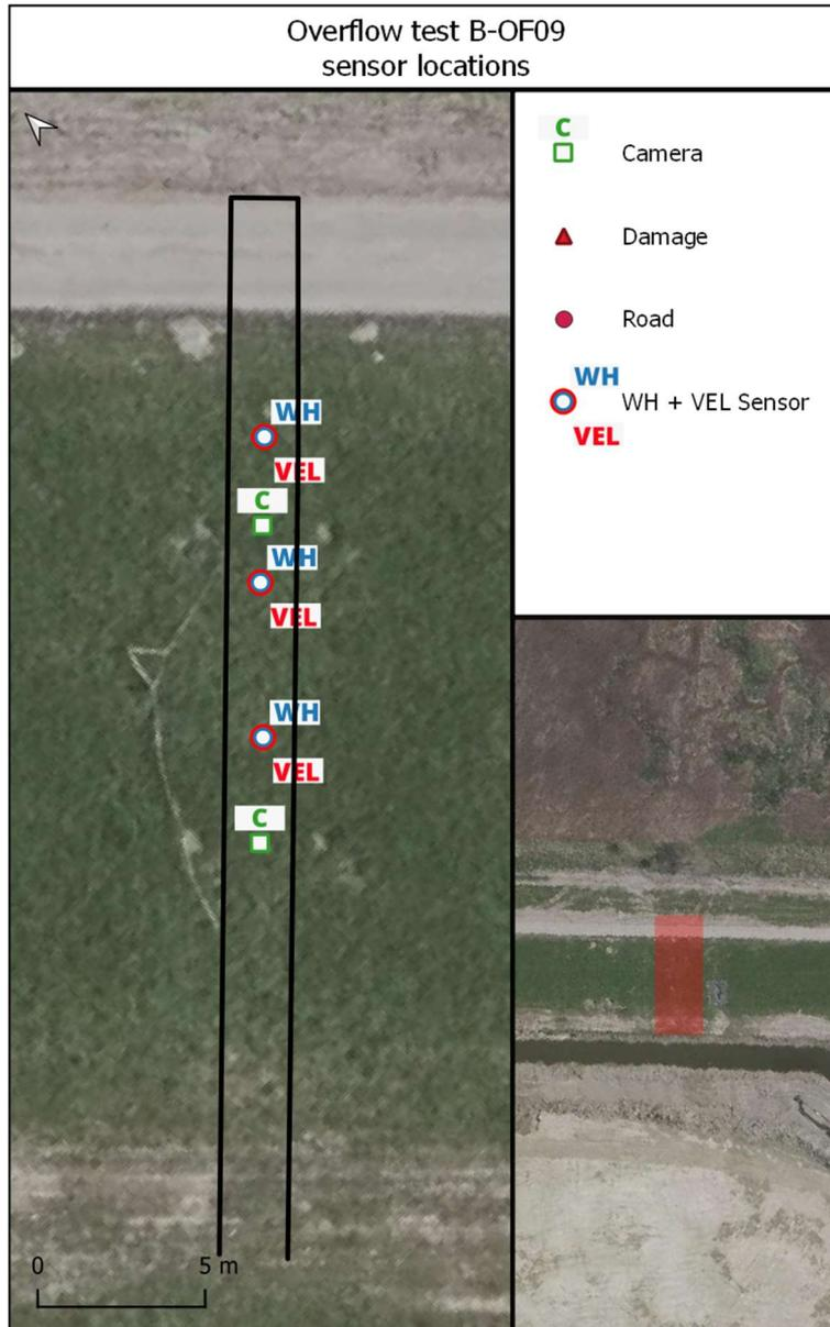
Figure 64 - Positioning of the sensors at the B-OF09 position.
