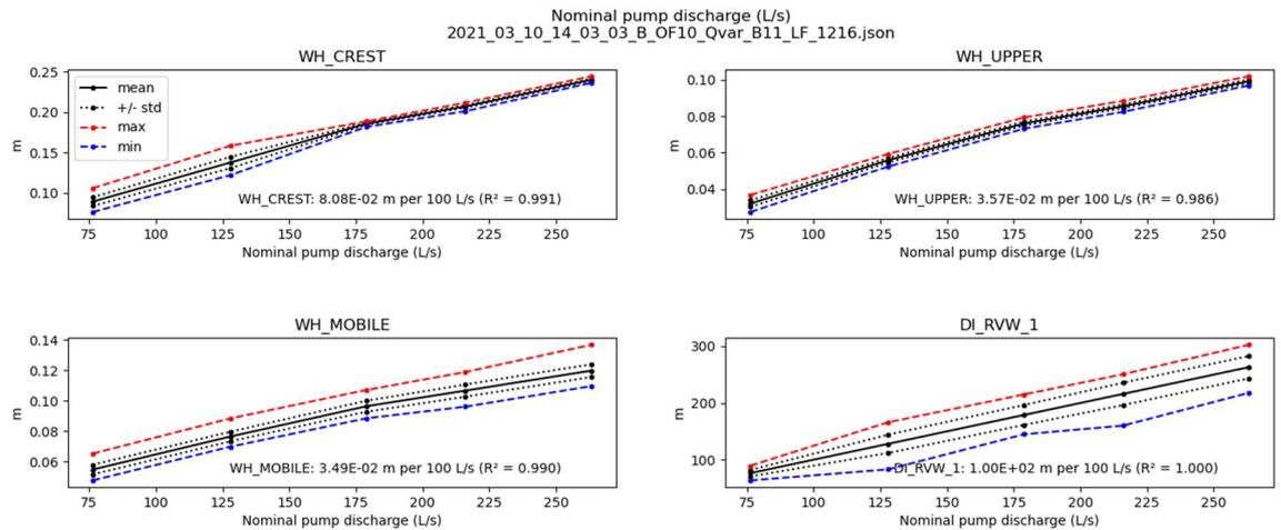
Figure 74 - Relations between timeseries (Water height at CREST, UPPER (= Upper slope) and MOBILE (= middle slope) and measured discharge (DI\_RVW\_1) in function of nominal discharge (= as per frequency regulator).
