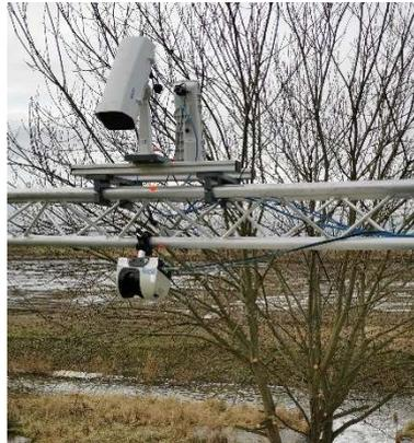
Figure 88 - Overhead cameras and 2D Line scanner mounted on the lower portal.
