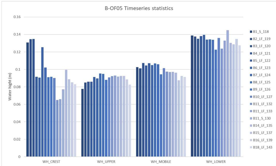
Figure 43 - Water height timeseries statistics per sensor and block.
