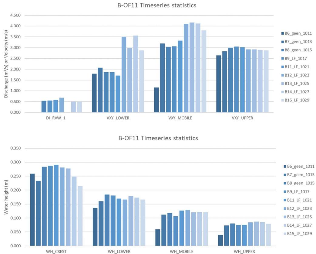
Figure 87 - Mean hydraulic parameters per test block.
