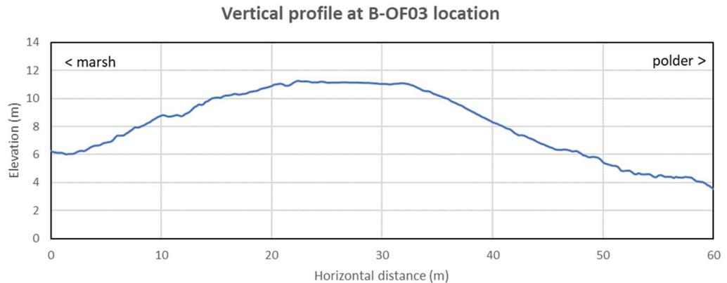
Figure 21 - Elevation profile over the B-OF03 High Discharge site. Data from drone based photogrammetry survey.
