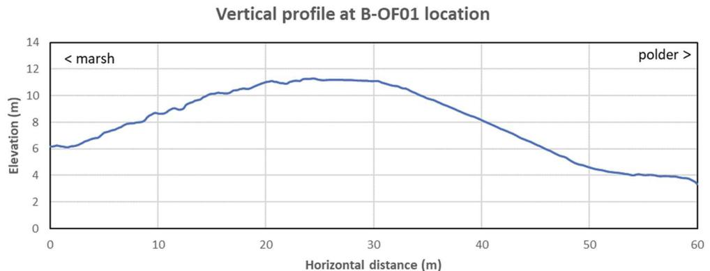
Figure 3 - Elevation profile over the levee at test site B-OF01.
