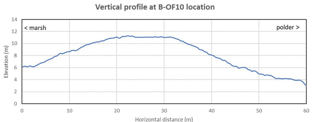
Figure 47 - Vertical profile at the B-OF10 site.
