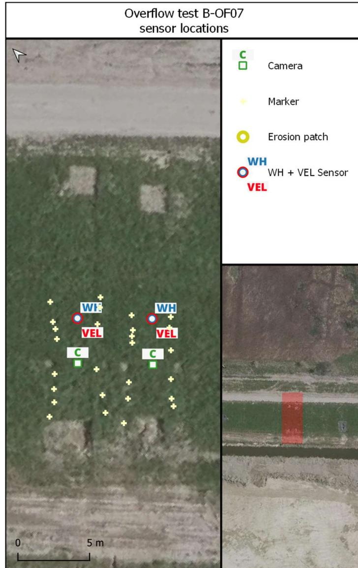
Figure 54: Sensor locations on B-OF07.
