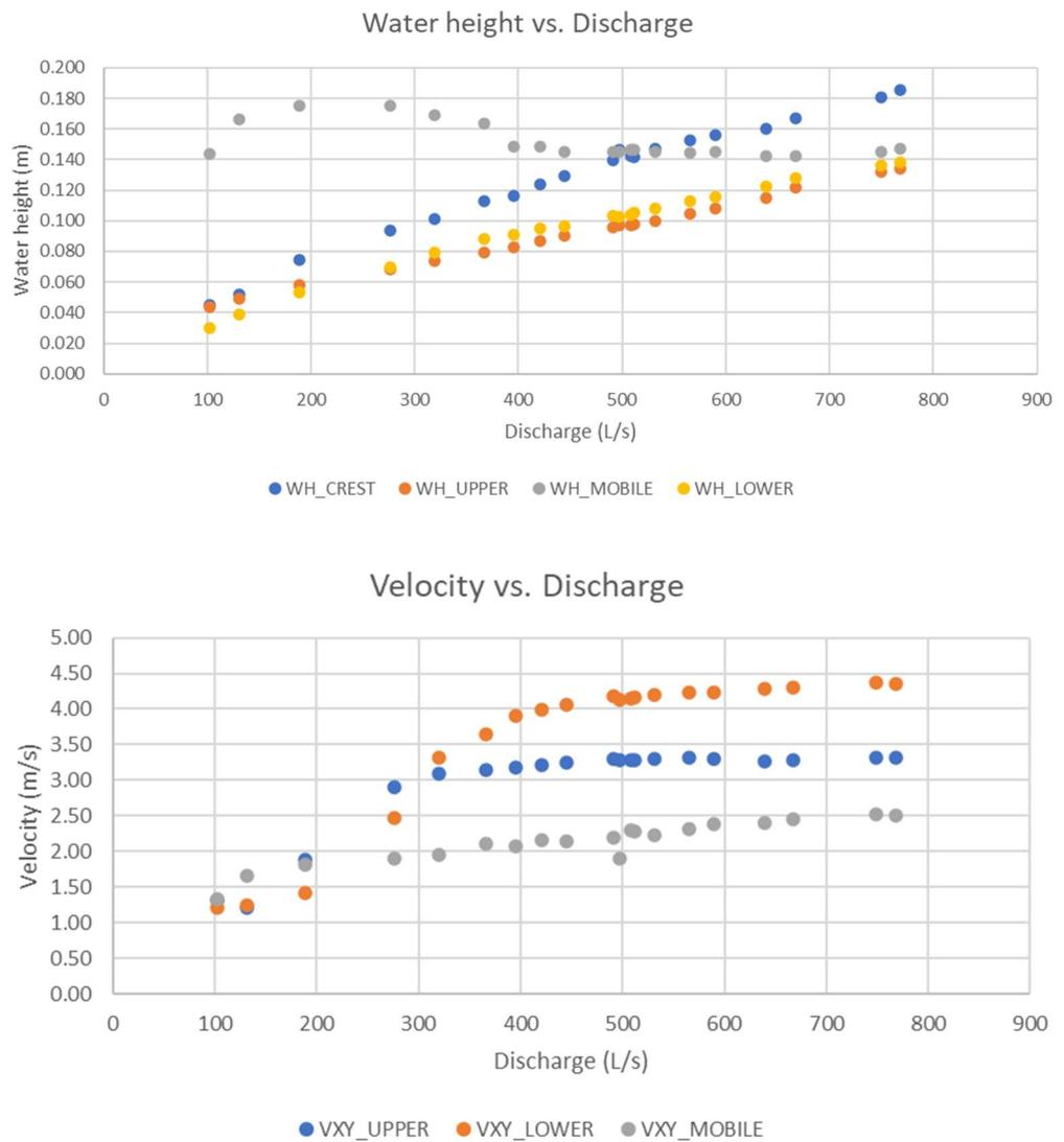
Figure 62 - Average water heights (upper) and velocities (lower) vs. discharge.
