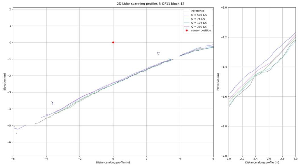
Figure 89 - 2D LiDAR scan of the ground and water surface at different discharge conditions.
