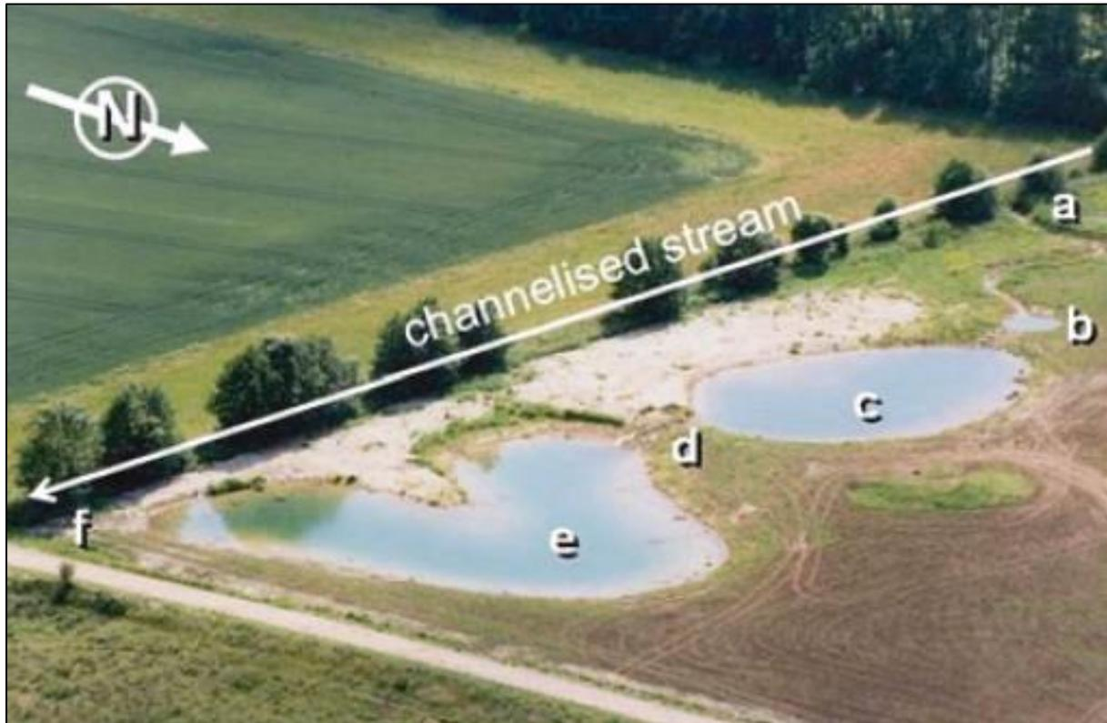
Figure 17. Overview of the stages in a riparian wetland in Hörby, Sweden: a. Diversion from the main channel into the wetland; b. Sediment trap; c. First wetland; d. Connective riffle; e. Second wetland; f. Wetland outflow to the main channel. (Olsson, 2001)
