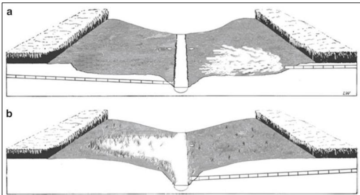
Figure 14. Visual representation of two methods that can be applied in tile-drainage alteration: a. Drainage-tiles opened up at the top of the stream valley; b. Drainage-tiles opened up into a horseshoe built within the riparian zone.
