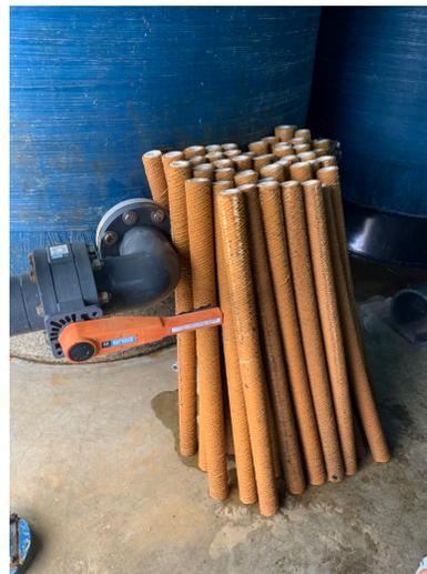
Figure 12: Filter Cartridge after routine maintenance and change. Taken by Briana Halley
