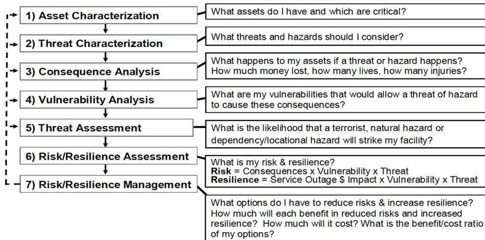
Figure 7: The seven step RAMCAP Plus Process. (Brashear & Jones, 2010).
