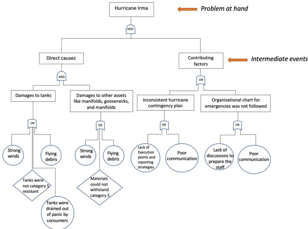
To explain the event tree above, Hurricane Irma was the main problem at hand which cause a major disruption to the water distribution system. The intermediate events describe what caused the system to fail and what attributing factors caused additional disturbance to the response and recovery period.
