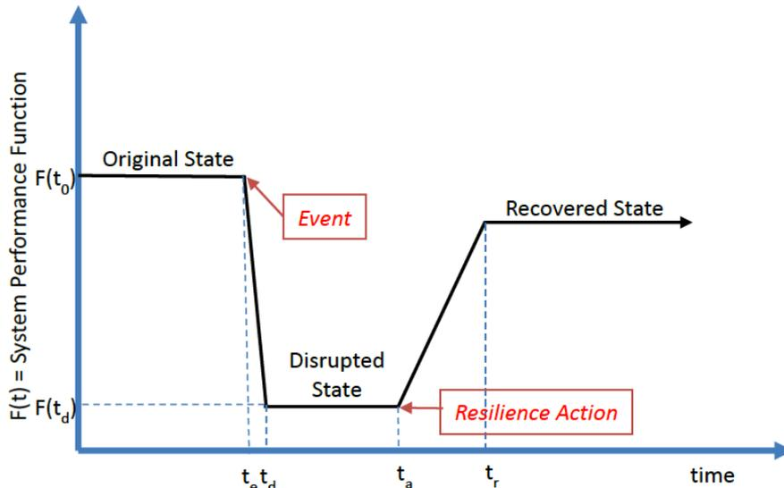
Figure 6: System performance function before, during, and after an event. (Systems Measures of Water Distribution System Resilience, 2015)
