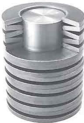
Disk springs are chosen, for their linear spring properties, and ability to handle high forces with small displacements. The disks can be stacked in different ways to adjust the spring characteristics, as illustrated in Figure 37. As illustrated in the graph, stacking them the same face up or upside down, either doubles the required force, or doubles the stroke.
