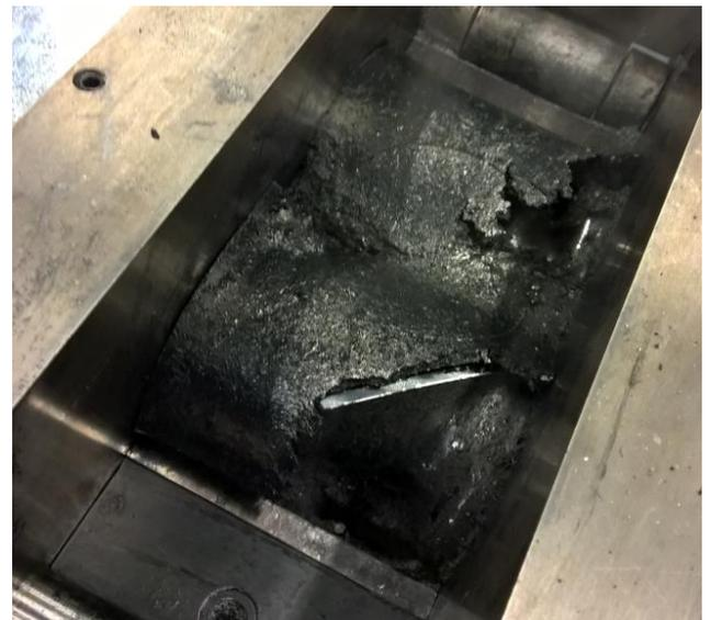
The consistency has a great effect on milling behaviour. The first batch stuck more to the surface of the roller and did not form a smooth sheet of rubber. Batches 2 and 3 stuck less to the roller and formed a uniform sheet, which accumulated on the faster turning roller as in Figure 12.
