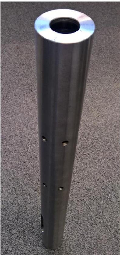
Figure 43, Roller shaft
