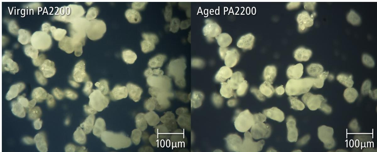
Figure 6: Particle shape of virgin and aged PA2200 from the Windesheim University, originating from the same batch.
