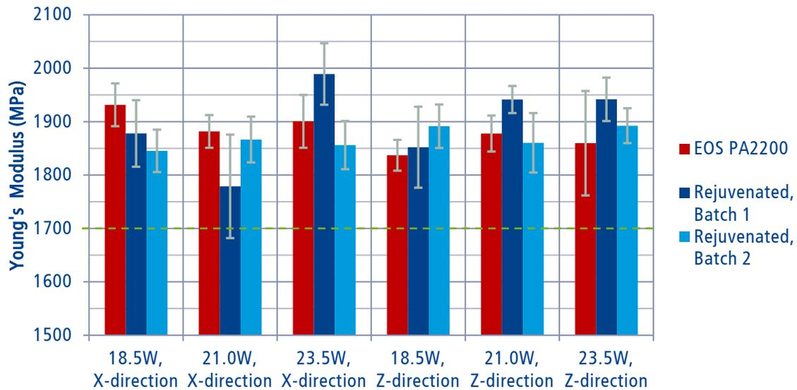
Figure 16: Comparison of Young's Modulus in the X- and Z-direction of rejuvenated versus standard PA2200 at various laser energies. The (green) dotted line is EOS' specification for PA2200 (Appendix A).
