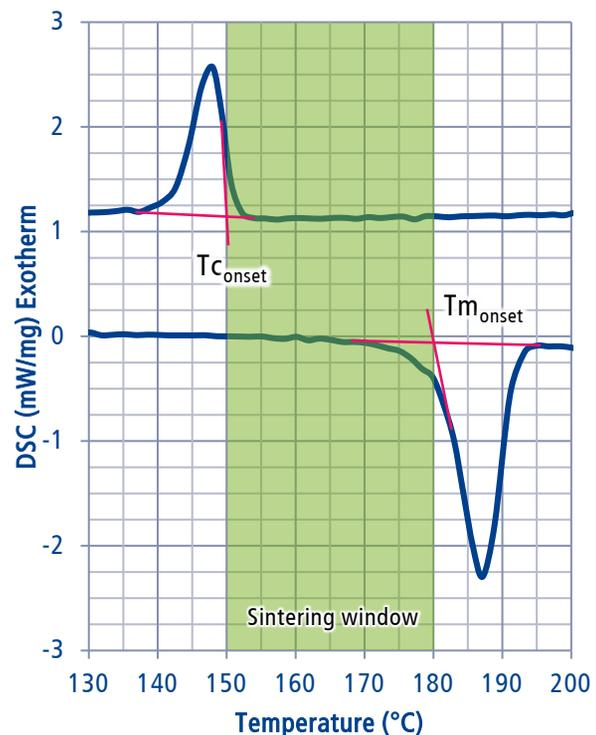
Figure 2: Schematic representation of a typical sintering window of SLS-PA12.
