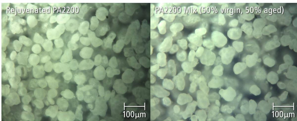
Figure 7: Particle shape of rejuvenated versus 50/50 mixed PA2200 powder.
