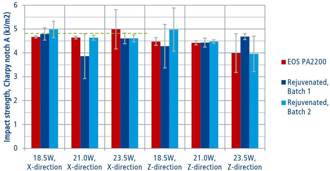
Figure 18: Comparison of Charpy notched (A) impact strength in the X- and Z-direction of rejuvenated versus standard PA2200 at various laser energies. The (green) dotted line is EOS' specification for PA2200 (Appendix A).
