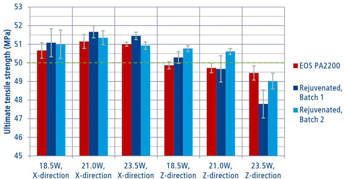
Figure 15: Comparison of Ultimate tensile strength (UTS) in the X- and Z-direction of rejuvenated versus standard PA2200 at various laser energies. The (green) dotted line is EOS' specification for PA2200 (Appendix A).
