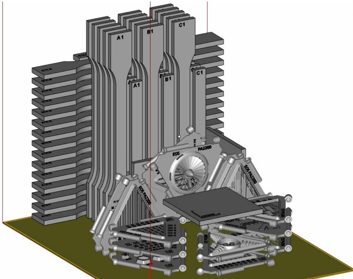
Figure 13: Layout for production of test specimens. The ochre plane in the lower part of the image represents the XY-plane / building area of the machine; the Z-direction is vertical.
