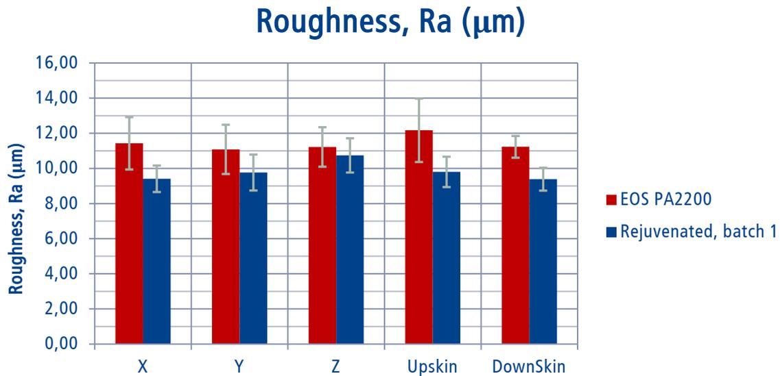
Figure 20: Roughness (Ra) measurement of standard material and batch 1 rejuvenated material.
