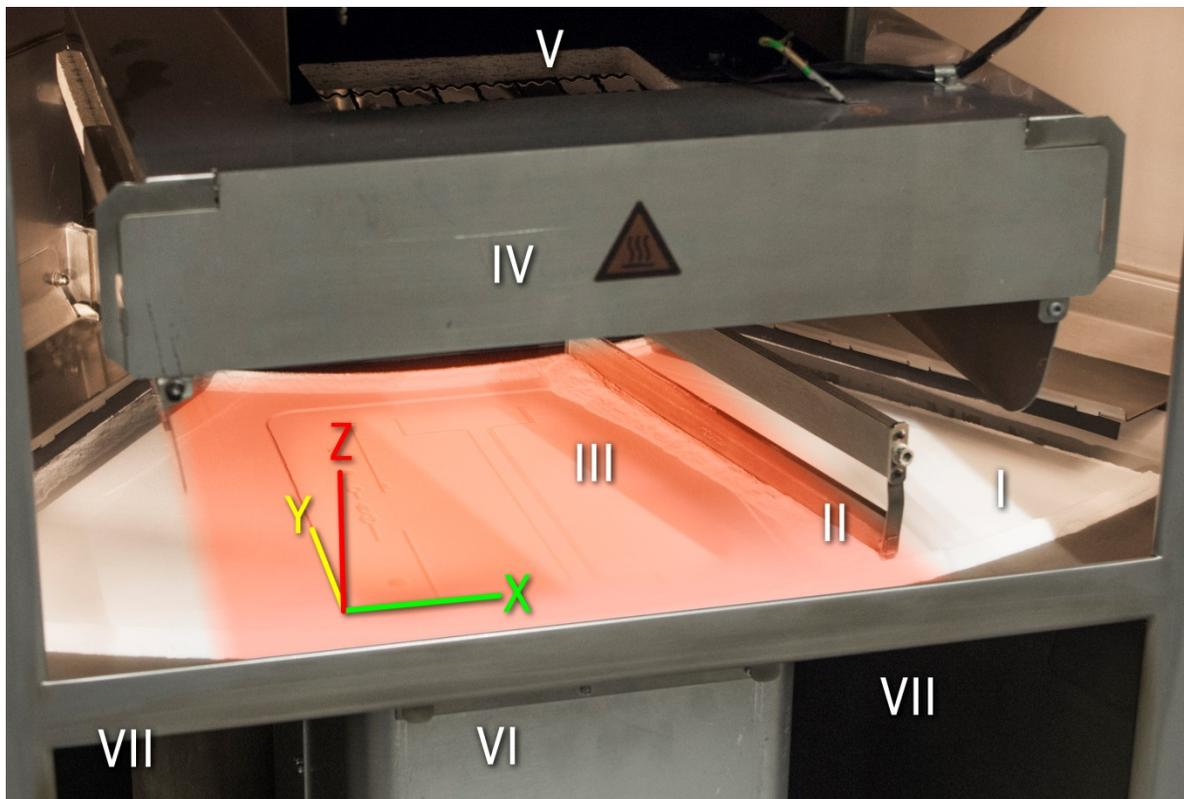
Figure 1: The building and removal chamber of the EOS Formiga P100 printer. The coordinate system and key components are marked for reference.
