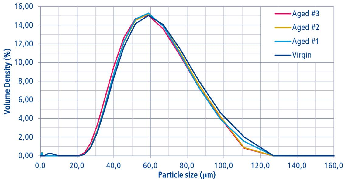
Figure 4: Particle size distribution on a linear scale.
