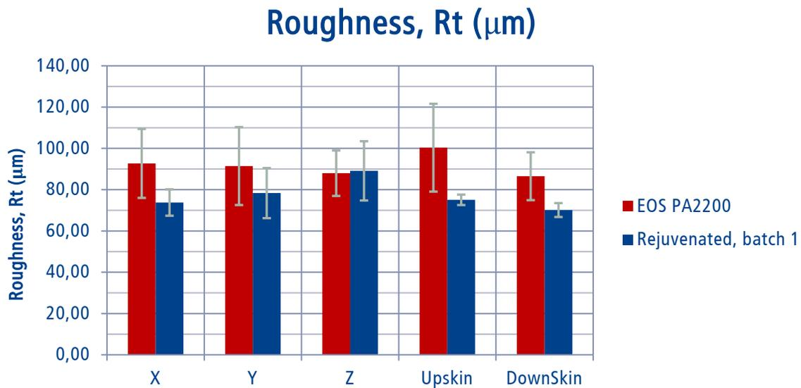
Figure 21: Roughness (Rt) measurement of standard material and batch 1 rejuvenated material.
