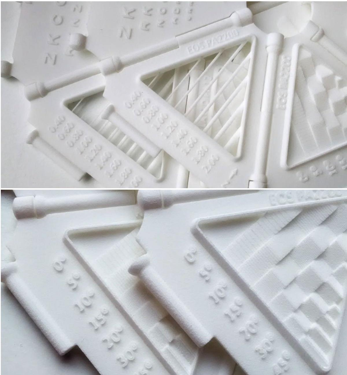
Figure 14: Comparison of visual properties of rejuvenated and standard PA2200. In both pictures, the rejuvenated material is on the left, and the PA2200 on the right (on top of the rejuvenated sample). No differences were found that distinguish the materials/products from each other.
