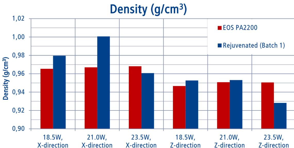
Figure 19: Density of standard material and batch 1 rejuvenated material, measured using the impact test specimens.
