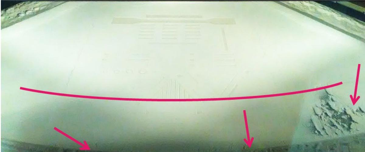
Figure 11: Powder bed during initial testing, where a breakup of the powder bed is visible near the arrows. The breakup only occurred in the front area of the printer, in front of the indicated line and outside the actual sintering area.
