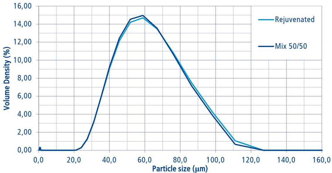
Figure 8: Particle size distribution plot of rejuvenated versus 50/50 mixed PA2200 powder.
