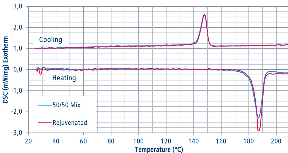
Figure 9: DSC plot with a heating and cooling curve of rejuvenated PA2200 and a 50/50 mix of virgin and aged PA2200.
