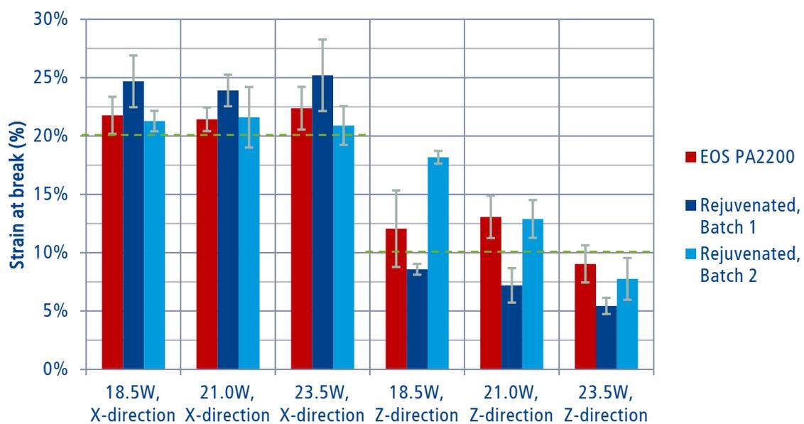
Figure 17: Comparison of Strain at break in the X- and Z-direction of rejuvenated versus standard PA2200 at various laser energies. The (green) dotted line is EOS' specification for PA2200 (Appendix A).
