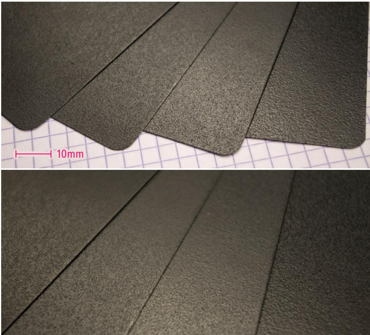
*Figure 5: The coating samples using different types of powder. Top: overview picture. Bottom: detail picture. In order from left to right on each picture: Commercial Belticryl coating, coating with aged powder #1, coating with aged powder #2 and coating with aged powder #3. The coatings are 40-50 $\mu$ m thick and feature the same concentration of powder.*
