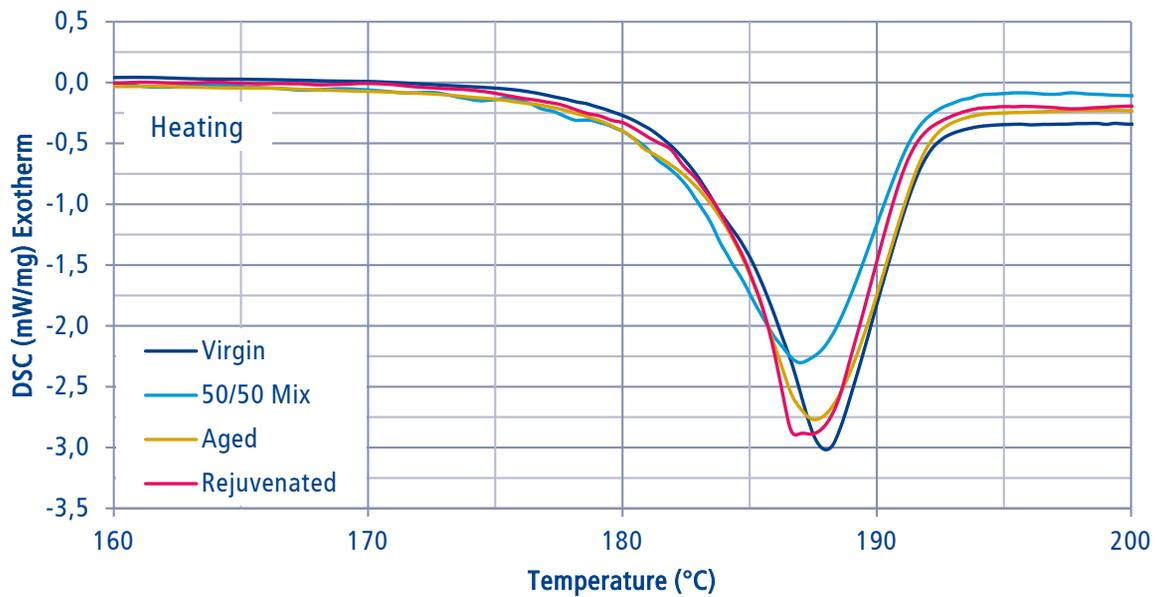
Figure 10: Melting peak from DSC measurements of PA2200 with various types of thermal history and treatment.
