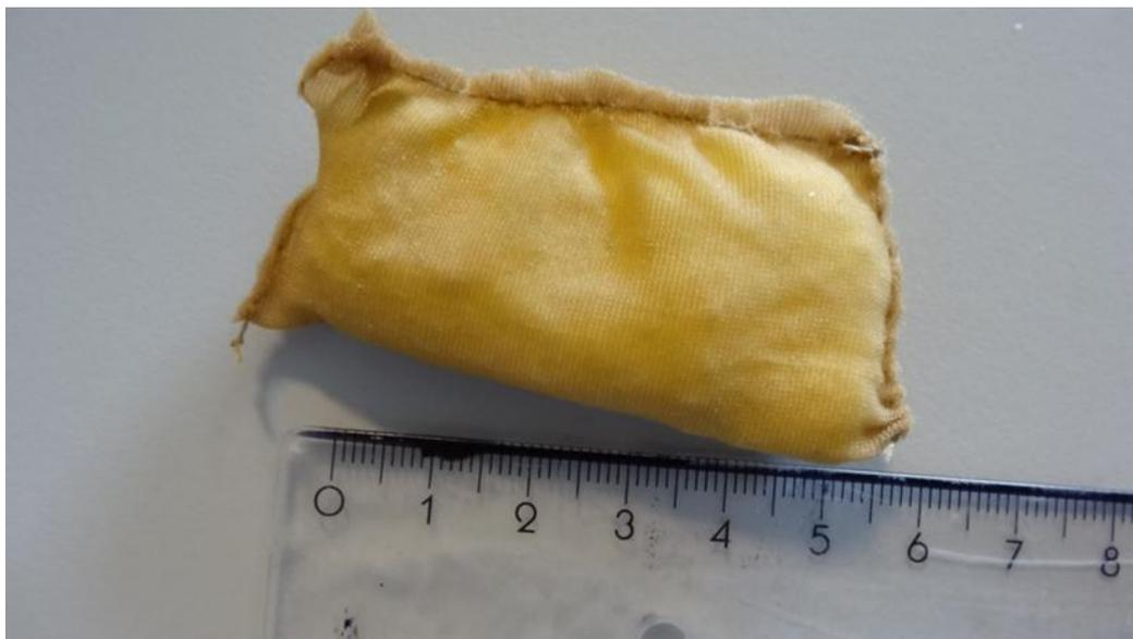
**Figure 8. Permeable nylon bag containing EcoTech Oil Foam made from panties.**
