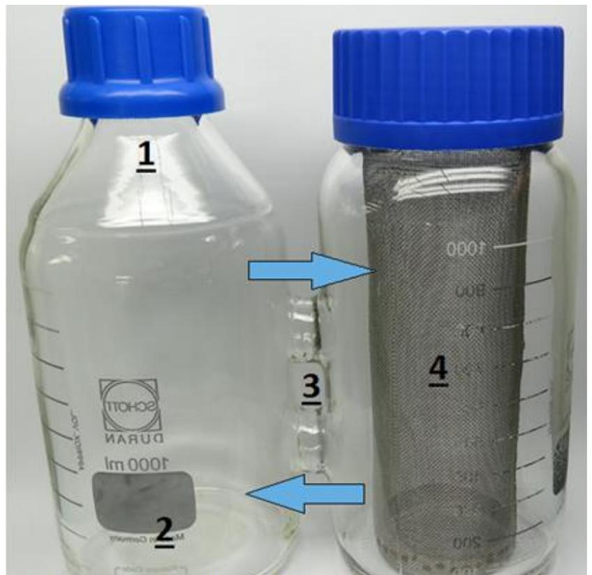
Figure 7. Schott Duran double-bottles used during research. 1) Surface layer of the first bottle contained the layer of oil or oil-dispersant. 2) This side of the structure was placed above a stir plate, a stir bean on the bottom of the flask provided a circulating. 3) The glass tubes enabled a circulation of water from the oil carrying flask through the second flask. 4) The second flask contained a mesh cylinder in which *C. volutator* were kept.
