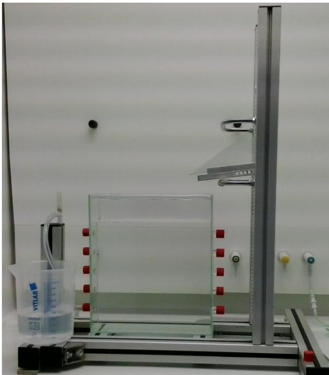
Figure 1. Plunging jet system
