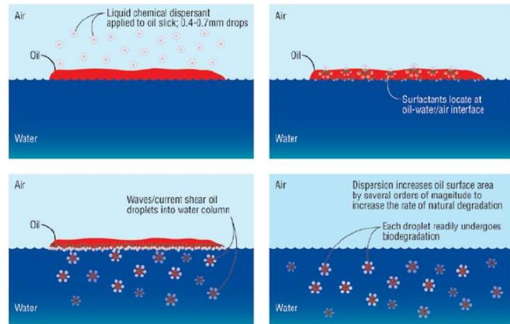
**Figure 3. The schematic working of a dispersant on an oil slick** (Potter, Buist, Trudel, Dickins, & Owens, 2012).
