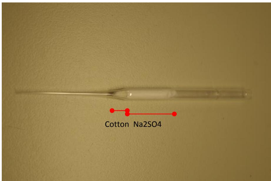
Figure 4 glass pasteur pipette with cotton and dried  $\text{Na}_2\text{SO}_4$
