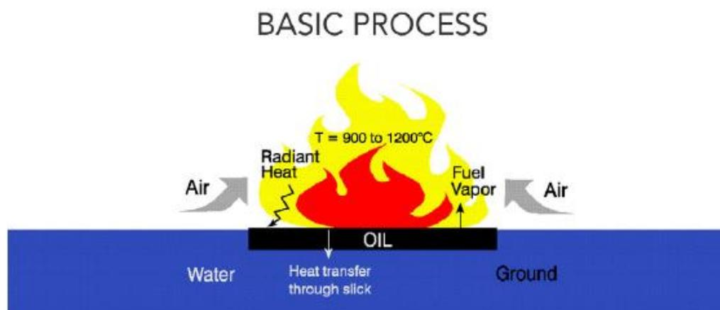
Figure 2. The basic process of *In-situ* burning of an oil slick. Keep in mind the figure does not contain information concerning possible toxic effects (Bothe et al., 2014).
