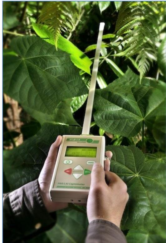
Figure 13: Septometer (Source: decagon)
