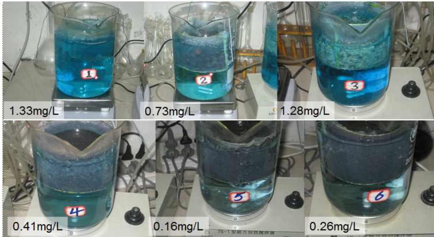
In 10 minutes of the experiment Decomposition of Methylene Blue with minerals and aeration
