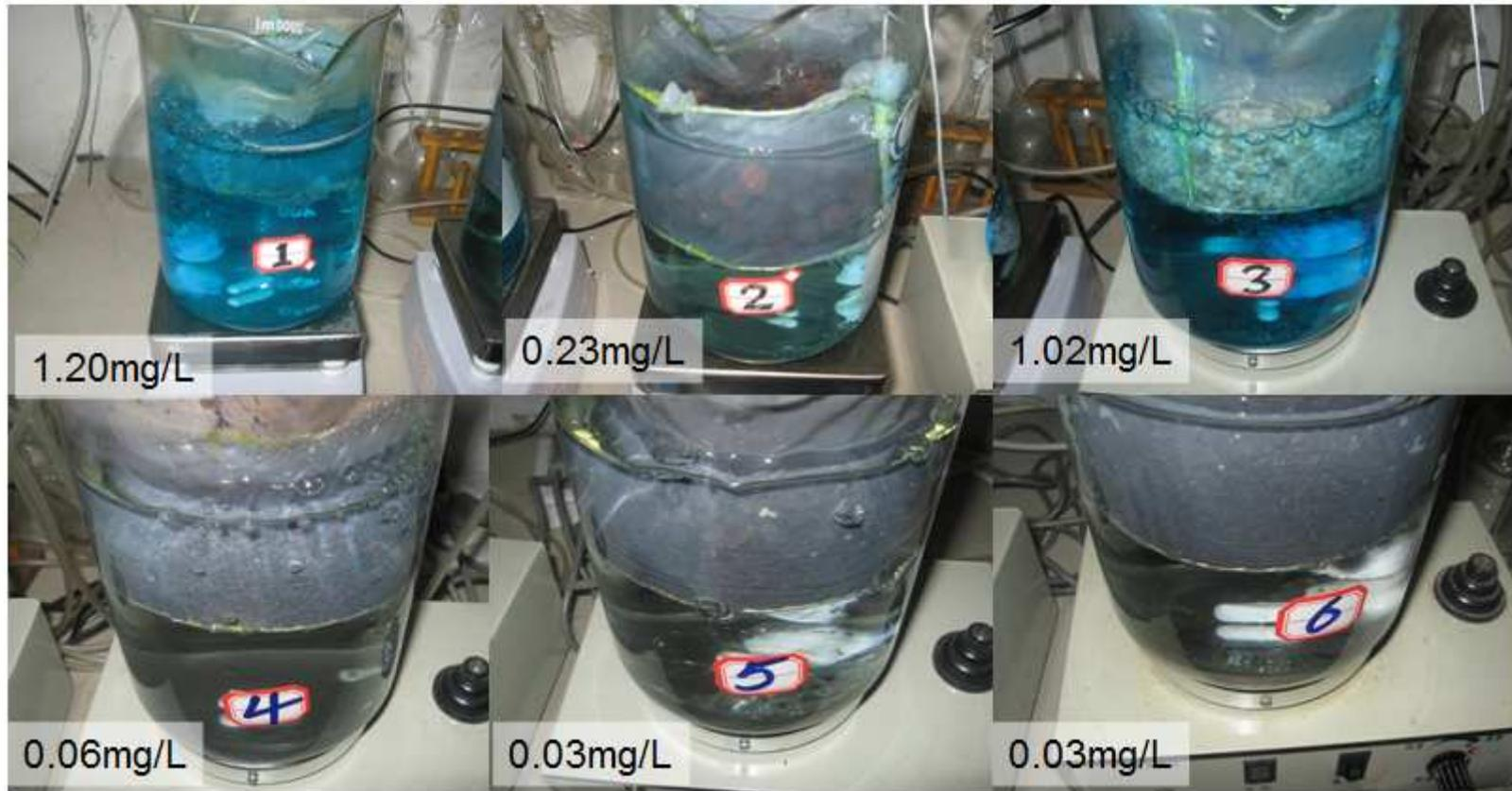
In 60minutes of the experiment Decomposition of Methylene Blue with minerals and aeration
