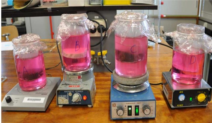
Figure 4 Decolorization of Reactive red 2 at the surface of Magnetite without aeration.
