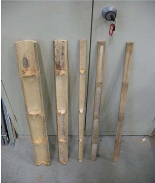
Firstly, the culms were sawn lengthwise into 8 strips using a circular saw (first in halves, then in quarters and finally in eights). Following this, the remaining parts of the diaphragms were removed with a band saw. Next, the strips were planed to the desired thickness by a planing machine. Finally, the strips were edged by planing one side on the joiner’s bench, which allowed the other side to be edged by the circular saw.
