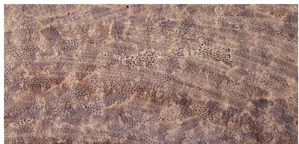
Figure 53 Transverse surface (bamboo composite of BambooXL - dark)
