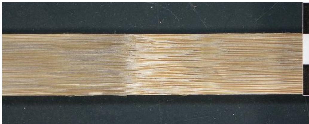
Figure 22 Guadua - tangential surface, inside of culm wall, with node (1 stripe equals 1 cm)
