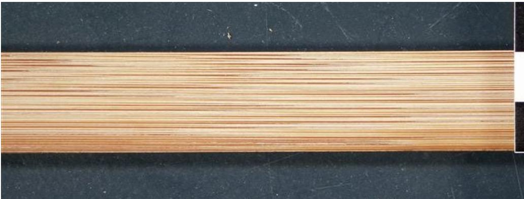
Figure 18 Moso - tangential surface, outside of culm wall (1 stripe equals 1 cm)
