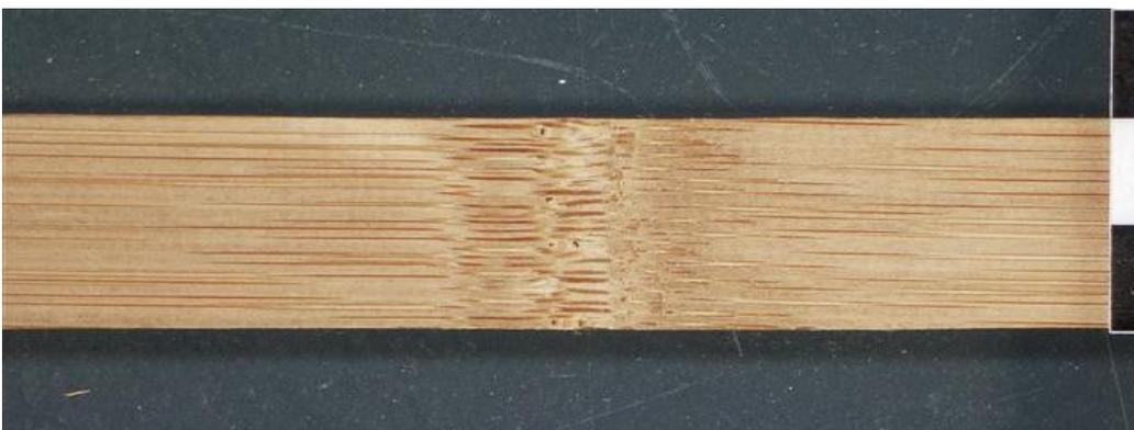
Figure 19 Moso - tangential surface, inside of culm wall, with node (1 stripe equals 1 cm)
