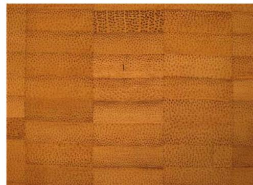
Figure 51 Transversal surface of laminated strips of ±2 cm wide, plain-pressed (product from GreenBoo)
