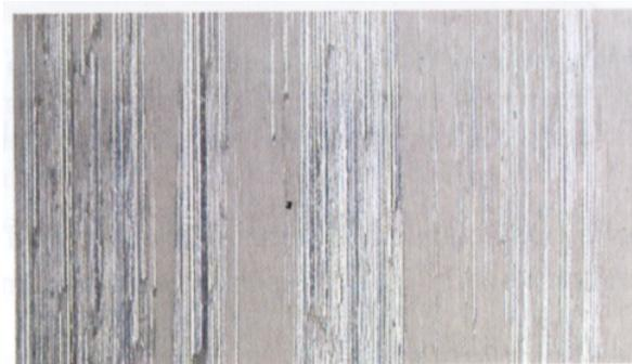
Figure 2-1 Example of adhesive wear [4]
