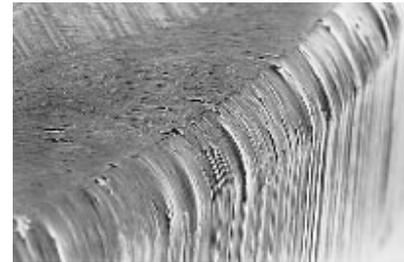
Figure 2-2 Punch edge showing abrasive wear [4]
