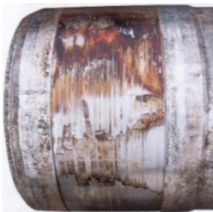
Figure 2-3 Corrosive wear on chrome steel bushing [4]
