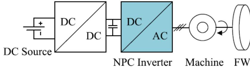
Figure 17 DC/DC plus Neutral Point Clamped (NPC) inverter [3]
