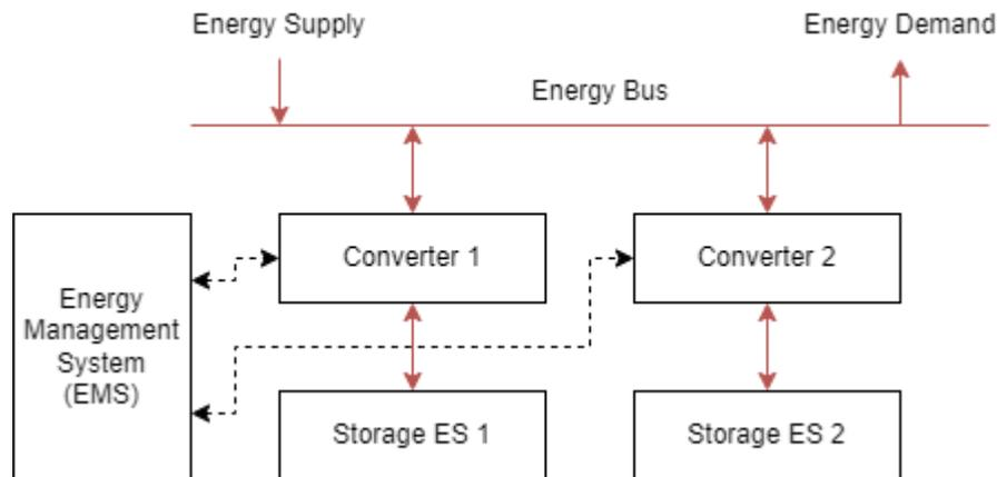
Figure 11 Possible HESS topology with two storage devices
