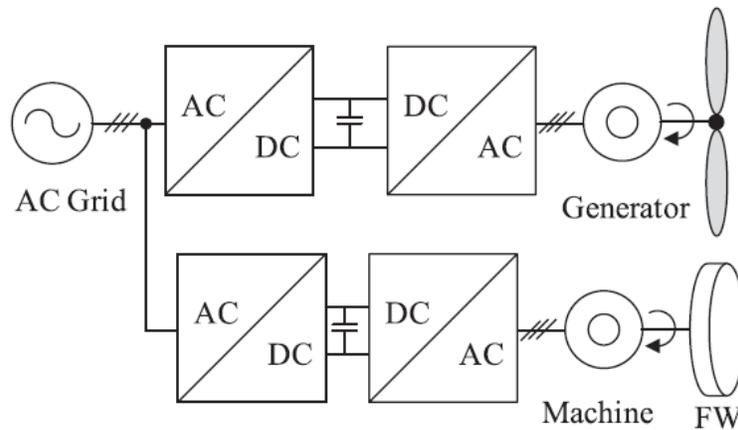
Figure 14 Back-To-Back power converter connected directly to the grid [3]
