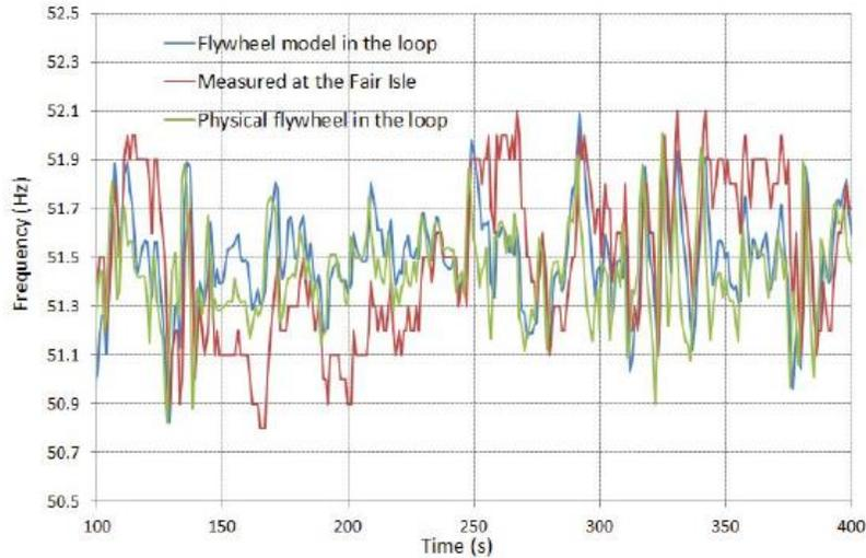
Figure 9 Service load frequency with and without Flywheel [32]
