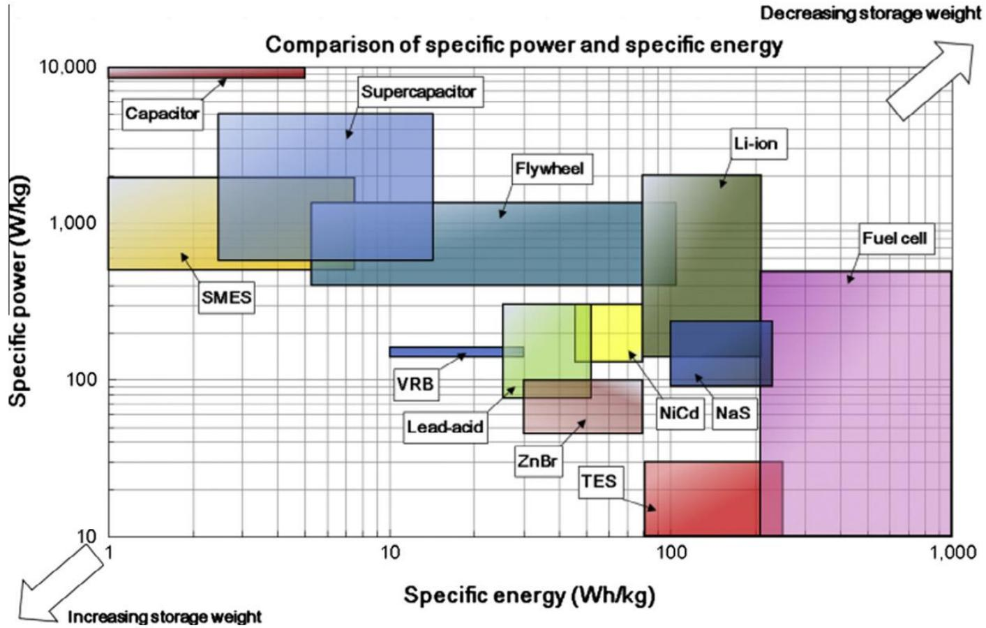
Figure 22 Comparison of specific power vs specific energy [17]
