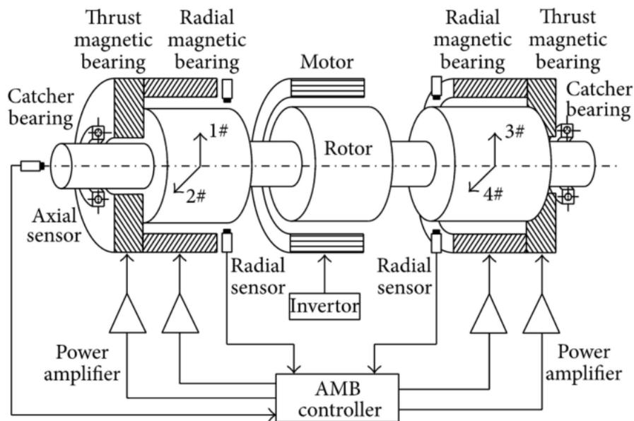
Figure 3 Active magnetic bearings system [11] [12]
