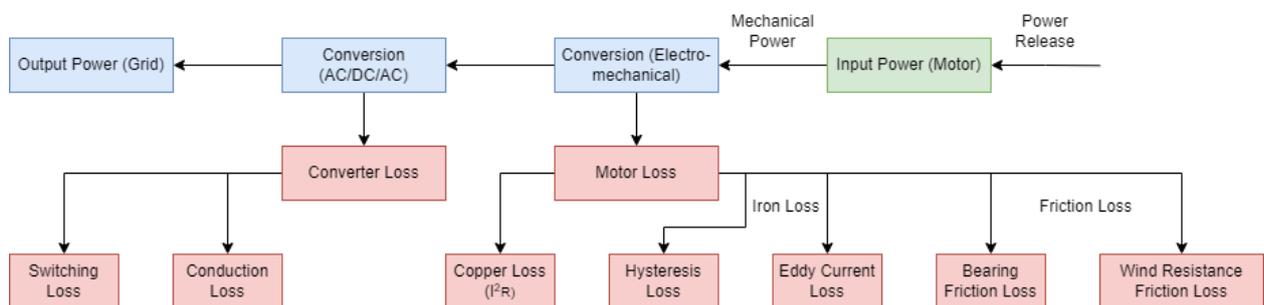
Figure 6 Discharge energy conversions and losses [20]
