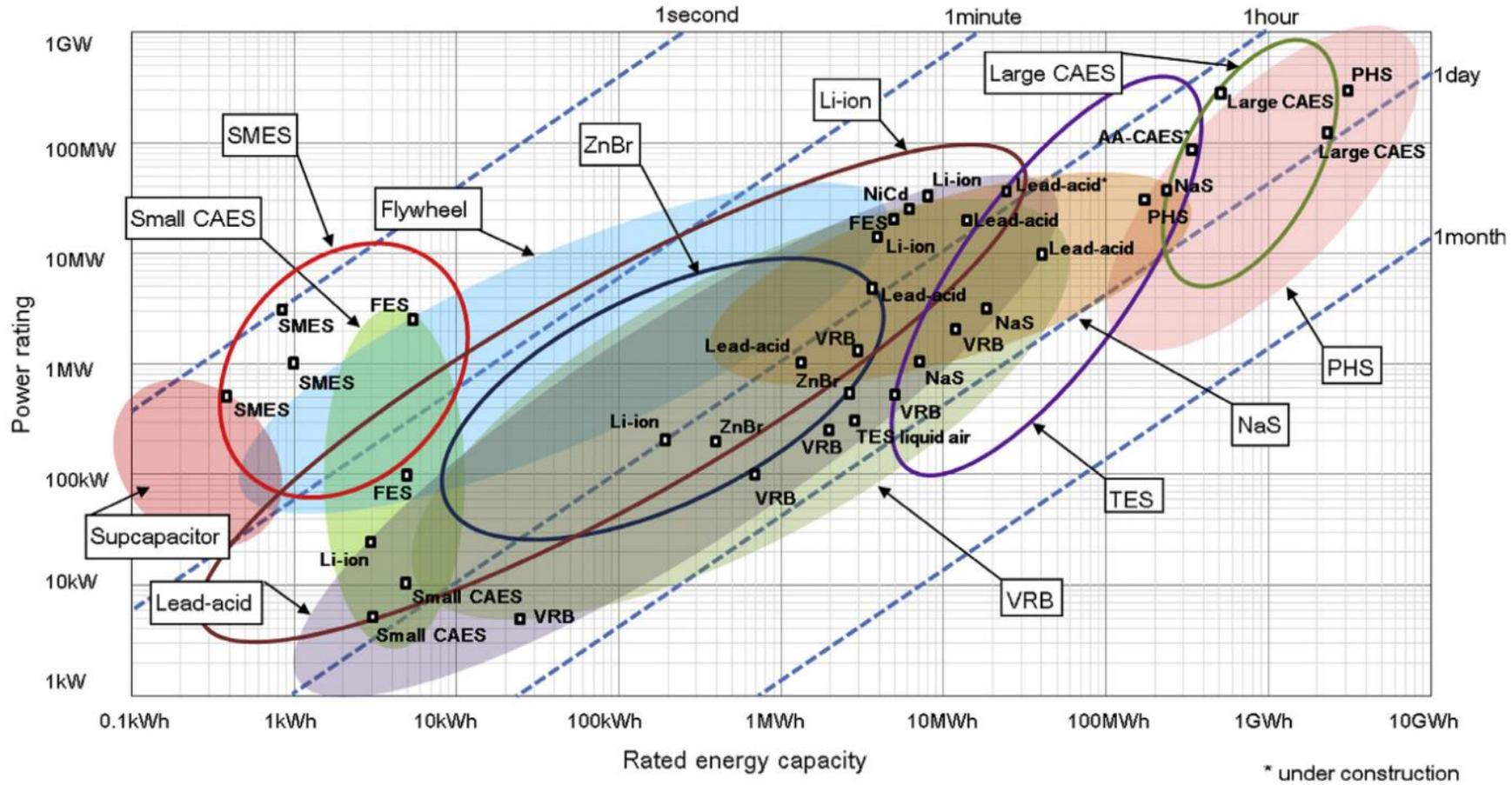
Figure 20 Comparison of power rating vs rated energy capacity [17]
