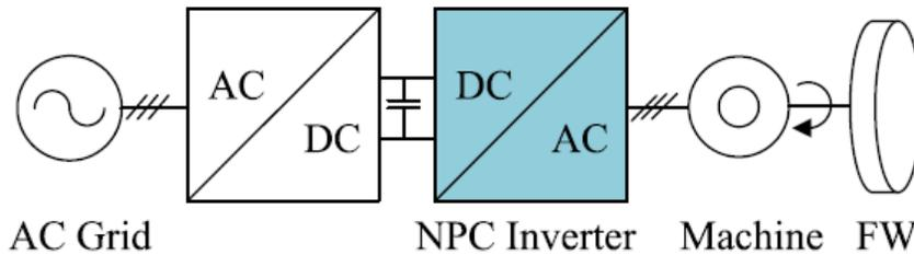
Figure 18 AC/DC plus NPC inverter [3]
