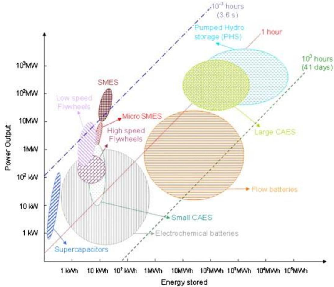
Figure 24 Comparison of Power output vs energy stored [44]
