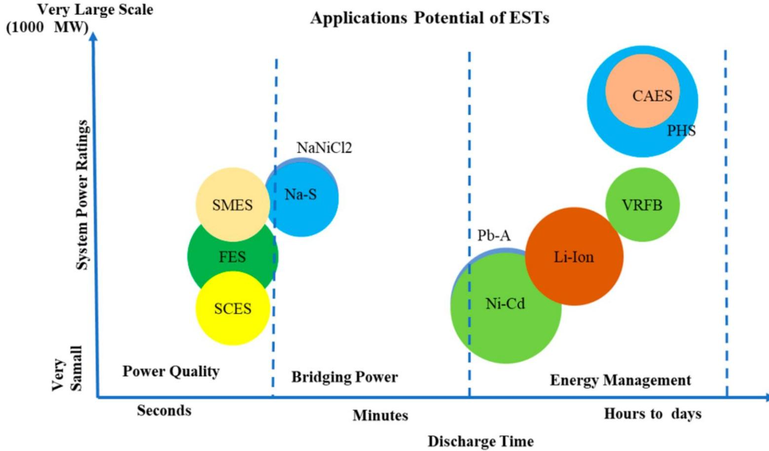
Figure 21 Comparison of power rating vs discharge time [18]
