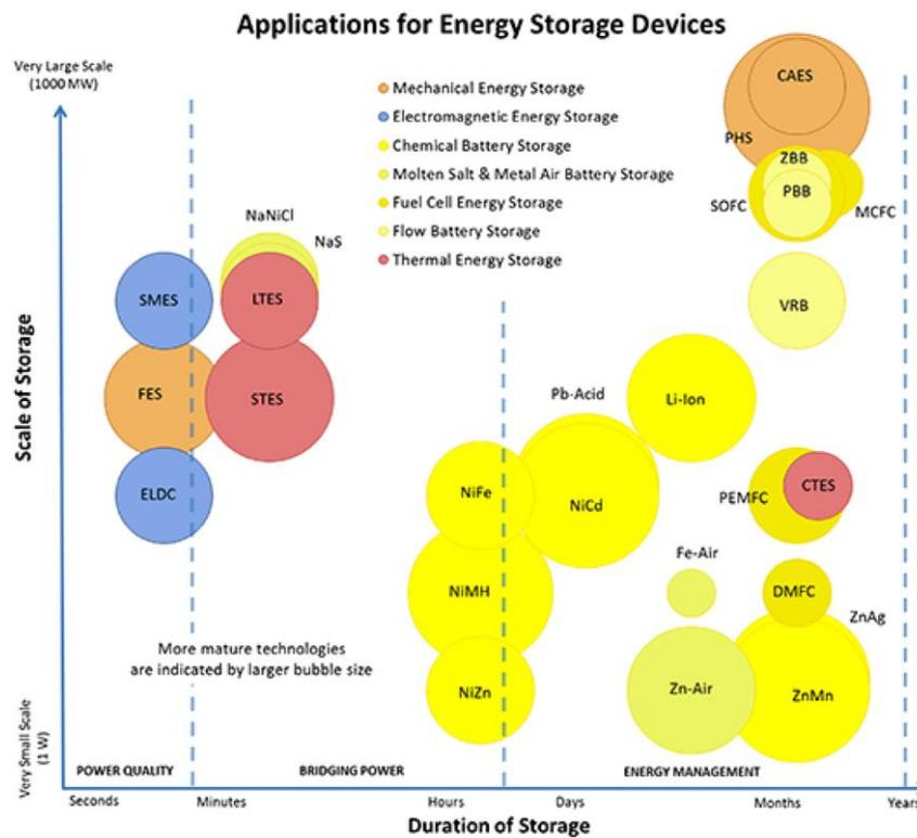
Figure 7 Comparison of scale of storage vs duration of storage [21]
