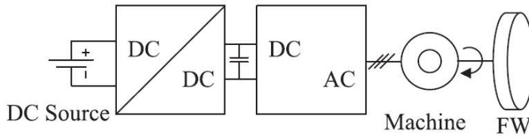
Figure 16 DC/DC plus AC/AC configuration [3]
