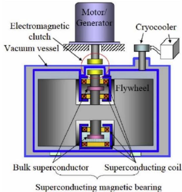
Figure 4 Superconducting magnetic bearings system [11] [14]
