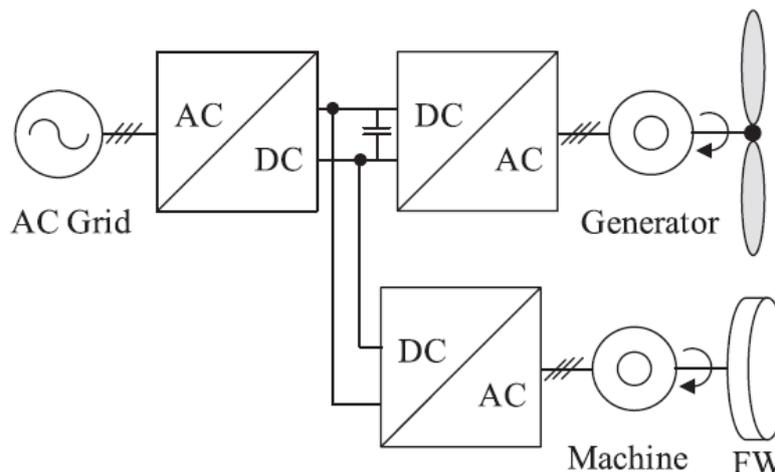
Figure 2 Back-To-Back power converter [3]
