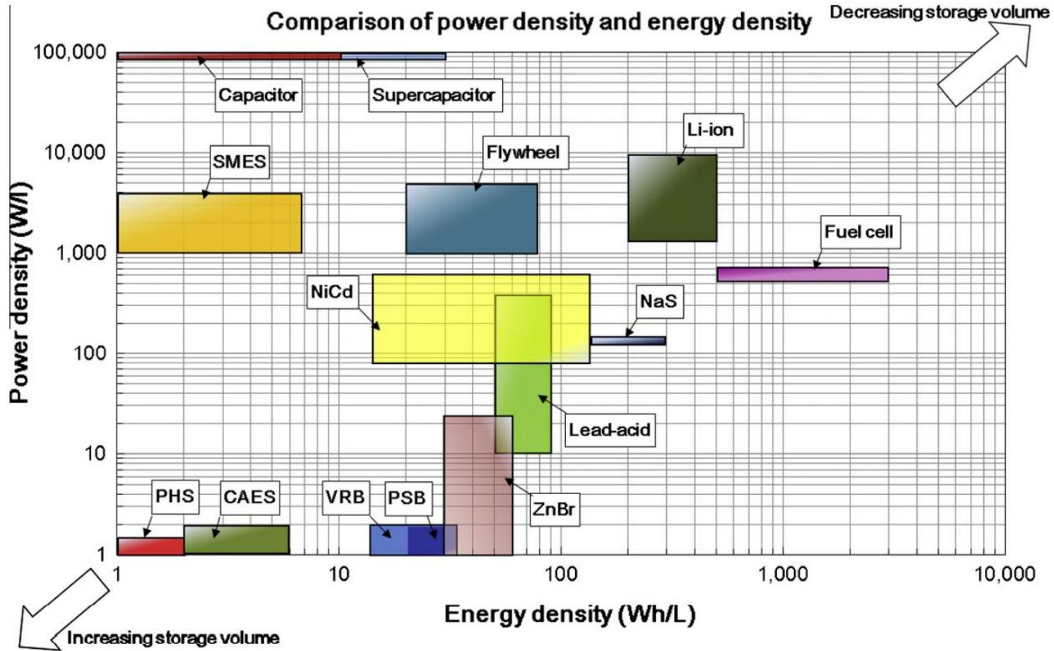
Figure 23 Comparison of power density vs energy density [17]
