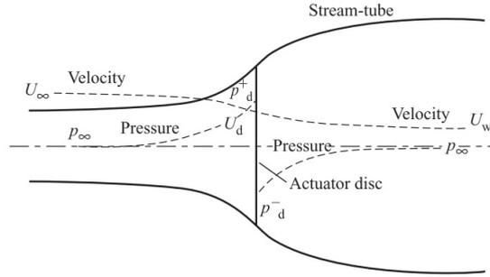
Fig. 1: Schematic representation of the actuator disc momentum theory.
