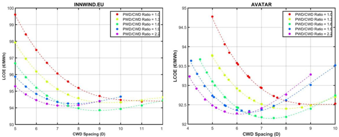
Fig. 4: Levelised cost of electricity (LCoE) for INNWIND.EU (left) and AVATAR (right) wind farms in all layout configurations including electrical losses.
