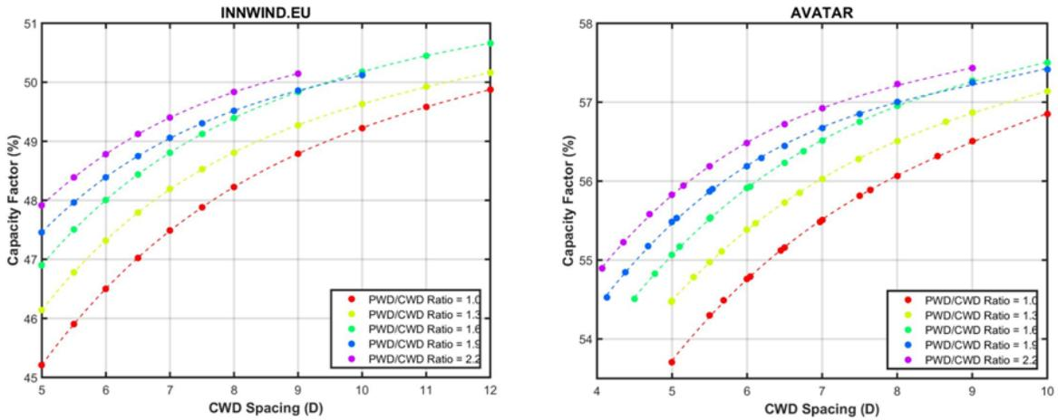
Fig. 3: Capacity factor for INNWIND.EU (left) and AVATAR (right) wind farms in all layout configurations including electrical losses.
