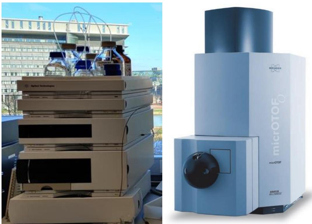
Figure 7: (left)
