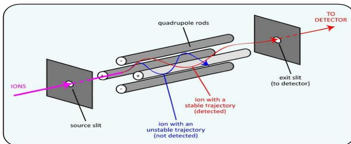
Figure 5: Schematic overview of a QMS.<sup>[29]</sup>
