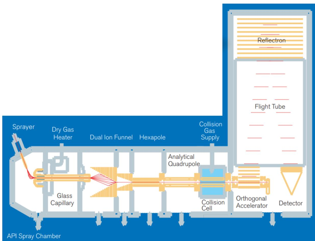
Figure 3: A schematic overview of the QTOF MS used in this study.<sup>[27]</sup>
