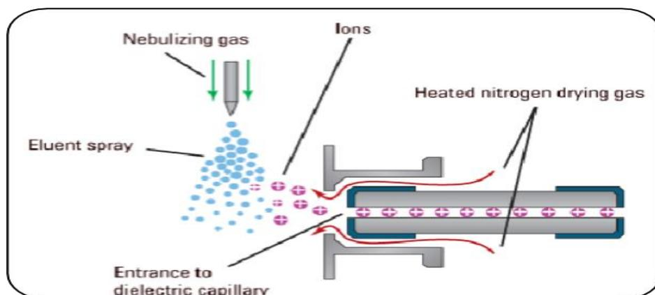
Figure 4: A schematic overview of the mechanism of electrospray ionization.<sup>[28]</sup>
