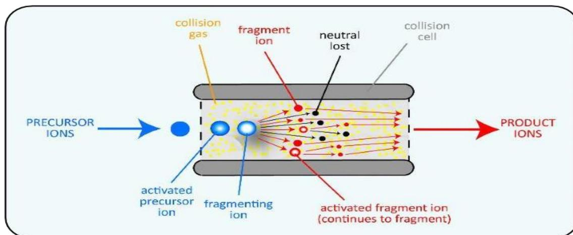
Figure 6: Schematic overview of a collision cell.<sup>[29]</sup>
