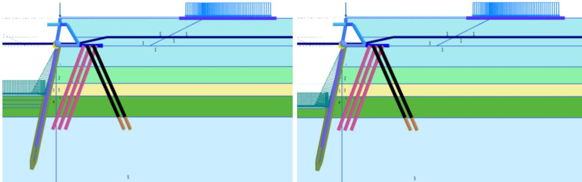
Figure 16 Plaxis model before deepening (left side) and after deepening (right side)
