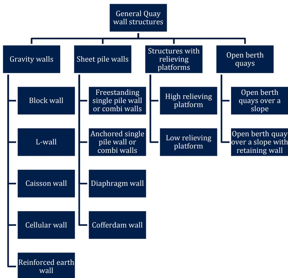
Figure 5 main types of quay wall structures
