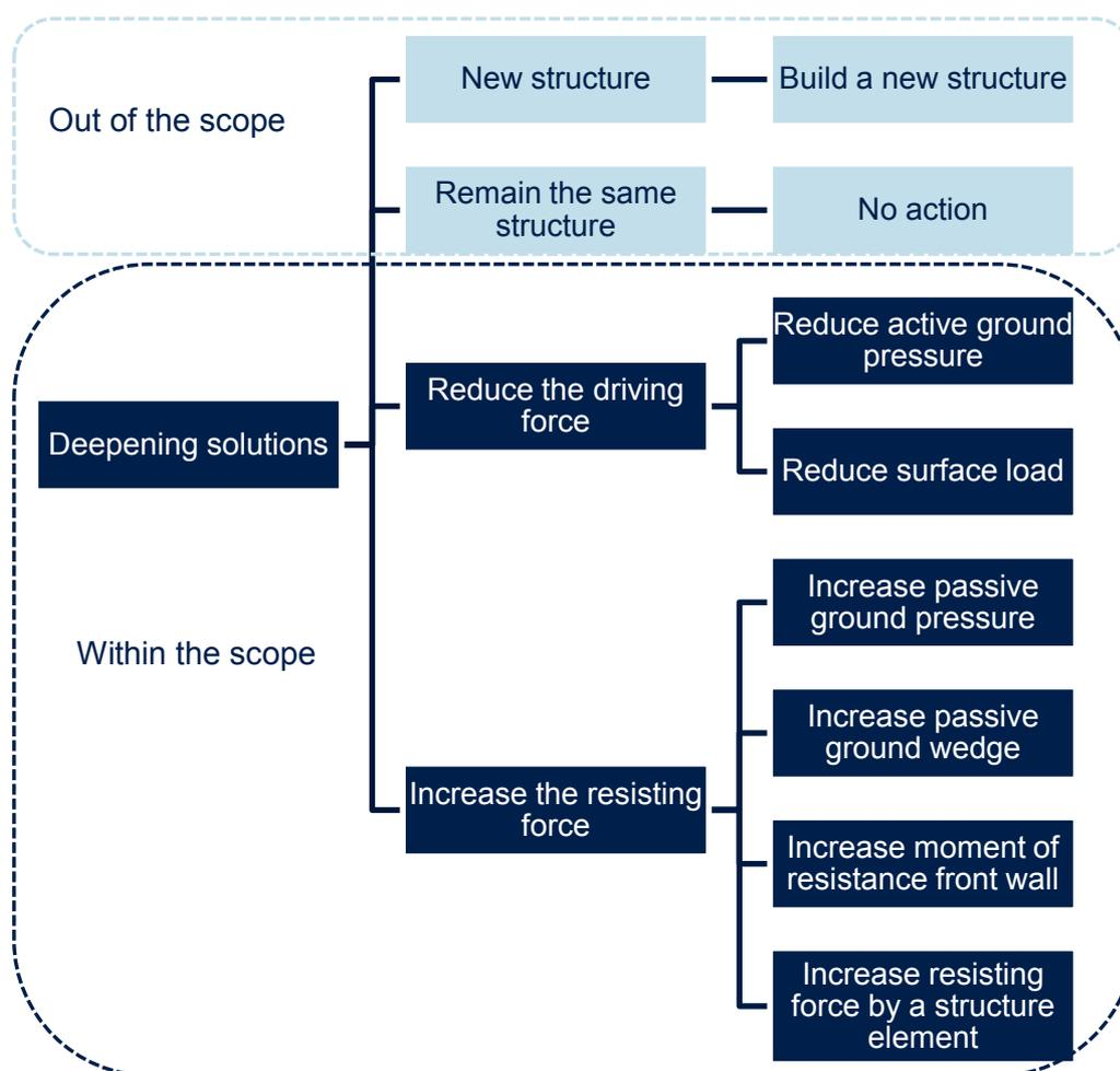
Figure 22 type of upgrading solutions
