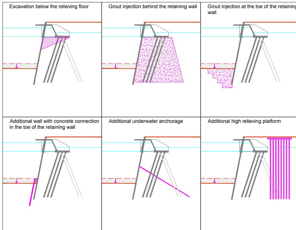
Figure 28 preselected best solutions to deepen a combi wall structure
