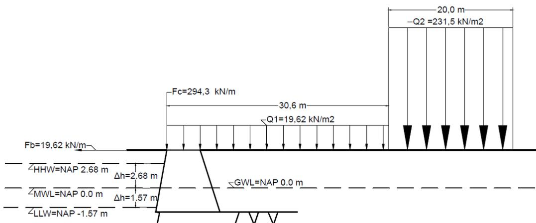
Figure 14 modulation of the loads
