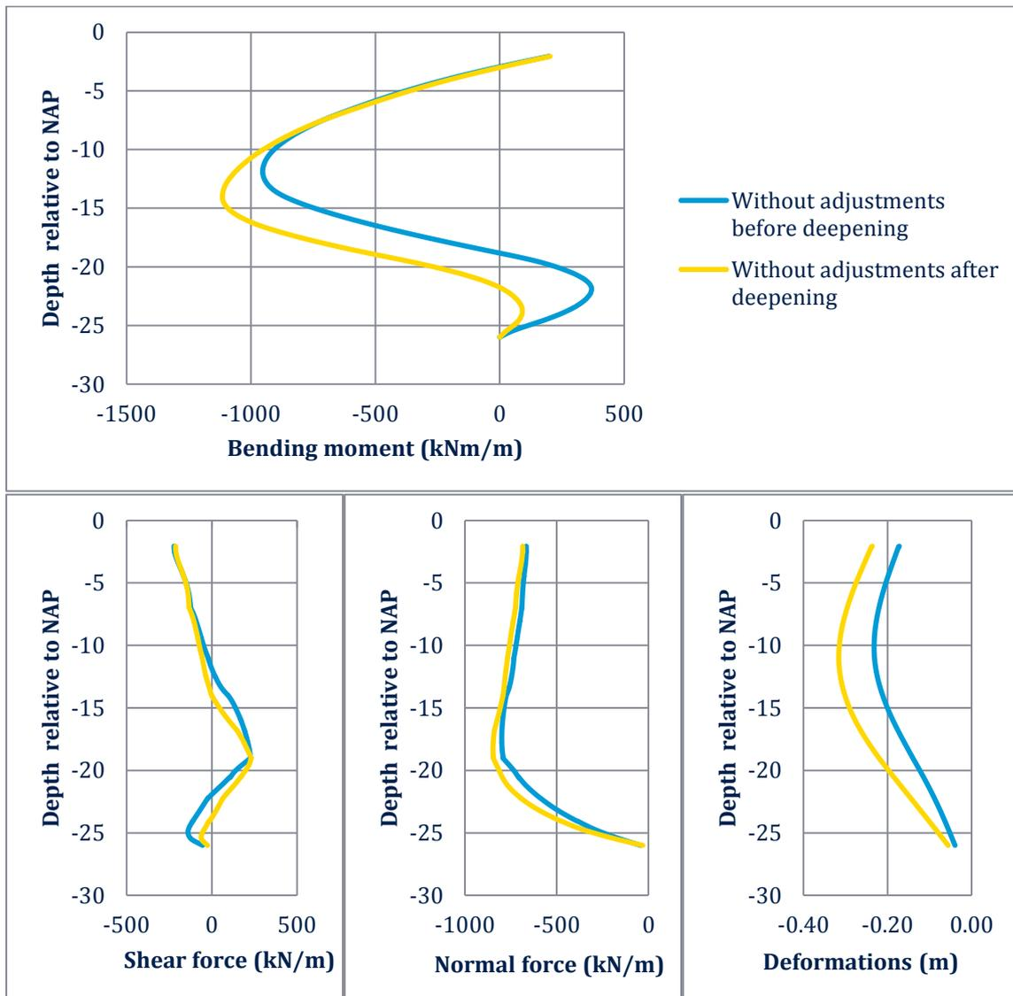
Figure 19 results of the front wall: bending moment, shear force, normal force and deformations, before (blue) and after deepening (yellow)
