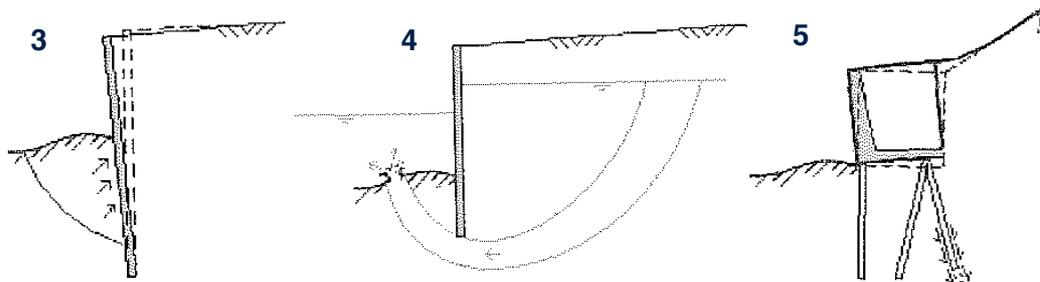
Figure 21 visualisation of the geotechnical failure mechanism (SBRCURnet, 2014)
