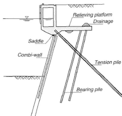
Figure 7 principle of a low relieving platform (SBRCURnet, 2014)
