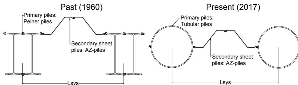
**Figure 2 typical combi wall type in the Port of Rotterdam**
