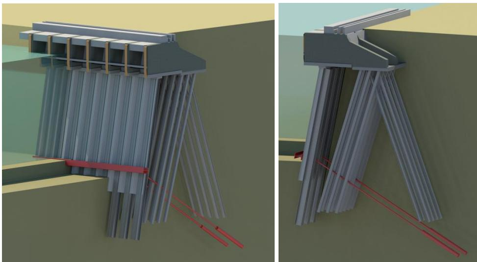
**Figure 2 visualisation of the additional underwater anchorage (red) in the existing quay wall**
