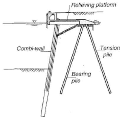
Figure 6 principle of a high relieving platform (SBRCURnet, 2014)
