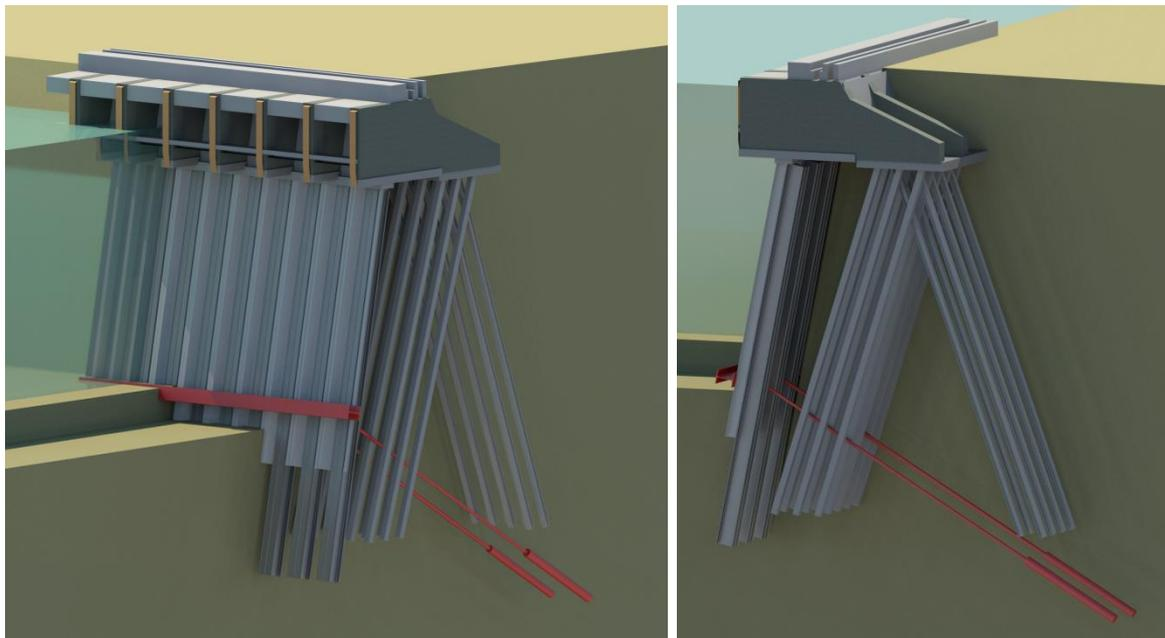
Figure 29 visualisation of the additional underwater anchorage (red) in the existing quay wall
