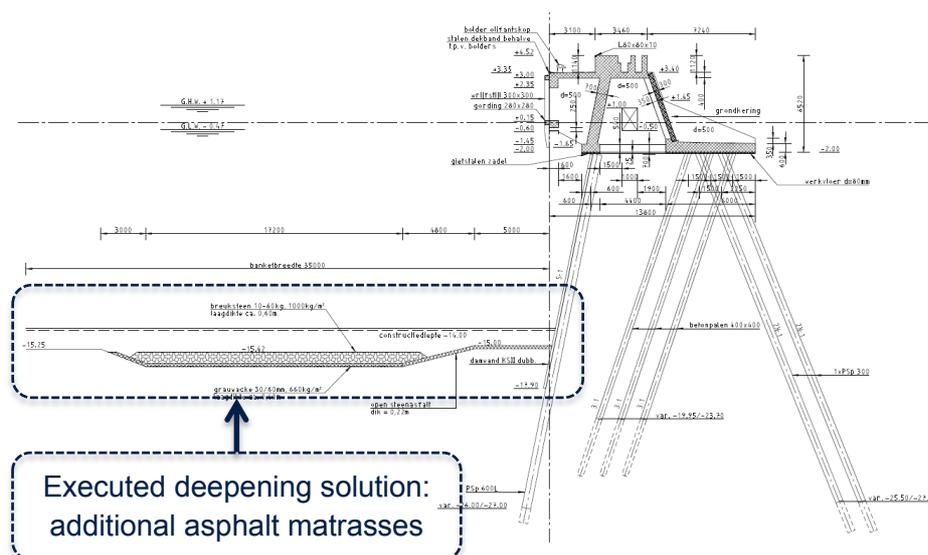
Figure 9 principle cross section reference structure with adjustment
