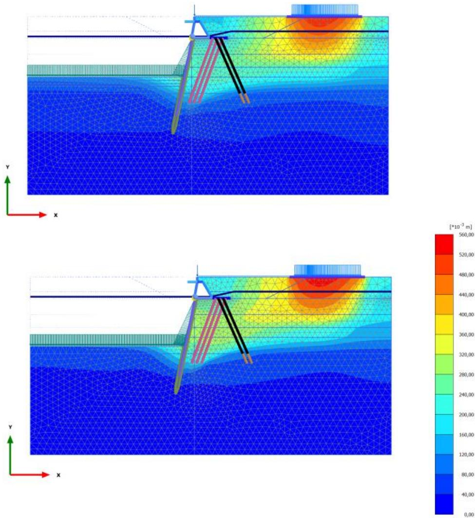
Figure 17 total displacements before deepening (upper figure) and after deepening (bottom figure)
