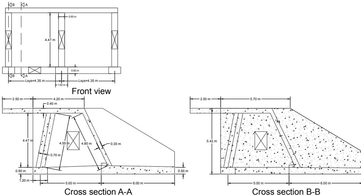
Figure 12 overall overview of the superstructure front view and cross section A-A and B-B
