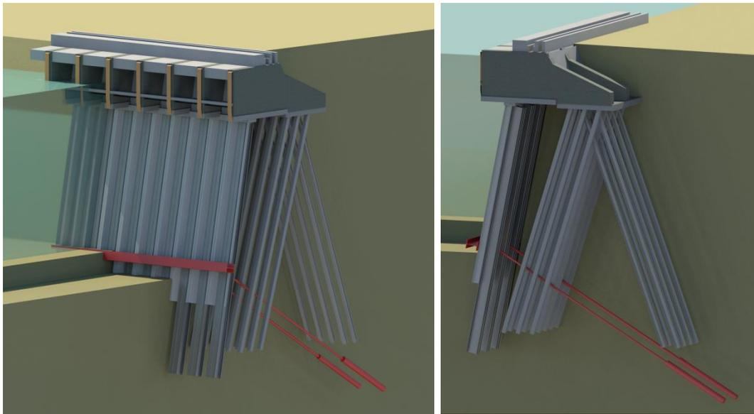
Figure 27 schematisation of the application of underwater anchorage
