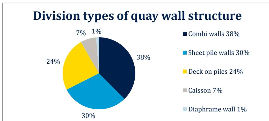
**Figure 3 deviation of quay wall types in the Port of Rotterdam (Port of Rotterdam Authority 4, 2017)**
