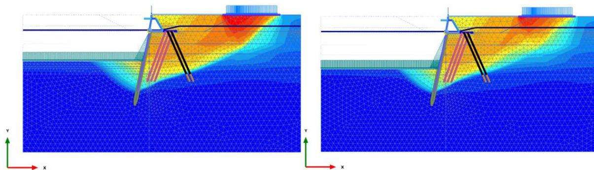
Figure 18 total displacements  $\sum Msf$  before deepening (left figure) and after deepening (right figure)
