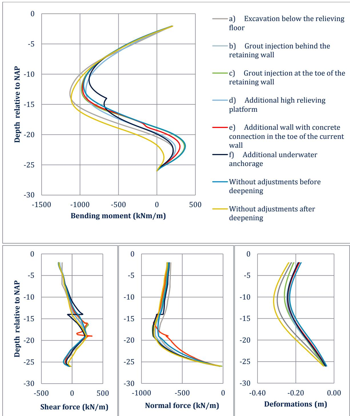
Figure 26 results of the bending moment, shear force and normal force of the front wall
