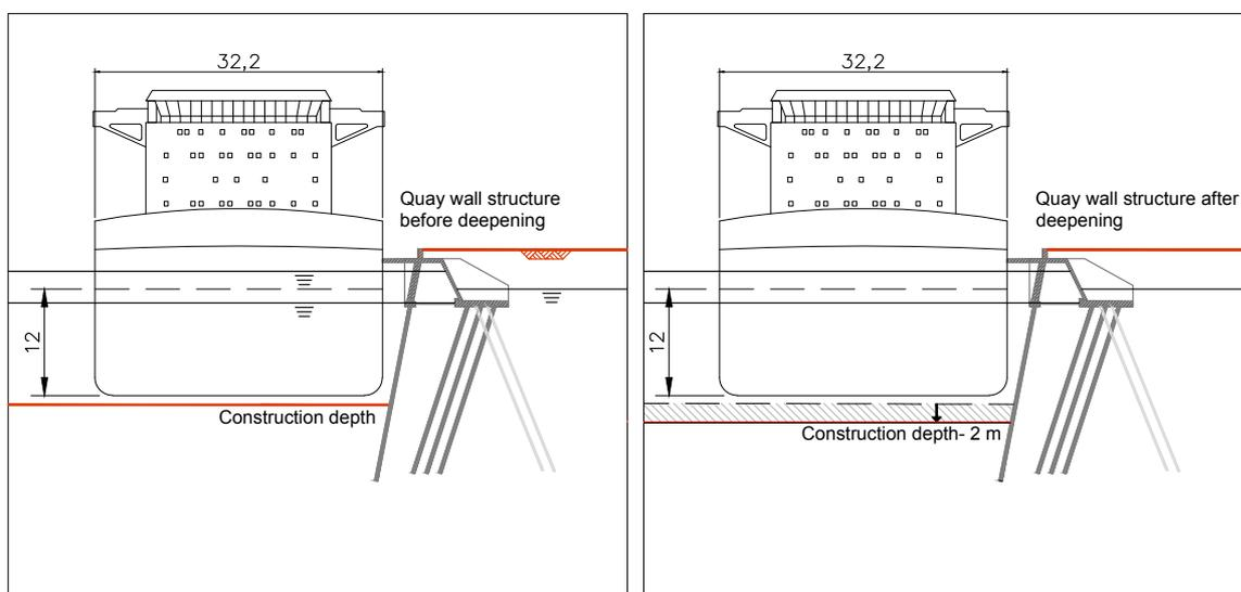
Figure 10 principle cross section before deepening (left side), and after deepening (right side)
