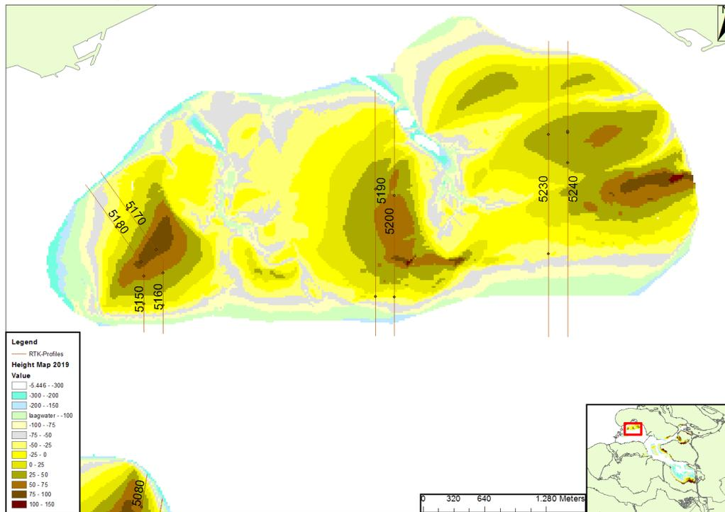
Figure 8. The RTK profiles on the intertidal flat Roggenplaat and the coloured areas are the Vaklodging data of the year 2019.
