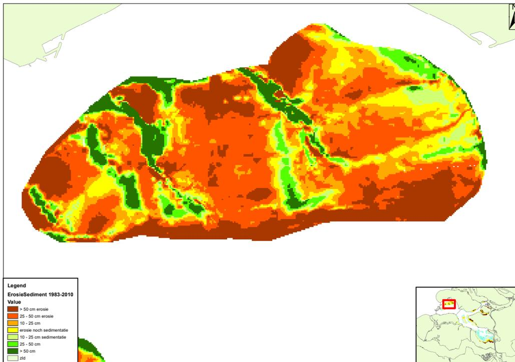
Figure 15. A visualisation of the Vaklodging difference between 1983 and 2010 of the intertidal flat Roggenplaat. The red colour is erosion and the green colour sedimentation.
