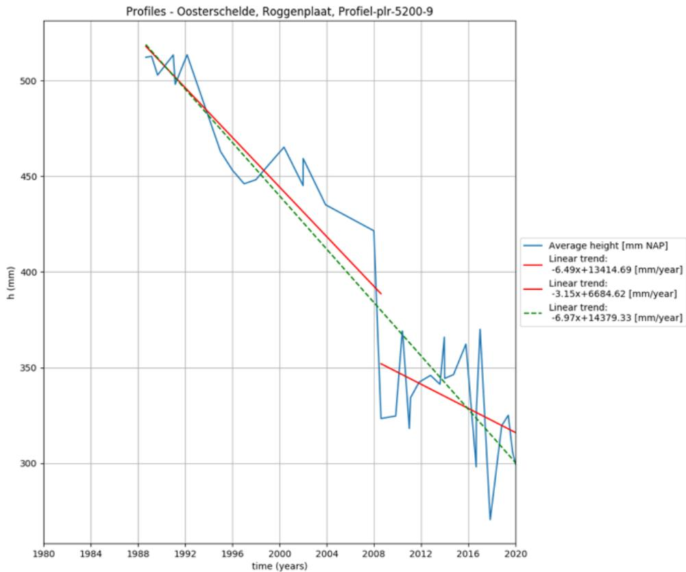
Figure 32. Multiple regressions of the profile Profiel-plr-5200-9, Roggenplaat.
