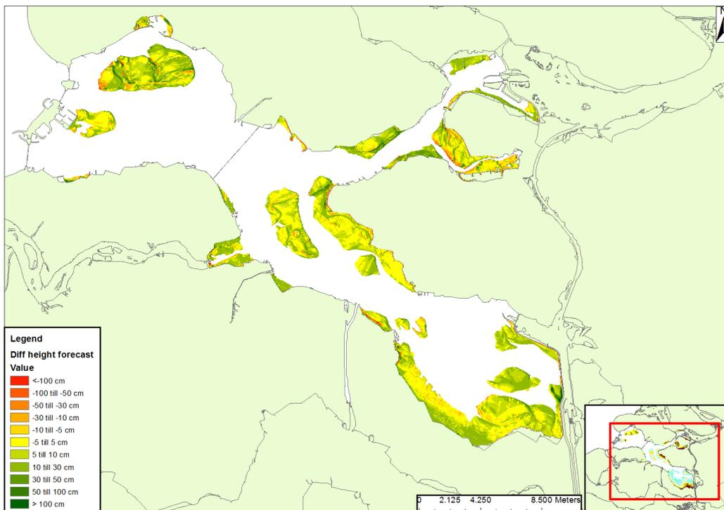
Figure 91. The result of the difference between Vaklodging 2019 and prediction 2020 of Deltares in the whole Eastern Scheldt.
