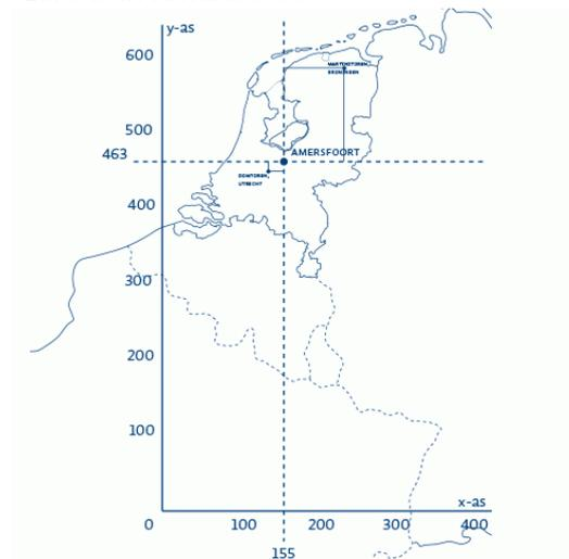
Figure 1. RD Coordinates system overlaid on The Netherlands.
