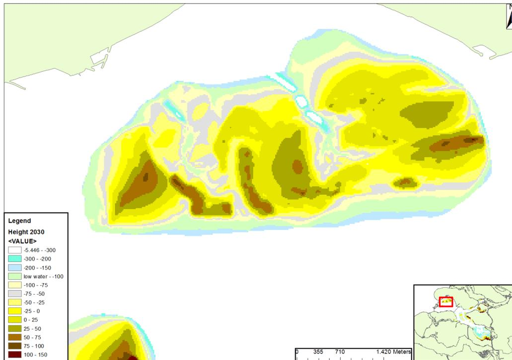
Figure 80. Predicted height of the intertidal flat Roggenplaat in 2030.
