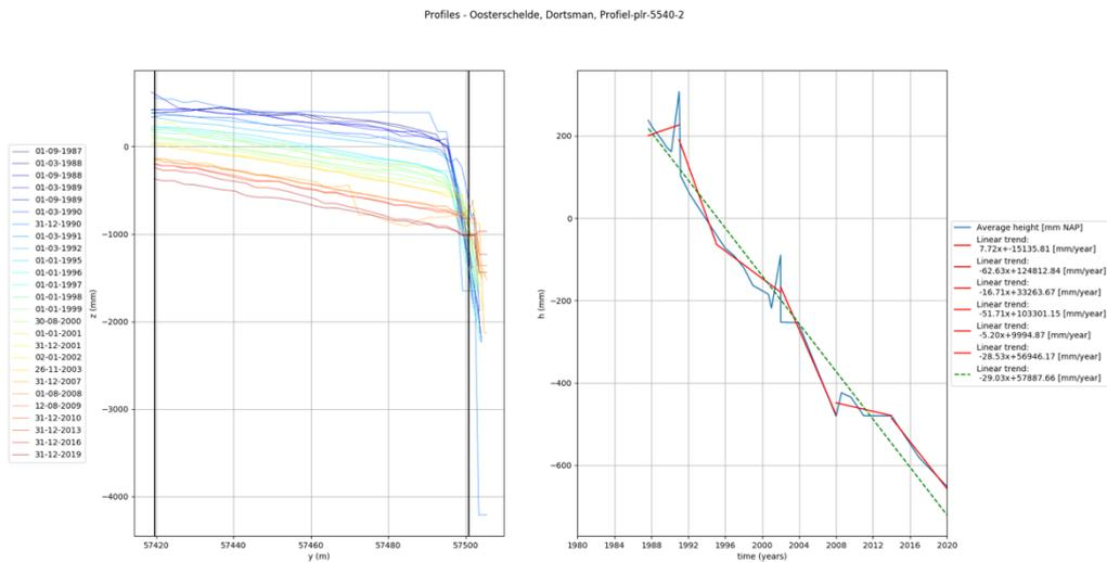
Figure 40. Dortsman Profiel-plr-5540-2, left side the profile and right side the average height per year of the profile.
