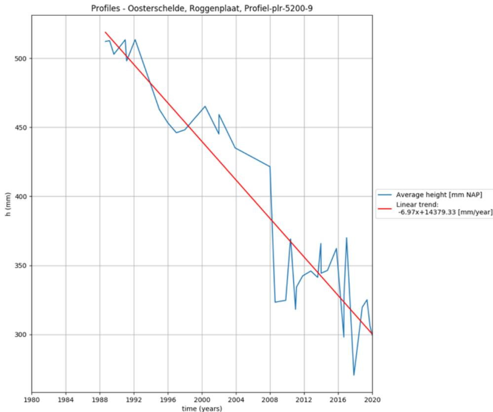
Figure 24. The average height per year together with a regression line. Profiel-plr-5200-9 on the Roggenplaat. The elevation is in millimeter respect to NAP. The regression line shows the average annual erosion of 32 years, in this image -6,9 mm/year.
