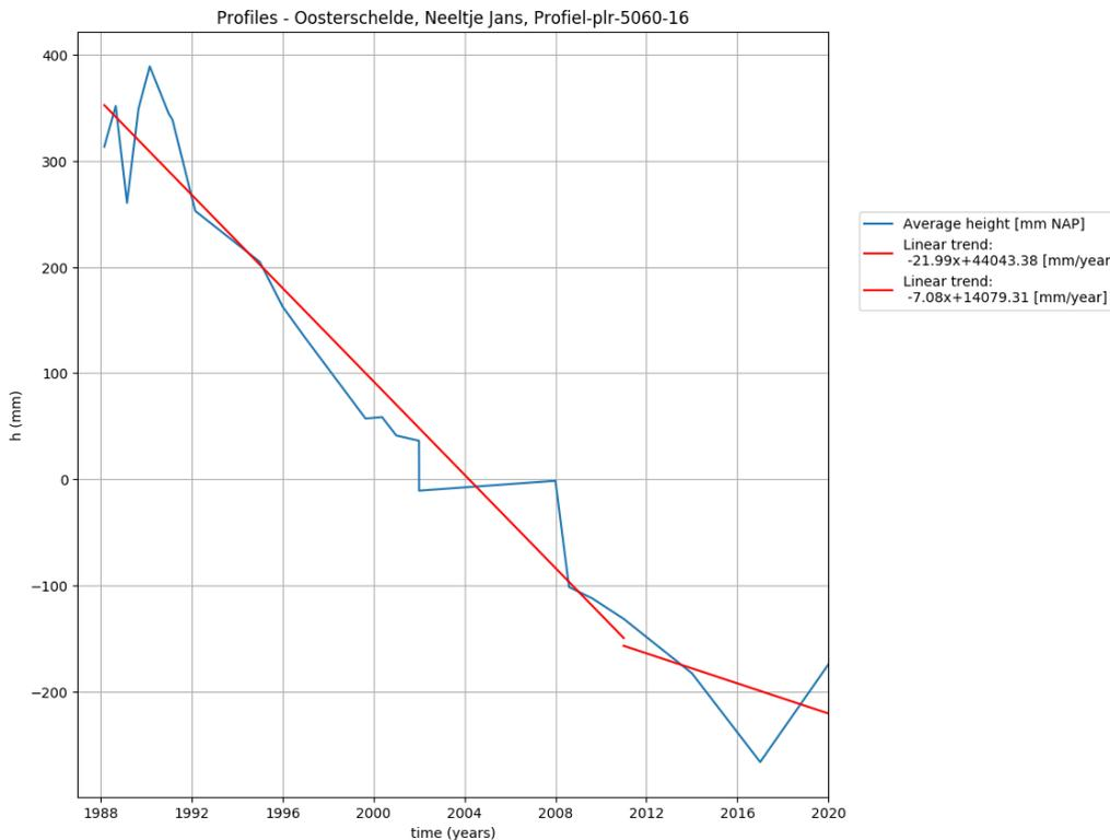
Figure 29. The average height per year together with a regression line. Profiel-plr-5060-16 on Neeltje Jans. The elevation is in millimeter respectively to NAP. The regression line shows the average annual erosion of 32 years, in this image -22 mm/year in 1987 – 2010 and -7 mm/year in 2010 – 2019.
