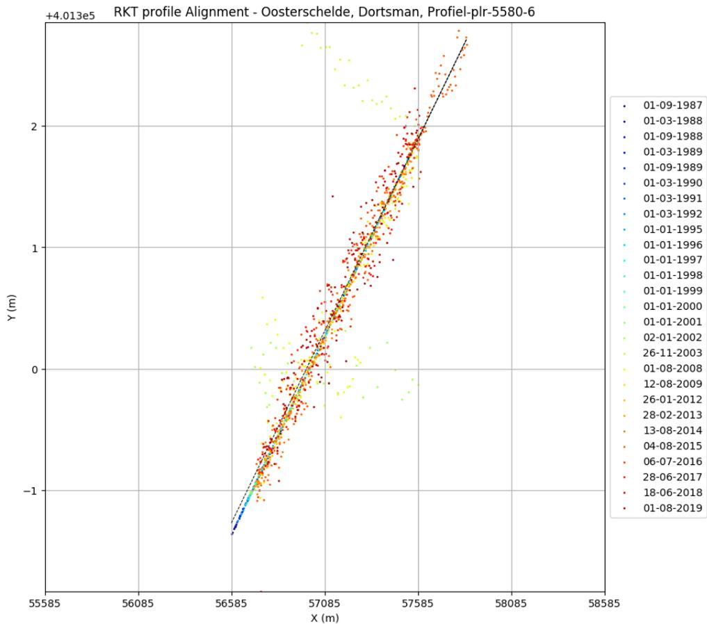
Figure 13. Check if each year of the Dortsman Profiel-plr-5580-6 is straight by plotting the x- and y-coordinates.
