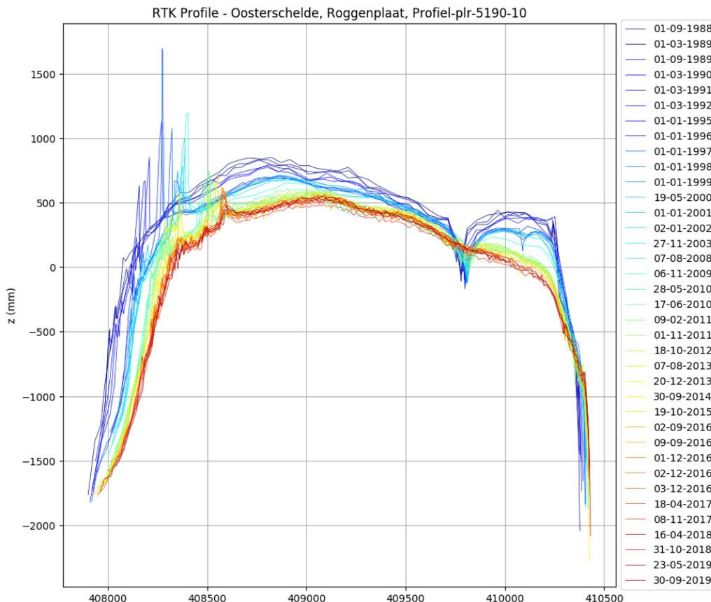
Figure 7. An illustration of the RTK profile. RTK profile Profiel\_plr\_5190\_10 on the intertidal flat Roggenplaat, Figure 8.
