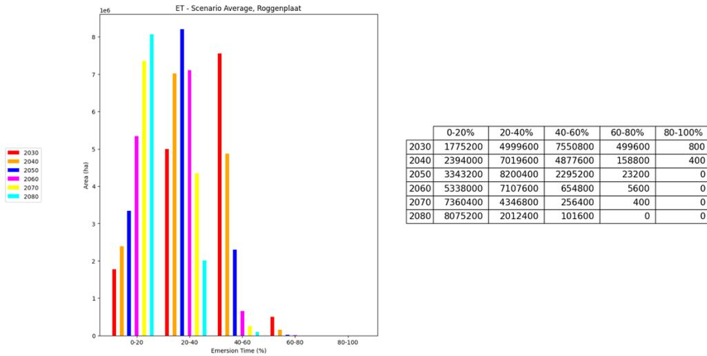
Figure 82. The emersion time graph of the intertidal flat Roggenplaat, Scenario Average.
