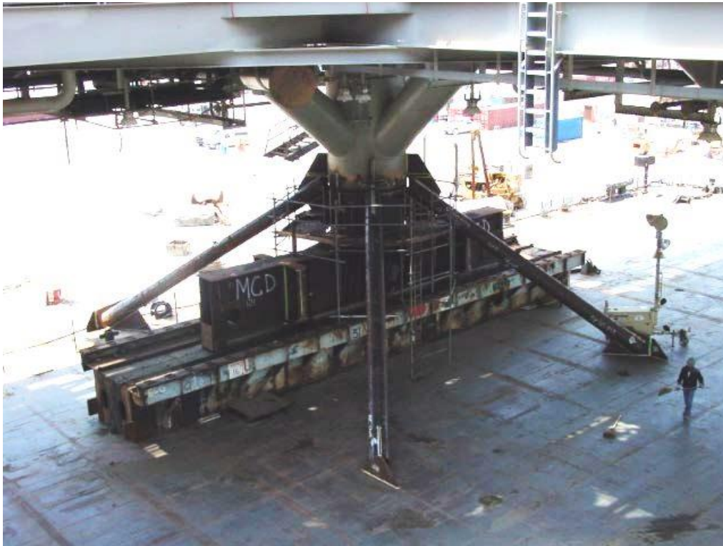
Figure III.H Picture of a Grillage and Seafastening. Grillage and seafastening take up static and dynamic transportation forces.
