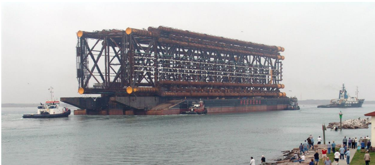
Figure 1.1 The H-851 carrying a jacket [7].
