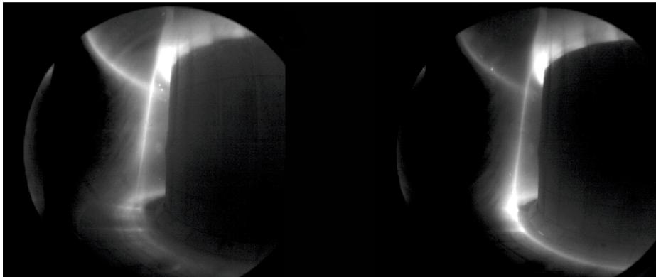
Figure 5.1: Detached plasma in shot #46111, times are 1.52s and 1.57s ( $\Delta t = 0.05s$ ). Left: Plasma is detached. Right: Plasma is re-attached.
