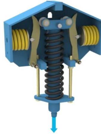
(b) Constant load (triple-spring mechanism)
