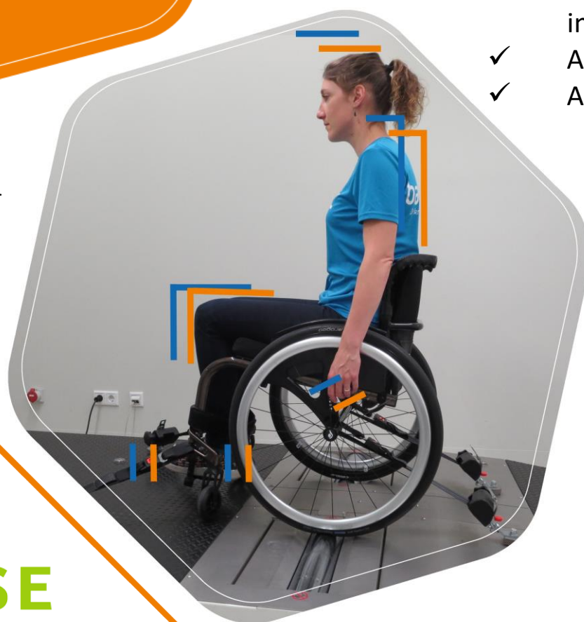
Fig. 2 Person in manual wheelchair after adjustment, on wheelchair ergometer (Lode, Esseda).
