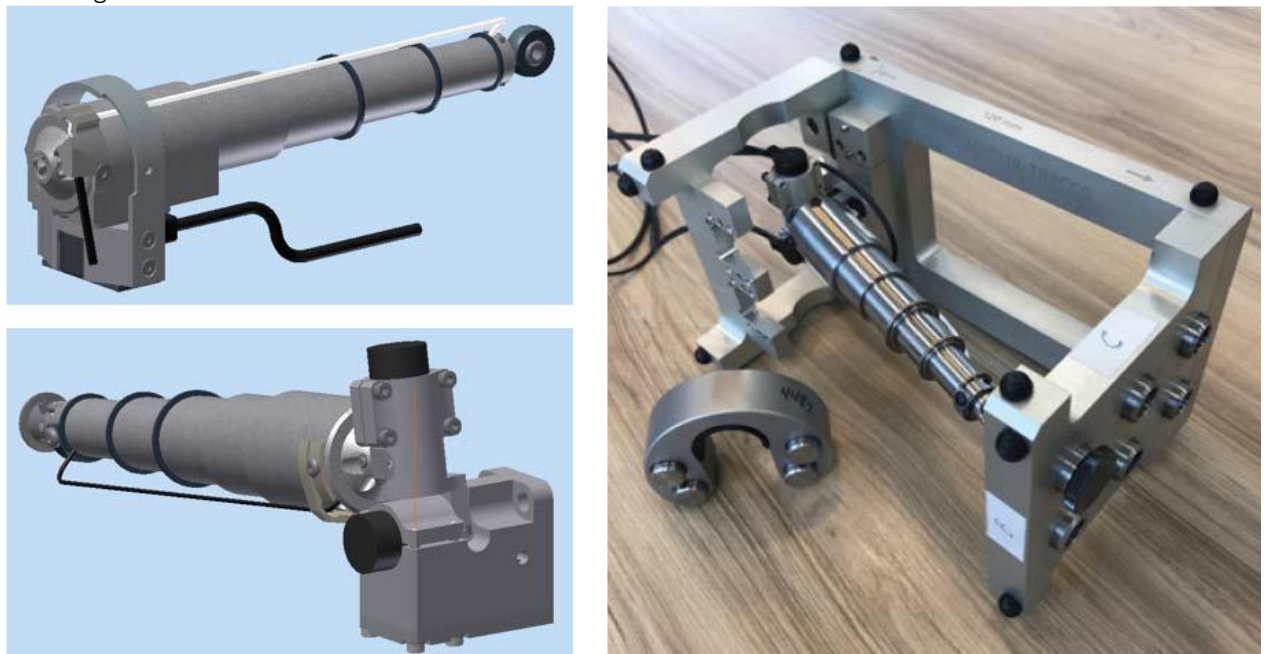
Figure 87: Left top: 2D IRTACC (Infra-Red deflection measurement sensor), Left bottom: 3D IRTACC, Right: Static 3D verification rig suitable for all 3D IRTACCs.
