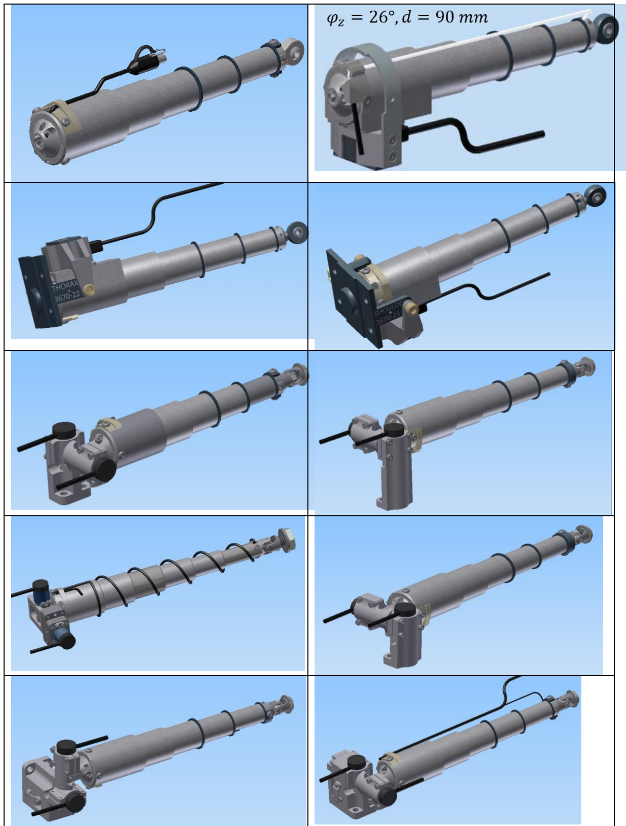
Figure 12: Various IR-TRACC models for 1D, 2D and 3D measurements. For the 3D models, first 3 right sided models are shown, followed by a left-sided model for the upper thorax. Finally the digital (476-series) versions of the lower right and upper right are displayed. The left-sided models are obtained by “inverting” the right-sided models in a similar fashion.
