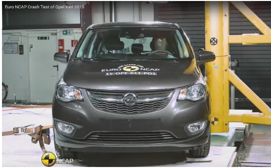
Figure 13: Situation 0. The car has made contact with the pole, but the dummy is not yet undergoing deformation (Euro NCAP, 2015)
