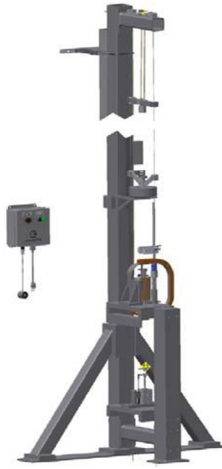
Figure 3: Try-out of a dynamic test set-up. Left: ES2 rib unit with parallel mounted IR-TRACC, Right: Drop tower equipment (total height 6.2 m).
