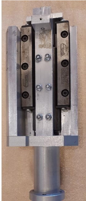
Figure 33: Two M and V guideways in a closed layout, taken out of an EuroSID-2 dummy
