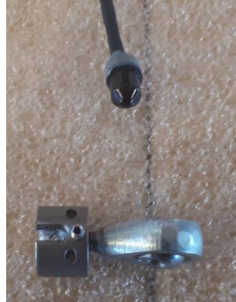
Figure 10: IR LED of an IR-TRACC and its mounting component
