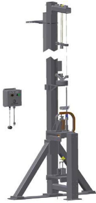
Figure 88: Try-out dynamic test set-up, Left: ES2 rib unit with parallel mounted IRTRACC, Right: Drop tower equipment (total height 6.2 m).
