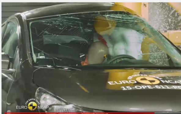
Figure 15: Situation 2. The dummy's direction of movement has been reversed and the compression is now decreasing instead of increasing (Euro NCAP, 2015)
