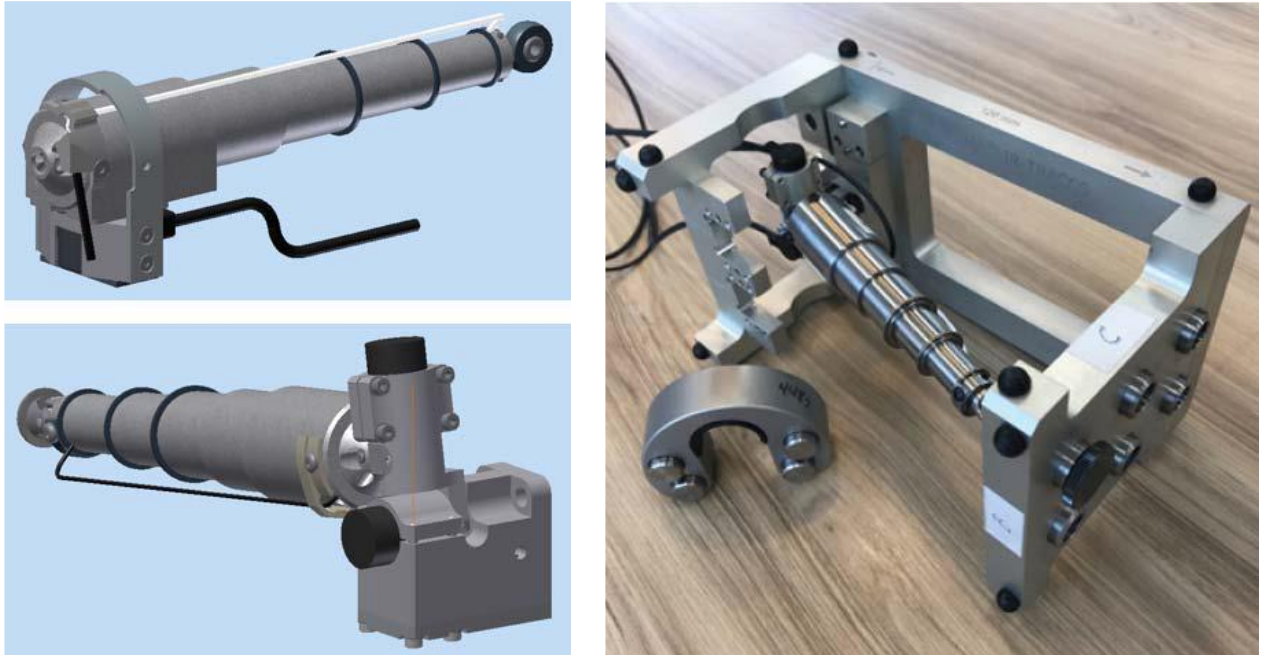
Figure 2: Left top: 2D IR-TRACC (Infra-Red deflection measurement sensor), Left bottom: Digital 3D IR-TRACC, Right: Static 3D verification rig suitable for all 3D IR-TRACCs.
