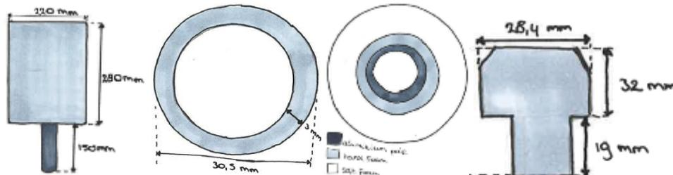
**Figure 25 A:** The dimensions of the perineal post, **B:** The front view of the perineal post, **C:** The aluminium hole tube, the top view of the perineal post with the different layers, **D:** The node of the mounting system of the perineal post
