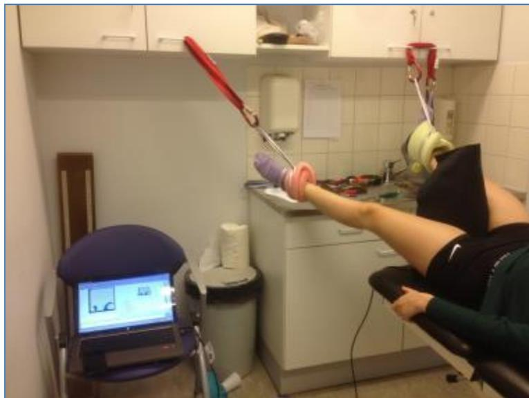
Figure 34 Test setting: redesigned post is placed between the legs, at the right leg traction of 15 kg is applied
