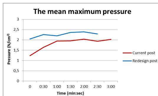
Figure 35 Mean maximum pressure, of the current post (Red) and the redesign (blue)
