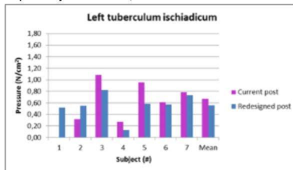
Figure 38 Mean pressure at the left tuberculum ischiadicum
