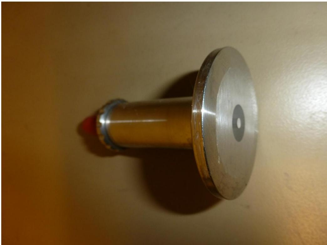
Figure A.1; the probe used for the dielectric measurements.
