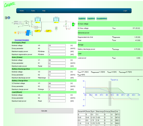
Fig. 5: Designing the droop control characteristics in Caspoc design tool[5]
