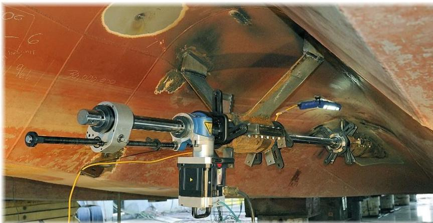
Figure 5-20: Line boring equipment (Redd, 2010)
