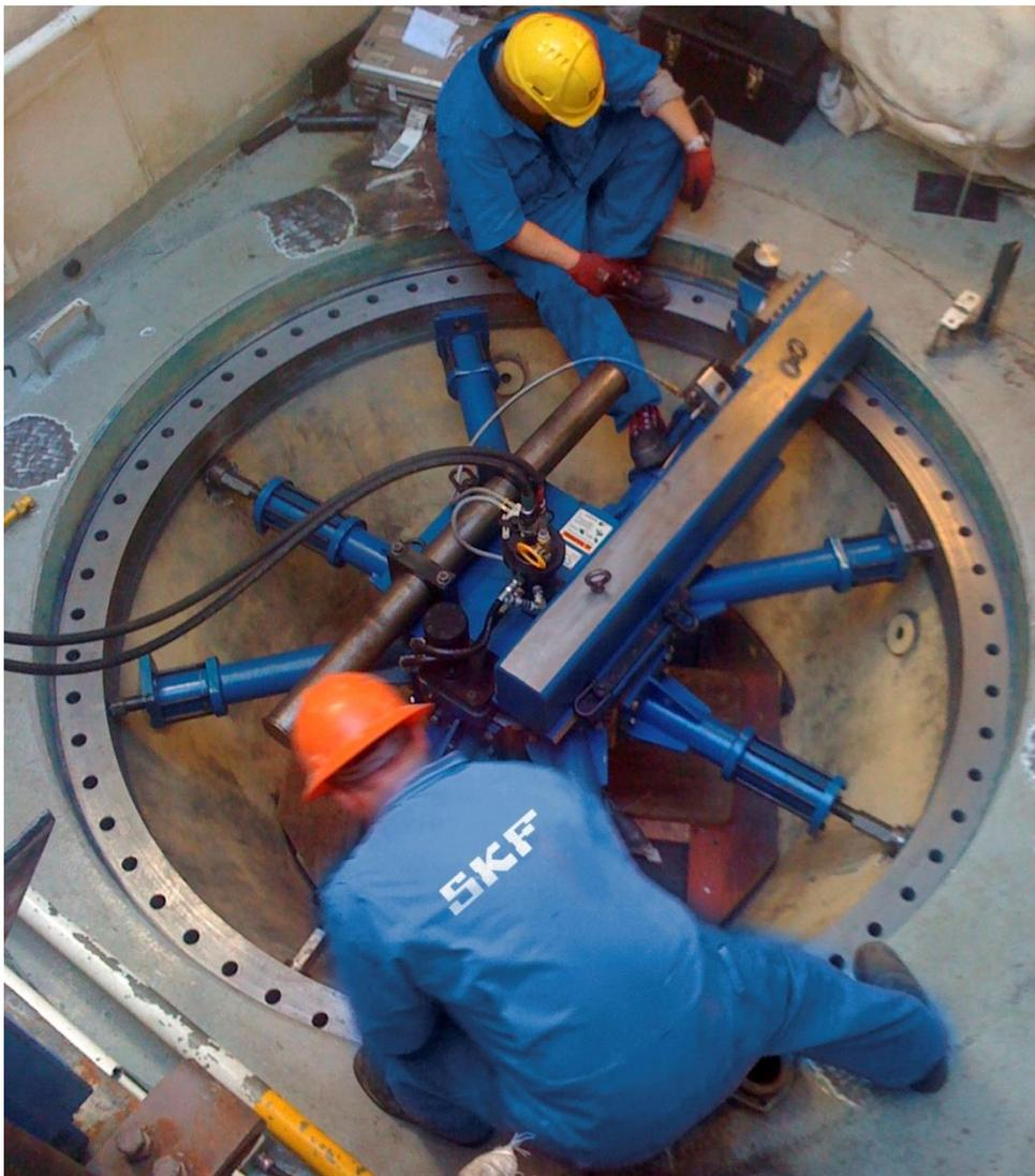
Figure 5-21: Flange facing equipment (SKF, 2013)
