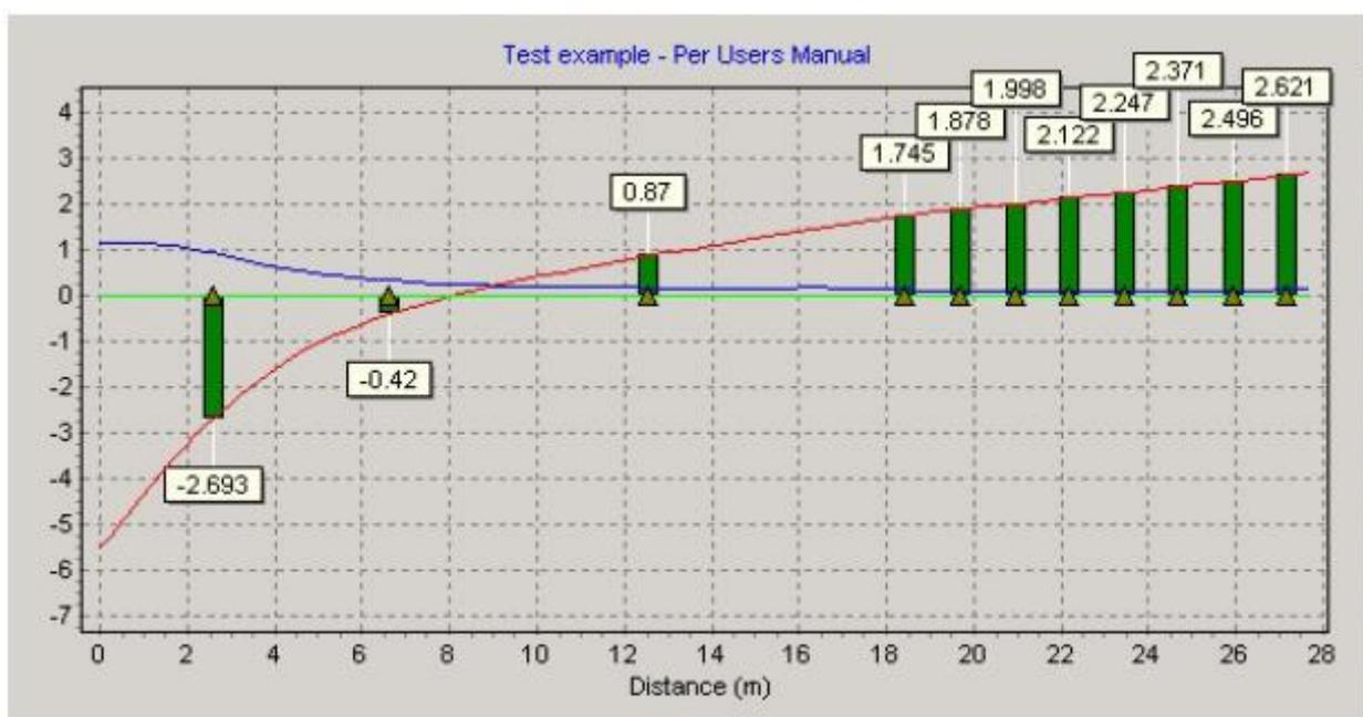
Figure 5-3: Alignment plan (ABS, GUIDANCE NOTES ON PROPULSION SHAFTING ALIGNMENT, 2006)
