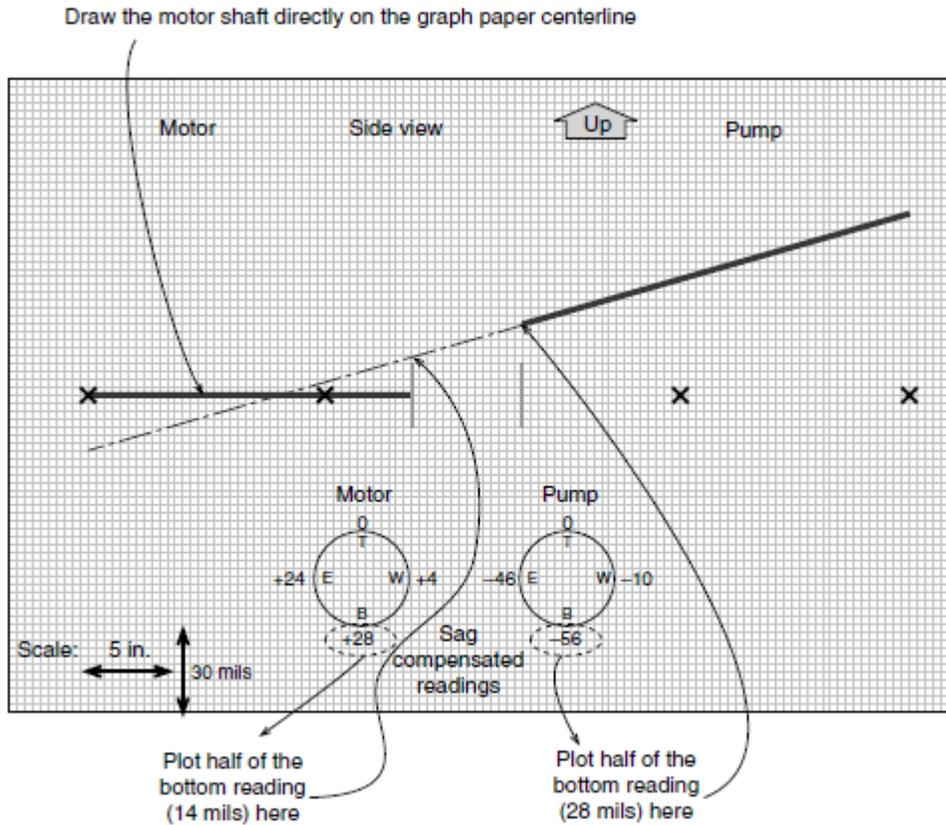
Step 2: Start with the top to bottom or side-to-side dial indicator readings on the other shaft (i.e., the one you did not draw on the graph centerline).
