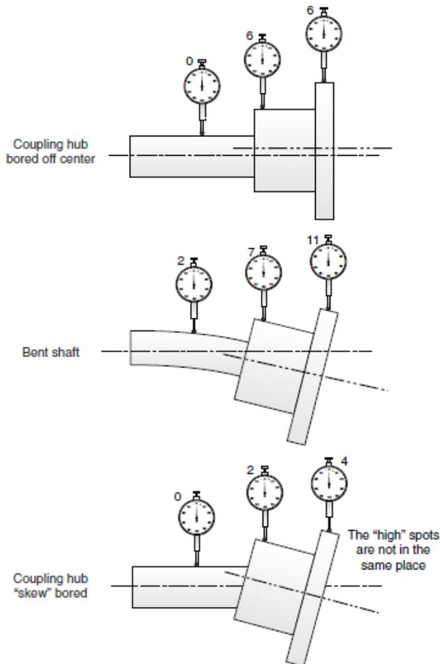
Figure 5-6: Shaft deflection measurement
