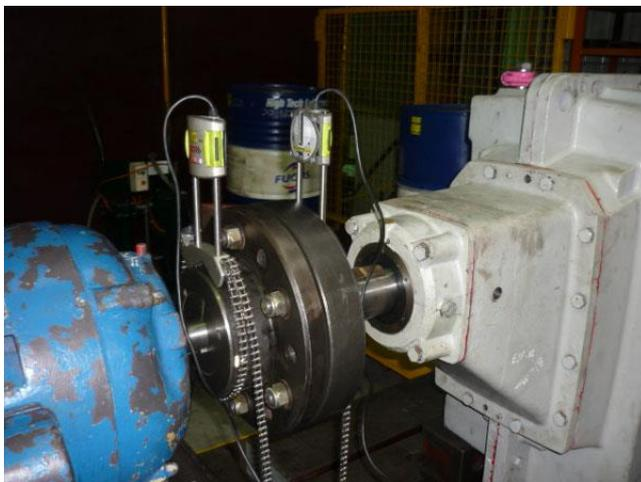
*Figure 5-16: Laser alignment set-up*
