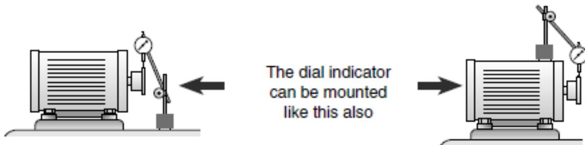
Figure 5-4: Run-out measurement set up
