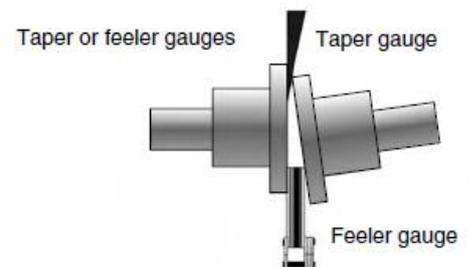
Figure 5-14: Feeler gauge measurement
