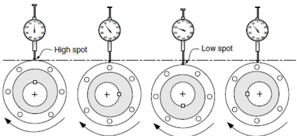
Figure 5-5: Visual representation of run-out
