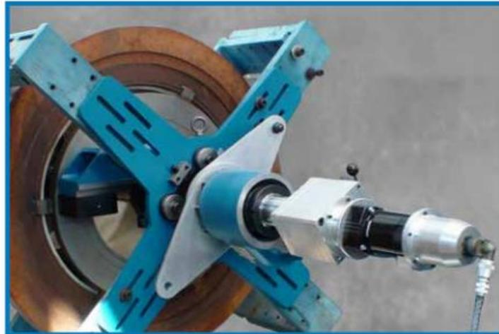
are available. Setup is quick & easy for both boring and facing operations.
