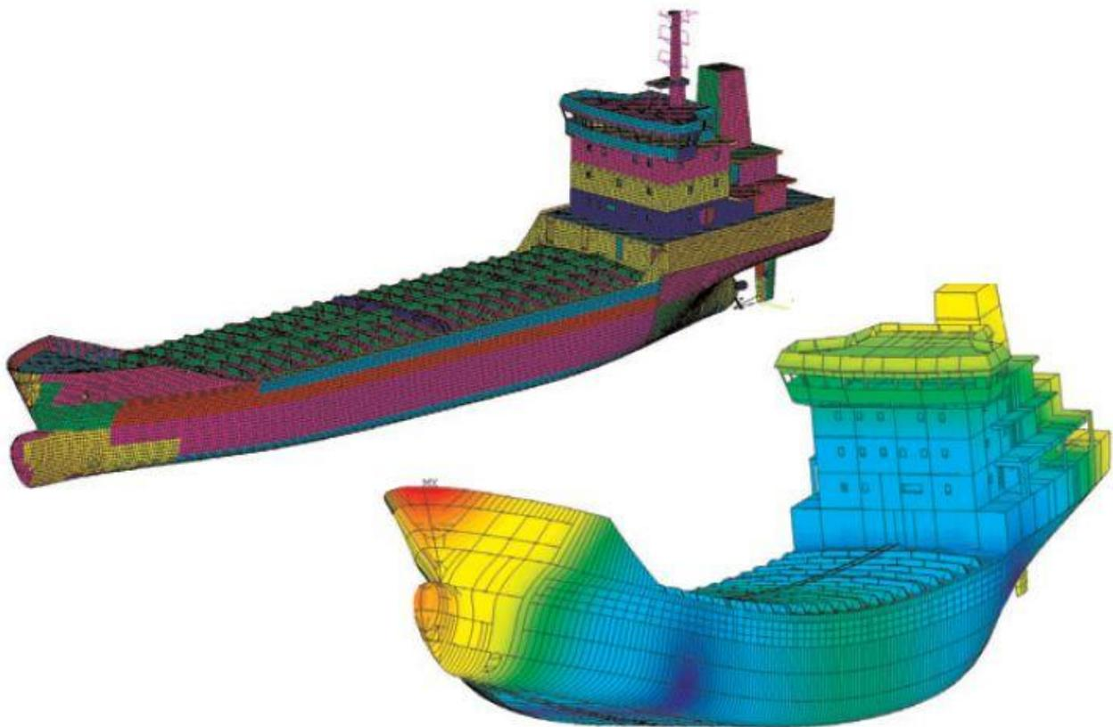
Figure 5-2: Hull deflection (Naval, 2015)
