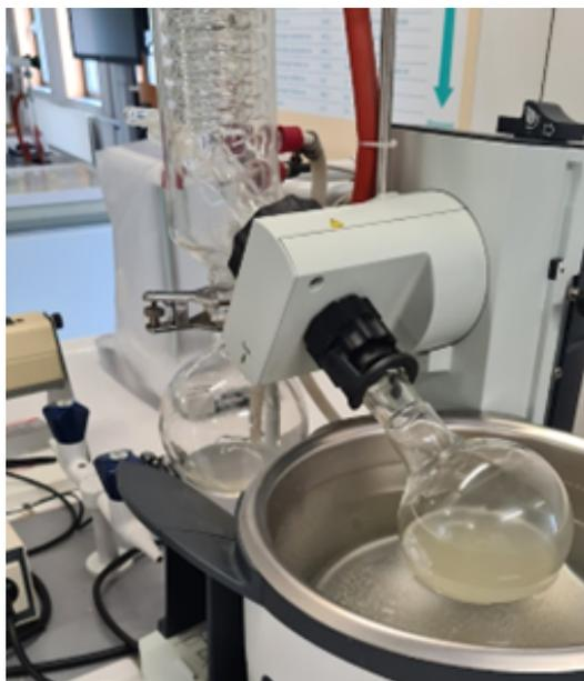
FIGURE 4.4: Rotary Evaporator.
