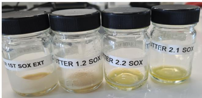
FIGURE 4.5: Mango butter Extraction with Soxhlet with Cotton Wool (1.1, 1.2) and Soxhlet with thimble (2.1, 2.2).
