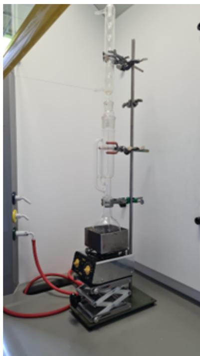
a) Soxhlet apparatus lab set-up.
