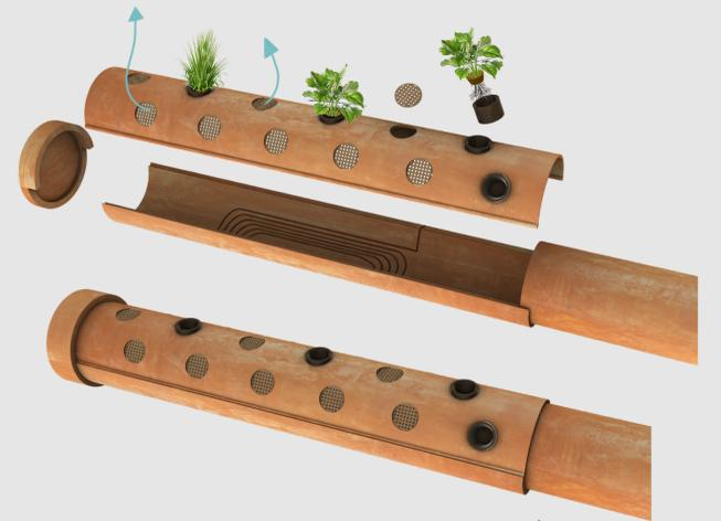
Passive Ventilation vents (windcatchers) lead hot and dry air into terracotta pipes, the end part is equipped with a patterned inner surface for maximum evaporation, the surface is saturated with water from roof what stormwater tank, to evaporating into the rooms cooling the air and humidifying it at once
