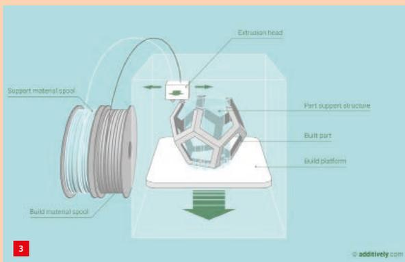
3 Fused deposition modelling (FDM) printing principle.
