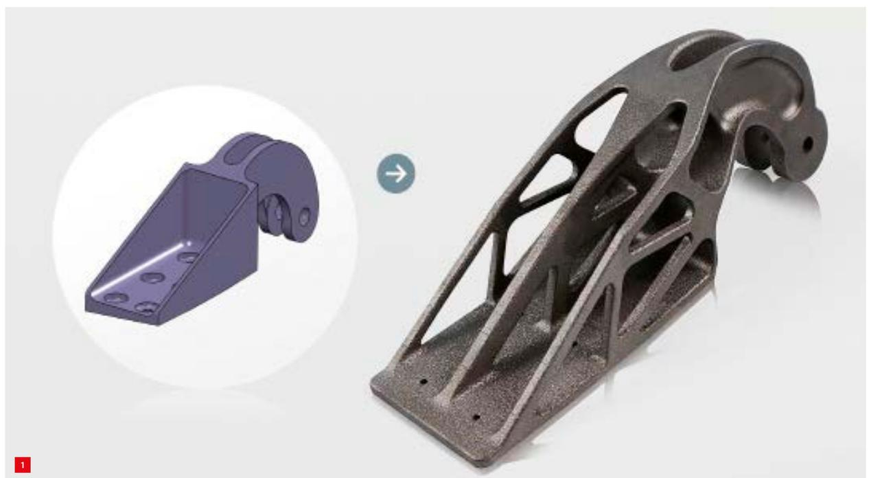
1 Conventional design of a steel-cast bracket (left) and the corresponding topology-optimised design of the titanium AM-made bracket (right), printed on an EOS machine. Source: Airbus Group Innovations
