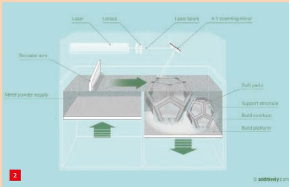
2 Selective laser melting (SLM) printing principle.
