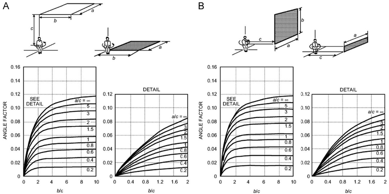
**Fig. 1.** Mean value of angle factor between a seated person and a horizontal or vertical rectangle when the person is rotated around a vertical axis [16]. (a) Horizontal rectangle (on ceiling or floor) and (b) Vertical rectangle (above or below center of person).
