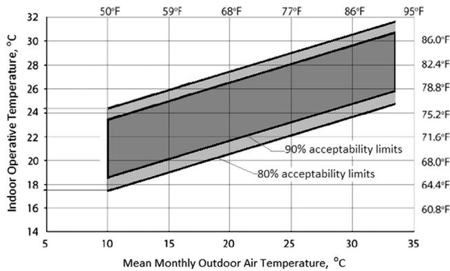
Fig. 5. Acceptable indoor operative temperature as in [21], intended for use in naturally ventilated buildings. The 80% acceptability limits may be used for typical applications and should be used when other information is not available. The 90% acceptability limits may be used when a higher standard of thermal comfort is desired [21].
