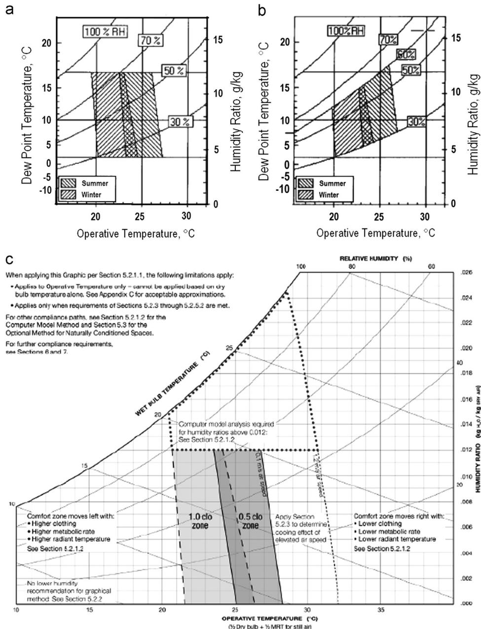
**Fig. 4.** Acceptable ranges of operative temperature and humidity ratio for persons clothed in typical summer and winter clothing, at light, mainly sedentary activity ( $\leq 1.2$  met). (a) ASHRAE Standard 55-1981 [45], (b) ASHRAE Standard 55-1990 [49] and (c) ASHRAE Standard 55-2010 [21].
