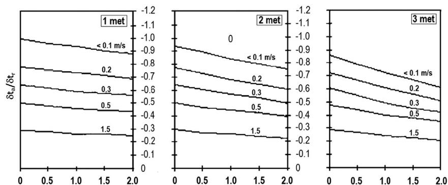
Fig. 3.  $\delta t_a / \delta t_r$  as a function of the thermal resistance of clothing with relative velocity as parameter (RH=50%) [15].
