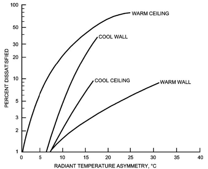
**Fig. 2.** Percentage of occupants expressing discomfort due to radiant temperature asymmetry [27].
