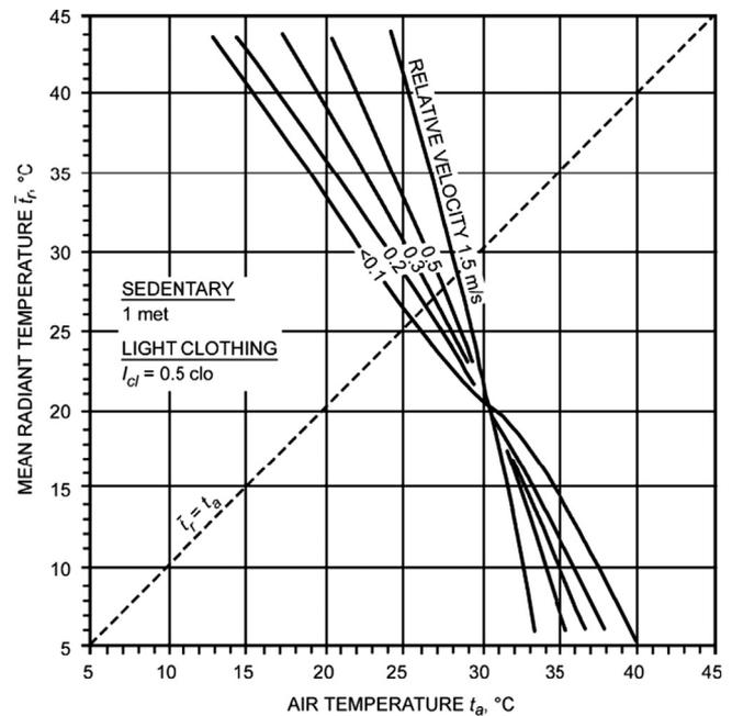
Fig. 6. The effect of air relative velocity on the optimum mean radiant temperatures at various air temperatures and air velocity [15].
