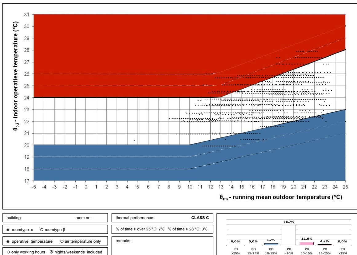
**Figure 6. The ISSO 74: 2014 format for the presentation of simulation or measurement results (colors refer to anticipated average thermal sensation at different rmot - indoor temperature combinations)**
