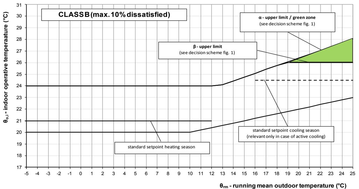
Figure 3. Class B requirements in ISO 74:2014 for the operative temperature indoors in relation to the running mean outdoor temperature
