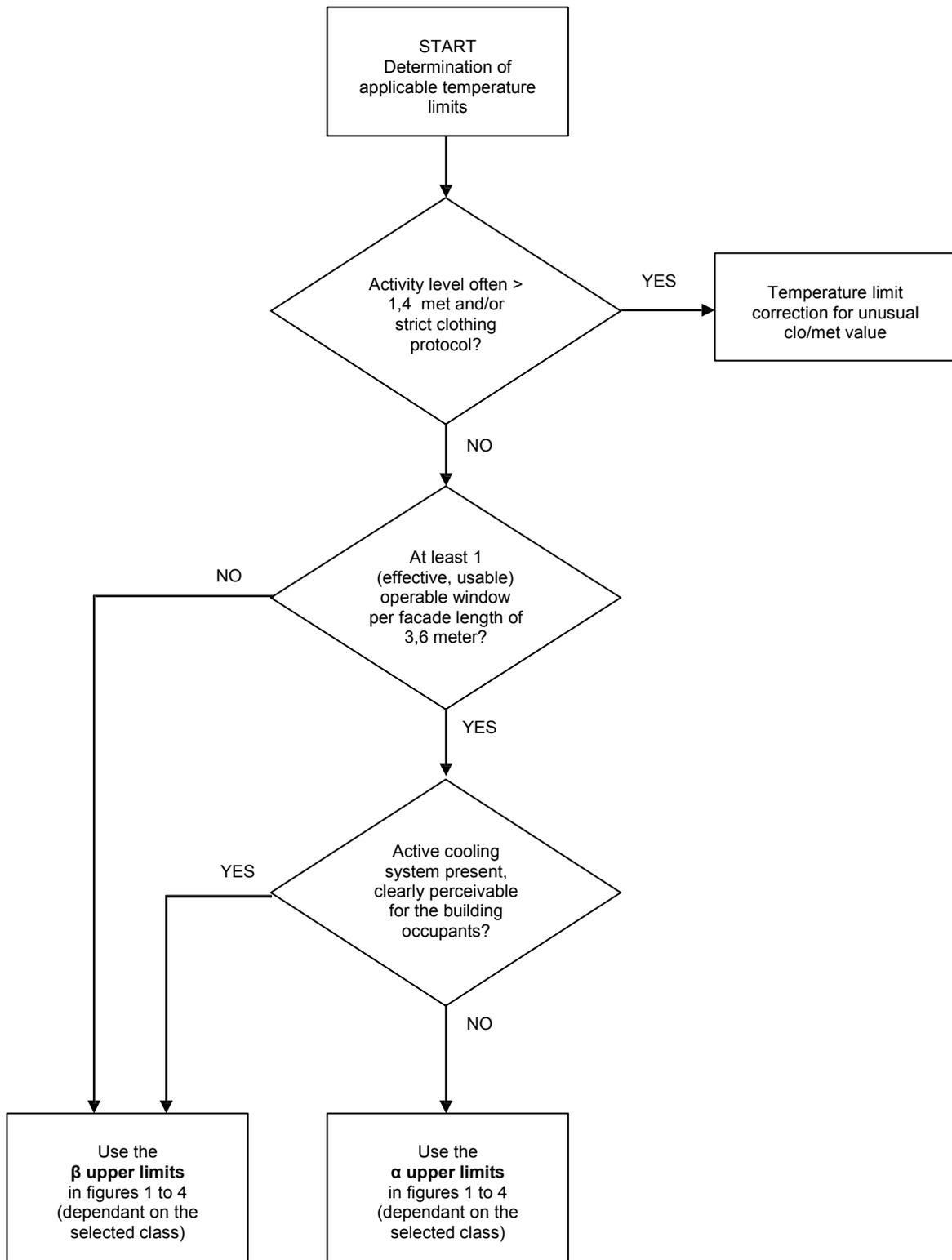
**Figure 1. Decision scheme from ISSO 74:2014 that describes how one can determine whether the  $\alpha$  or the  $\beta$  upper limits should be used**
