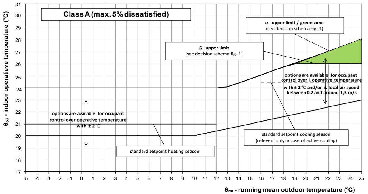
Figure 2. Class A requirements in ISO 74:2014 for the operative temperature indoors in relation to the running mean outdoor temperature
