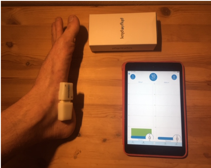
Fig 2. PhysiopluxGo app and EMG biofeedback system.
