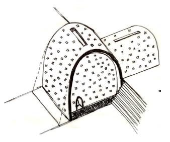
In traditional construction, vaults were built without moulds or support frames. However, using a wooden frame as a temporary guide during construction is common, which can be removed later. Alternatively, a frame made of wooden sticks can be used as a guide to constructing the vault underneath it.
