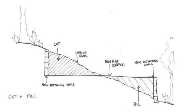
A terracing system is an effective solution for dealing with slopes. It involves creating a series of levelled and stepped platforms on the slop, which helps control erosion, improve stability, and optimize land use. Some critical aspects of implementing a terracing system:
