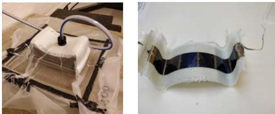
*Figure 20 Solar foil in composite using vacuum bagging*
