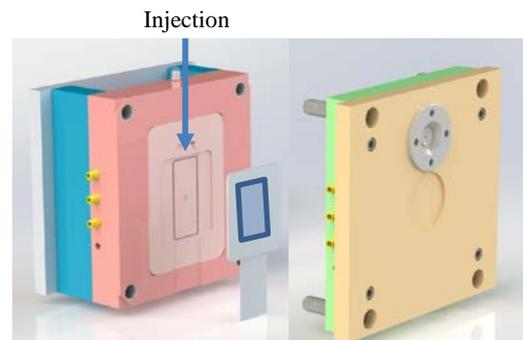
Figure 1 Mould used for testing solar foils
