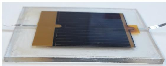
Figure 9 Solar Foil with PC foil 125  $\mu$ m on injected PC
